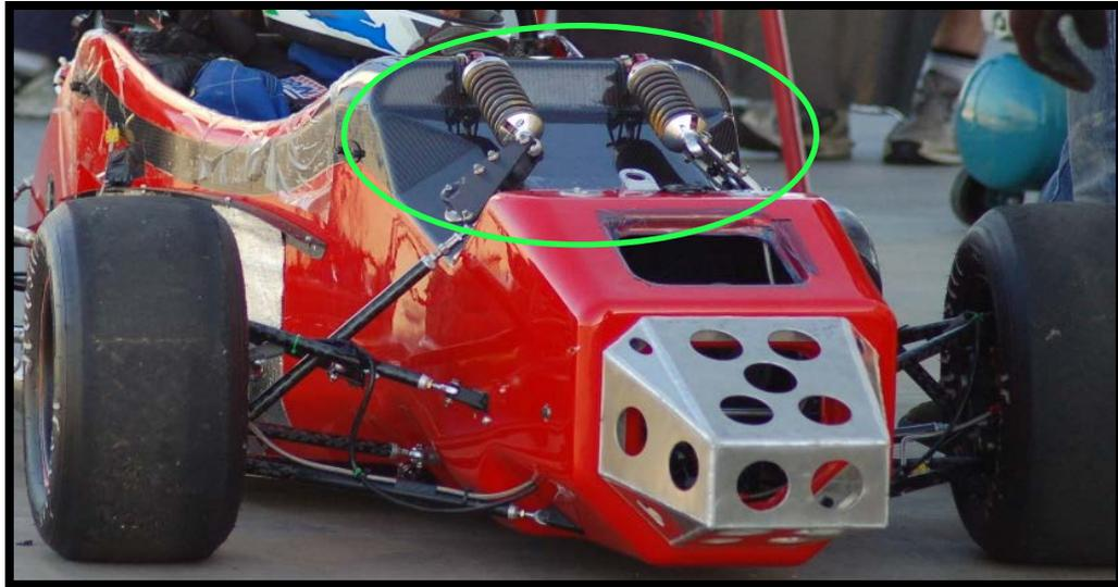
Figure 4.1: Example of the intended layout for the front suspension system – RMIT's 2009 FSAE vehicle. (RMIT Racing, 2010)
