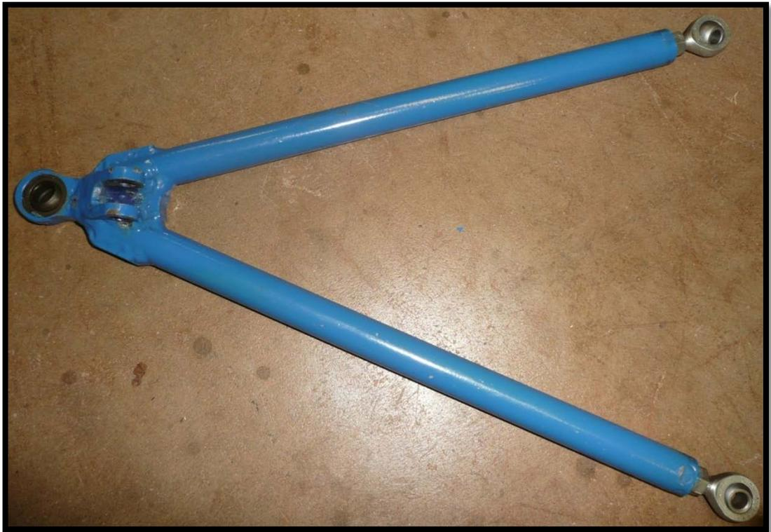
Figure C.6: Front upper wishbone from 2008 vehicle.
