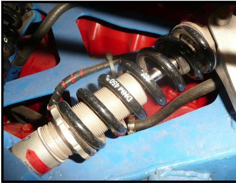
Figure C.3: Rear shock absorber used in 2008 vehicle.
