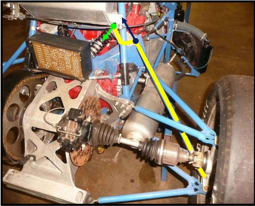
Figure C.1: Poor actuation of the shock absorbers on the 2008 vehicle as seen from the back of the car.
