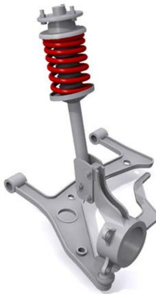
*Figure 2.9: Typical MacPherson strut suspension layout. (Longhurst, 2011)*
