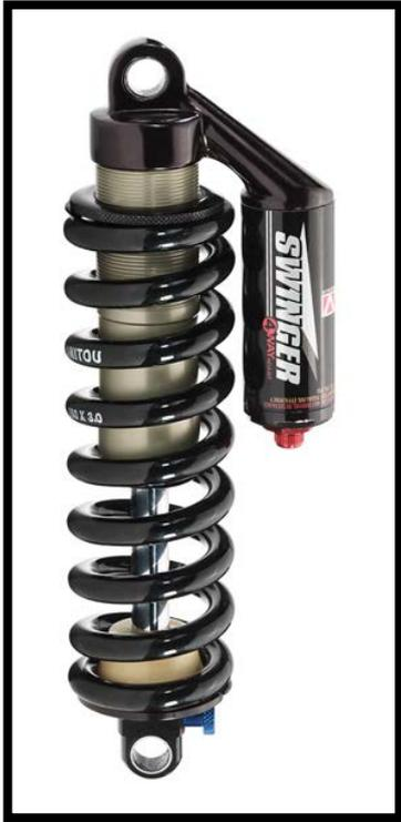
*Figure 6.1: 2005 Manitou Swinger 4-Way Rear Shock*
