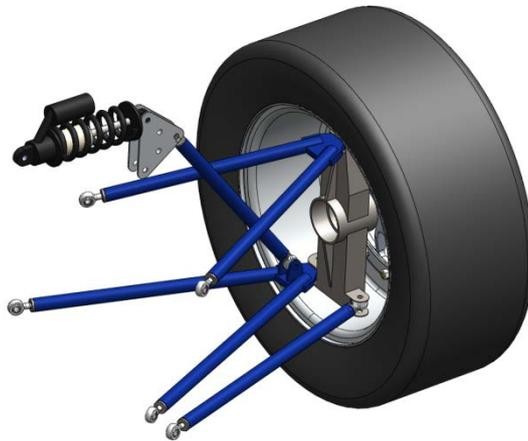
*Figure 8.12: Assembly of rear suspension system SolidWorks.*
