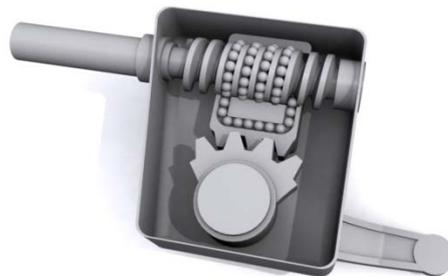
Figure 2.20: Worm and recirculating ball steering box. (Longhurst, 2011)
