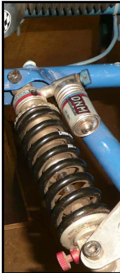
Figure C.4: Front shock absorber used in 2008 vehicle.
