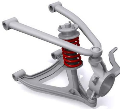
*Figure 2.6: Typical double wishbone suspension layout. (Longhurst, 2011)*
