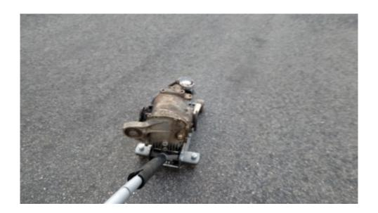
Remove speed sensor and clean it off it will probably have metal shavings on it since its magnetic. 10mm bolts
