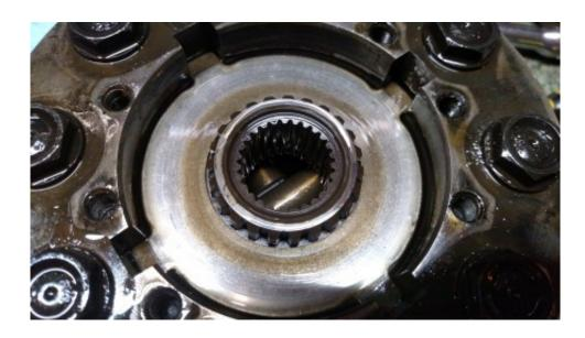
From bottom to top-bellevue washer, dog ear, friction plate. Outer to inner order.
