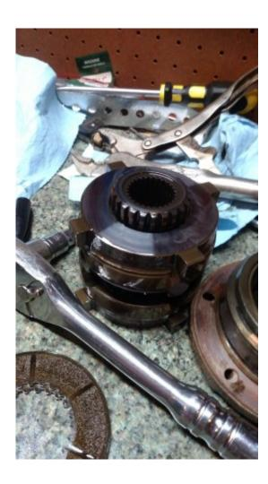
UPGRADE ALERT. This is the spacer that you throw away and replace with a dog ear+friction plate to get that 3rd. This is found right after second large bellevue washer. Place bellevue washer, then the 2 clutch packs ordered from bottom up if adding 3rd clutch pack.
