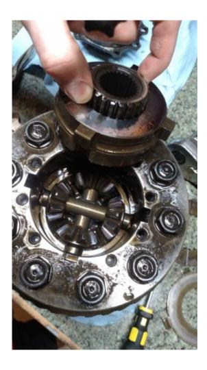
The full spider gear assembly. Below this is another set of (reverse order now) friction plate, dog ear, and bellevue washer. Refer to Diagram up the page to keep track of this.
