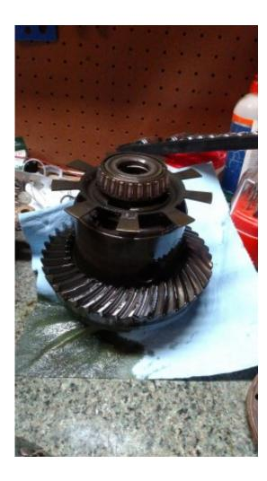
Other side. Other carrier bearing. and the case cover. These bolts are the ones you bought to replace because they do strip. Best way I found to get these off is to hold the whole thing by hand (2 hands hugs it bear style) and have a friend undo the bolts. Totally stripped the first two before I employed someones help to undo them. Have some vice grips ready for stripped bolts.
