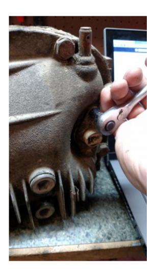
Drain the gear oil 2 17mm oil drain plug Allen key style(smelly) and remove diff cover (8 17mm bolts)
