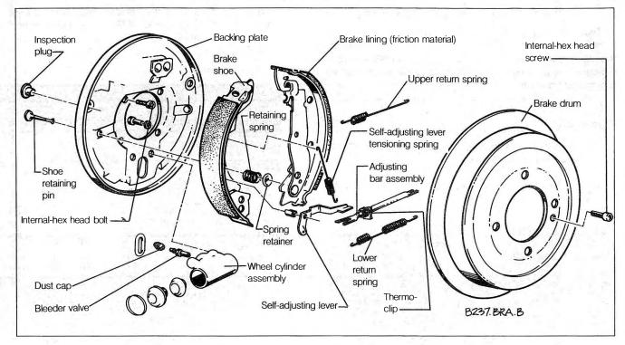
Fig. 6-1. Exploded view of rear drum brake assembly (318i).
