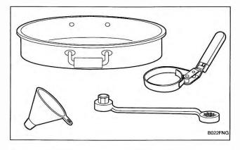
Fig. 4-9. Oil change equipment includes drain plug wrench (17mm), 5 qt. drain pan, oil filter wrench, and funnel.
