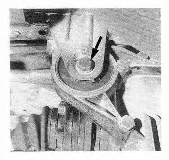
Fig. 5-4. Mounting bolt (arrow) for final drive rubber mounting bushing. Remove nut from other side.
