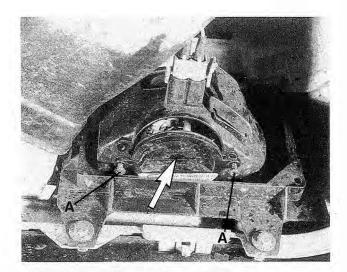
Fig. 6-9. Access cover (arrow) for fog light bulb. Mounting screws are at A.
