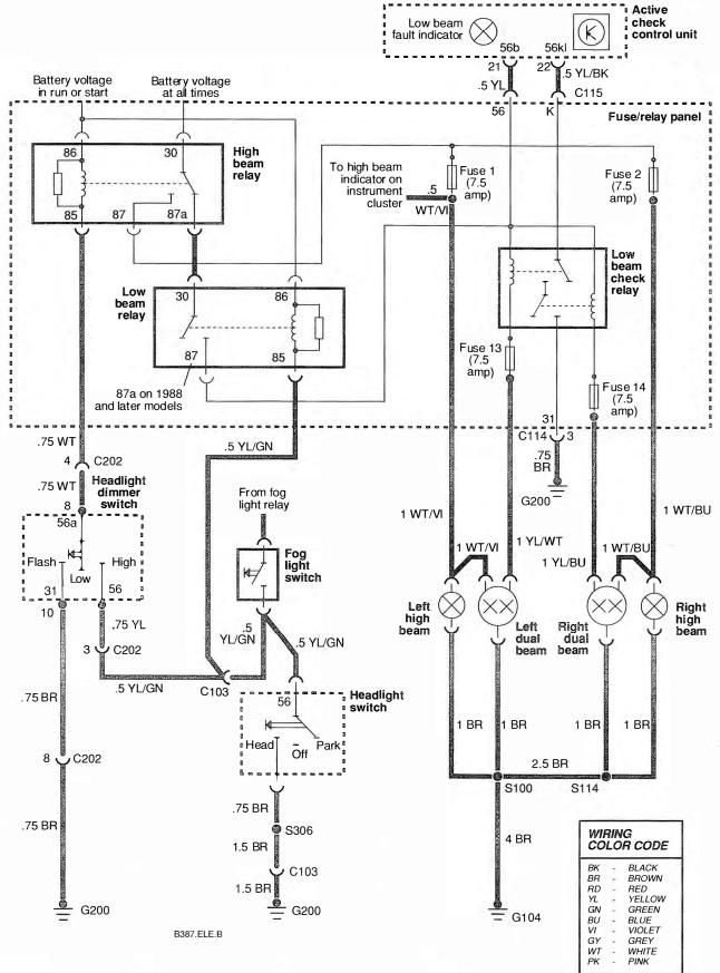
Fig. 10-1. Headlight circuit for models with active check control. Circuit may vary slightly on some models.
