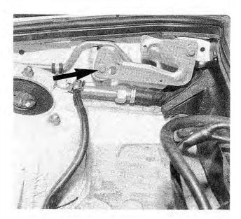
Fig. 6-23. Right-side hood rear-guide bolts (arrows) to be loosened for rear hood height adjustments. Left side is similar.
