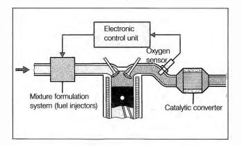
Fig. 7-1. Schematic of oxygen sensor circuit.
