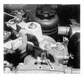
Fig. 6-5. Throttle adjusting screw with tamper-proof cap (A) and throttle lever (B).
