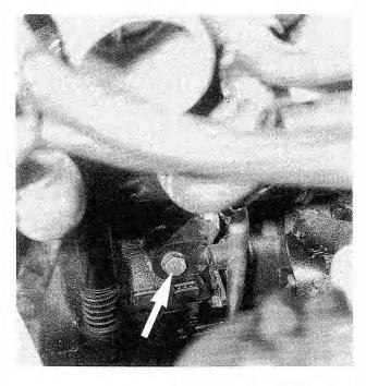
Fig. 6-4. Starter bracket mounting bolt (arrow).
