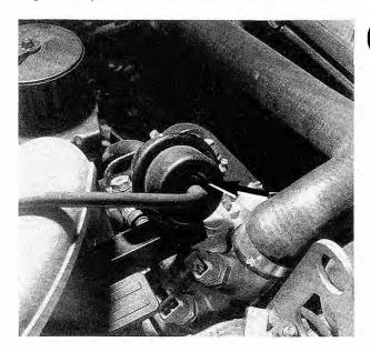
Fig. 4-20. Fuel pressure regulator (arrow). Vacuum hose connection to engine intake manifold adjusts fuel pressure based on engine load to keep difference between fuel pressure and manifold pressure constant.
