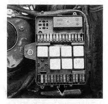
Fig. 5-7. Fuse/relay panel cover removed. Disconnect harness connector (arrow).
