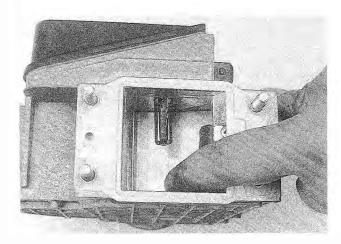
Fig. 6-3. Air flow sensor flap being checked. Move flap through entire range of travel to check for binding and smooth operation.
