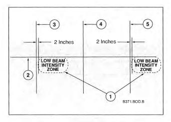
Fig. 6-3. Headlight aiming target on vertical wall. Low beam light intensity areas are at 1. Line 2 is at height of headlight centers. Line 4 is car centerline. Lines 3 and 5 are distance from centerline to centers of headlights.
