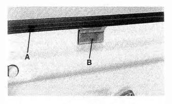
Fig. 5-17. Inner window channel seal (A) and interior trim panel retaining clip (B).
