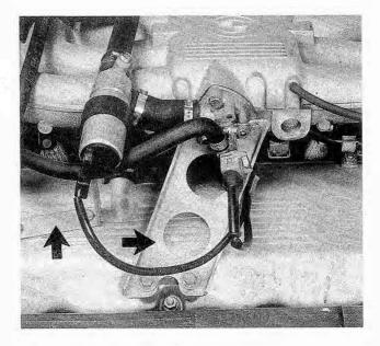
Fig. 4-2. Intake manifold and idle air stabilizer valve support brackets (arrows) on 325e engine. Brackets on other engines are similar.
