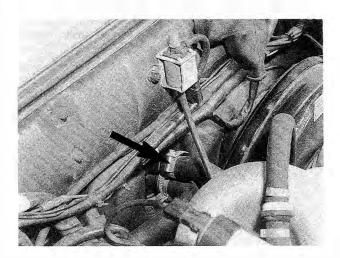
Fig. 4-20. Coolant hoses leading to heater core (arrow).
