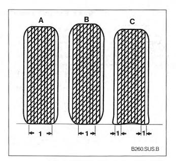
Fig. 3-2. Effect of tire inflation pressure on wear pattern. Condition A is normal. Condition B is overinflation which causes increased wear in center of tire tread. Condition C is underinflation which causes increased wear on outer edges of tire tread. Dimension 1 is tire contact area.
