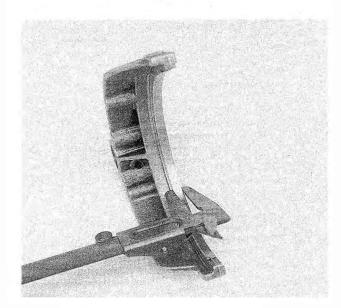
Fig. 7-48. Shift fork being checked for wear.
