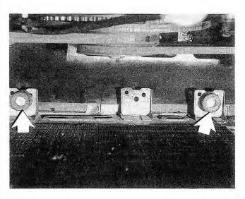
Fig. 4-31. Typical rubber lower radiator mountings (arrows).
