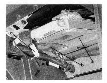
Fig. 5-15. Motronic control unit (a), idle speed control unit (b), and 3-point harness connector (c) as viewed from above glove compartment.
