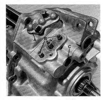
Fig. 7-10. Shiftrod detent ballend plate (A), springs (B), and end plug (C). Detent balls are under springs.
