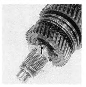
Fig. 7-33. Thrust washer and ball between 2nd and 3rd gear. Ball in shaft (arrow) prevents washer from rotating.
