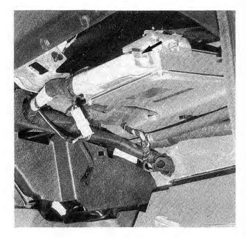
Fig. 5-18. L-Jetronic control unit connector and retaining screw (arrow).
