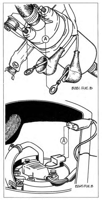
Fig. 4-14. Schematic view of ammeter connected between fuel pump connector and fuel pump on externally mounted fuel pump (top) and in-tank mounted fuel pump (bottom).
