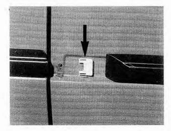
Fig. 6-15. Beveled clip (arrow) for body side moldings. Slide molding onto clip first, then press onto other clips.
