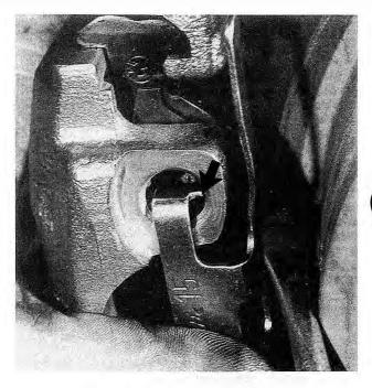
Fig. 7-4. Anti-rattle spring being removed. Unhook spring from caliper housing at arrow.
