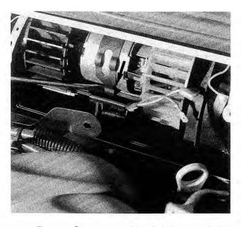
Fig. 4-33. Blower motor retaining clip being removed using screwdriver (arrow).
