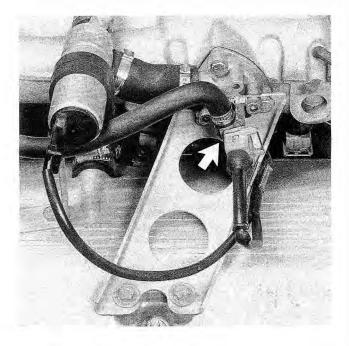
Fig. 1-1. Cold-start valve or "fifth injector" (arrow) on intake manifold distinguishes earlier Motronic system (with valve) from later Motronic 1.1 system (without valve).
