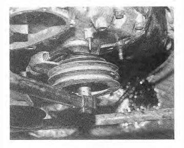
Fig. 4-16. Vibration damper secured with wrench while mounting nut is loosened.
