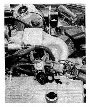
Fig. 3-2. Oil dipstick seal and oil filler cap seal (arrows) should be inspected and replaced if found to be faulty. 4-cylinder engine shown, 6-cylinder engine is similar.
