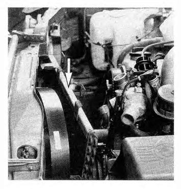
Fig. 4-26. Air conditioning condenser correctly positioned for removal of auxiliary cooling fan.
