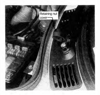
Fig. 8-5. Wiper arm retaining nut (arrow).
