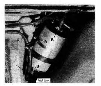
Fig. 5-4. Main fuel filter beneath car near left rear wheel. Direction of flow is indicated by arrow on filter housing. Loosen clamping bracket at filter center (A) and two hose clamps (B).
