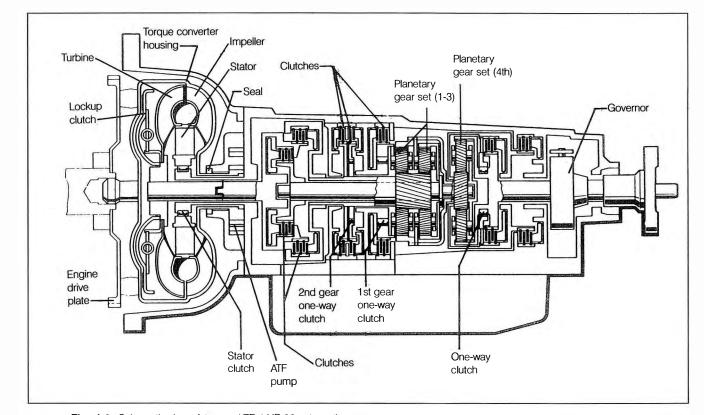
Fig. 1-2. Schematic view of 4-speed ZF 4 HP 22 automatic transmission. 3-speed ZF 3 HP 22 automatic transmission is similar.
