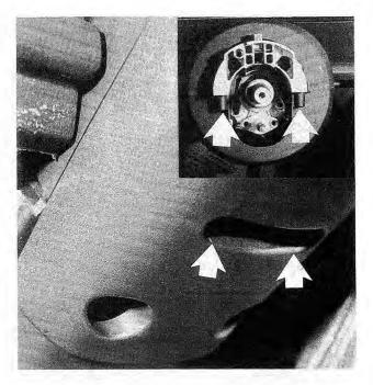
Fig. 7-7. Remove four screws (arrows) to release lower steering column trim panel for access to switches on steering column.
