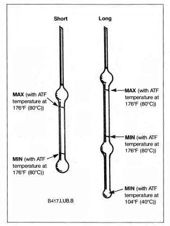
Fig. 7-7. Two versions of automatic transmission dipsticks installed on cars covered by this manual.
