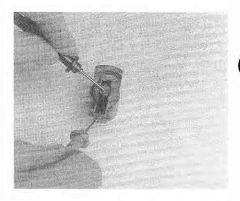
Fig. 3-7. Resistance of rotor being checked with ohmmeter. Rotor from 4-cylinder engine shown.
