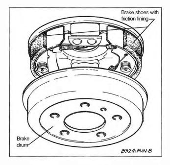
Fig. 1-8. Drum brake assembly with brake drum removed to show brake shoes.
