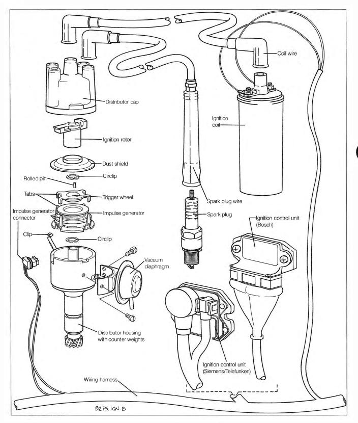
Fig. 4-1. Transistorized coil ignition with impulse generator installed on 4-cylinder engines.
