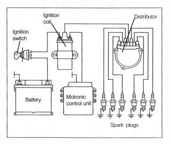
Fig. 1-2. Schematic view of ignition system on Motronic engine-management system for 6-cylinder engines.
