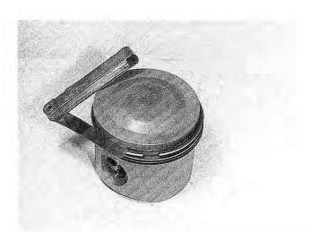
Fig. 6-8. Measuring piston ring side clearance with feeler gauge.
