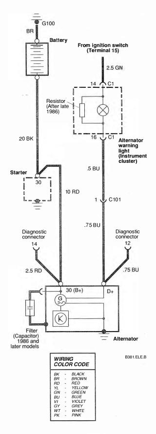
A reading below 13.5 volts means that the battery is not being adequately charged. This may be due to either a faulty regulator or alternator. To determine which, keep the car running at about 1500 rpm and turn on all electrical accessories, then check voltage across the battery. A reading that is the same as the first most likely indicates a faulty regulator. A reading that is lower most likely indicates a faulty alternator.
