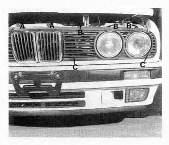
Fig. 6-17. Front center grille retaining clips (A), and side grille retaining clips (B) and screws (C).
