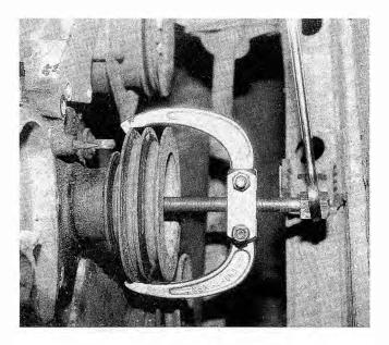
Fig. 4-17. Vibration damper being removed from crankshaft with puller and wrench.
