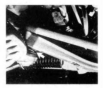
Fig. 5-11. Outer control-arm ball joint. Inner ball joint is similar. Excessive play between control arm and subframe or suspension strut (arrow) is cause for replacement.
