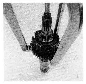
Fig. 7-34. 5th/reverse gear guide sleeve assembly being removed from output shaft.
