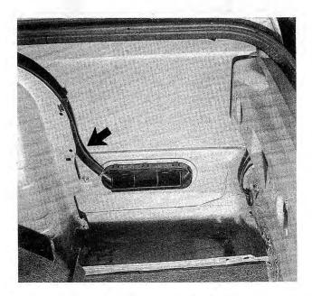
Fig. 7-1. Sunroof rear drain hose (arrow) behind trunk side trim.
