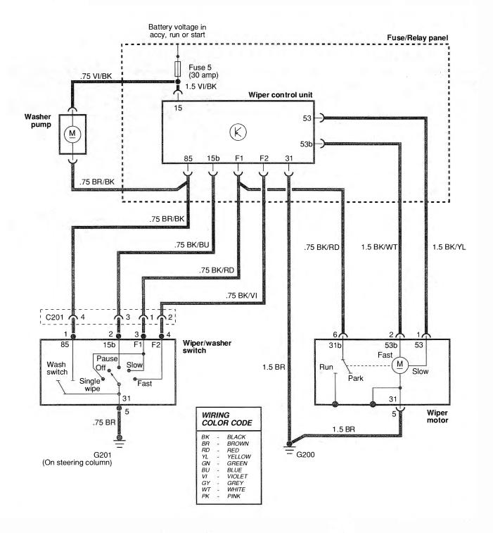
Fig. 8-2. Windshield wiper and washer system circuit.
