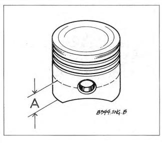
Fig. 6-5. Distance from bottom of piston skirt to measuring point (A) for determining piston diameter. Distance varies between engines depending on piston manufacturer.
