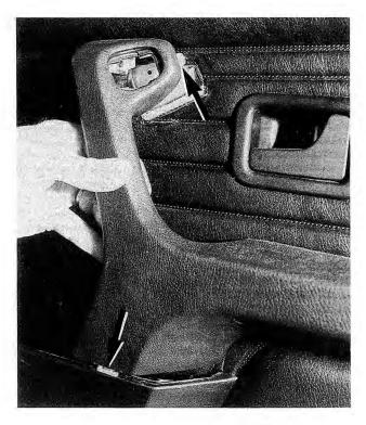
Fig. 5-10. Front armrest being disengaged from door trim panel. Note locking tabs (arrows). Pull armrest forward and out.
