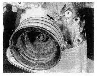
Fig. 4-47. Top Dead Center (TDC) mark on vibration damper aligned with boss on lower timing chain cover (arrow).
