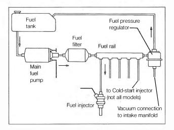
Fig. 4-1. Schematic view of L-Jetronic fuel supply system.
