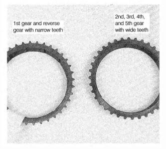
Fig. 7-38. Two types of synchronizer rings.
