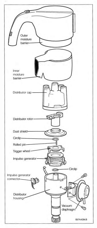
Fig. 4-6. Exploded view of distributor assembly installed on cars with 4-cylinder engines.
