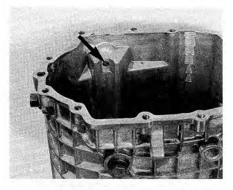
Fig. 7-22. Area of front transmission case (arrow) requiring gasket sealer.
