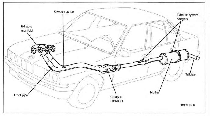
Fig. 1-5. Typical exhaust system.
