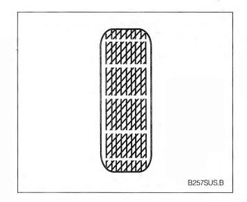
Fig. 3-1. Tire tread wear-indicator bands showing on worn tire indicate that replacement is necessary.
