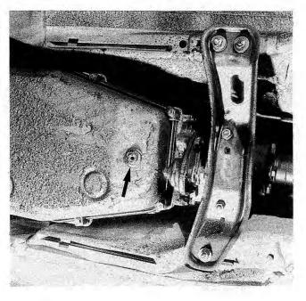
Fig. 7-8. Automatic transmission fluid drain bolt (arrow).
