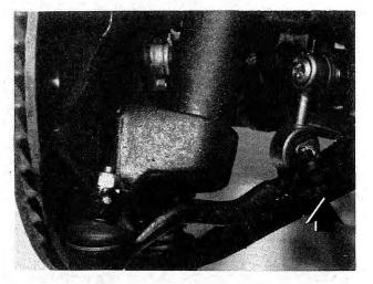
Fig. 4-5. Front wheel toe is adjusted by shortening or lengthening tie rod. Loosen tie rod clamping bolt (arrow) and turn tie rod as shown. (Shown with steering turned off-center for clarity).
