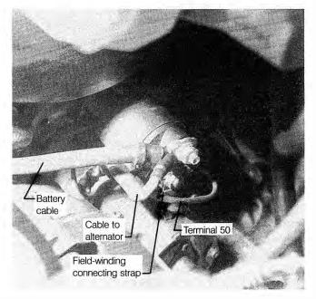
Fig. 6-3. Starter wiring at solenoid. Remove wires shown at arrows. 1988 through 1990 models have an additional wire (not shown).
