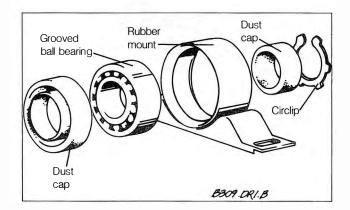
Fig. 4-10. Exploded view of center bearing components.
