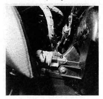
Fig. 4-27. Temperature flap control cable showing adjusting knob (A) and cable retaining clip (B).
