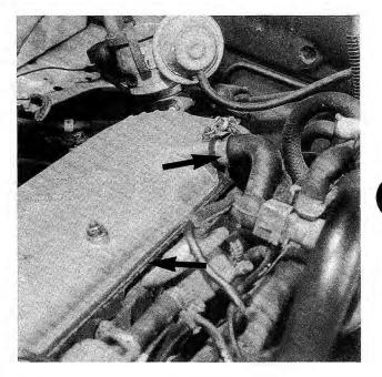
Fig. 3-4. A leaking cylinder head cover gasket or cracked or brittle PCV hose (arrows) should be replaced. Also check the small vacuum hose to distributor on models with 4-cylinder engine.
