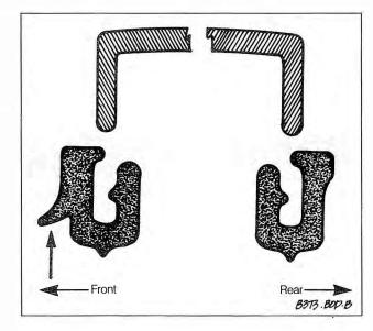
Fig. 7-2. Cross-section of sunroof seal showing correct installation of seal to sunroof panel. Note sealing lip (arrow) on forward portion.
