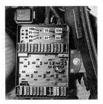
Fig. 8-1. Wiper control unit location (control unit removed) and terminal identification on fuse/relay panel.
