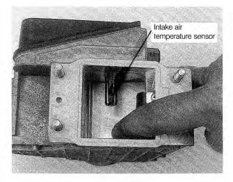
Fig. 5-3. Air flow sensor flap being checked. Move flap through entire range of travel to check for binding and smooth operation.
