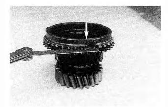
Fig. 7-47. Synchronizer ring being checked for wear using feeler gauge. Measure in the area of the tabs (arrow).
