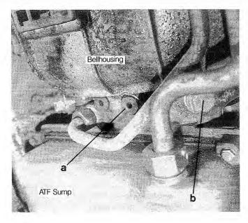
Fig. 3-1. Main pressure tap on transmission case for 3 HP 22 transmissions (a), and 4 HP 22 transmissions (b). Tap is located below torque converter bellhousing.
