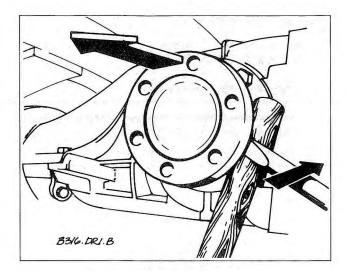
Fig. 5-6. Prying off drive flange. Use extreme care to avoid damaging final drive. For leverage, use wooden dowels as shown.
