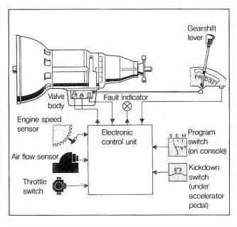
Fig. 1-3. Schematic of 4 HP 22 EH automatic transmission showing electronic control system.
