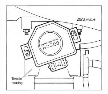
Fig. 5-16. Throttle switch showing terminal identification. Throttle switch is mounted on the right-hand side of throttle housing.
