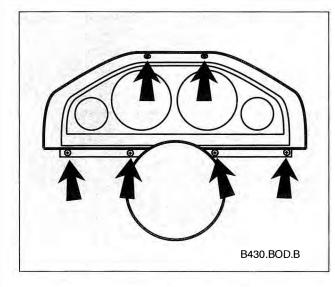
Fig. 4-3. Instrument cluster trim plate retaining screws (arrows) to be removed.
