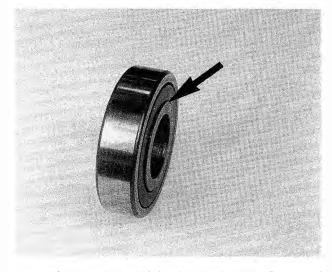
Fig. 7-24. Input shaft bearing showing protruding part of inner race (arrow). Protruding side of inner race faces gear train.
