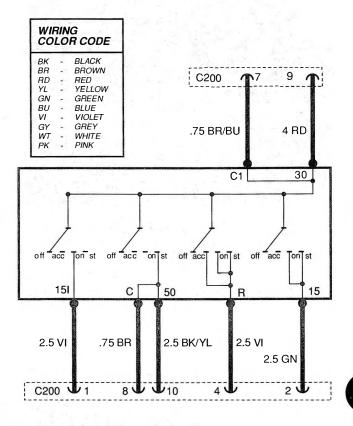
Fig. 10-11. Schematic diagram of ignition switch.
