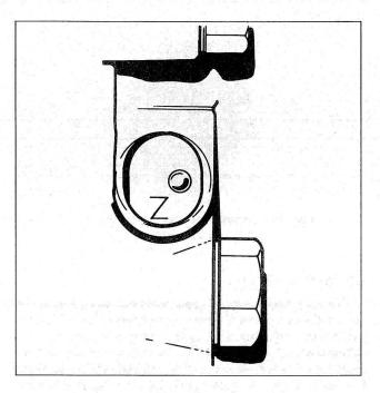
Fig. 4-15. Timing ball used to time models with 0 237 002 096 distributors.
