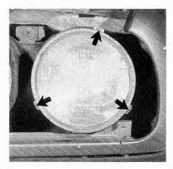
Fig. 6-1. Sealed beam headlight and retaining ring screws (arrows).
