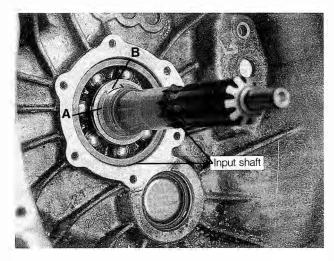
Fig. 7-2. Input shaft circlip (A) and spacer (B) on Getrag 260 transmission.
