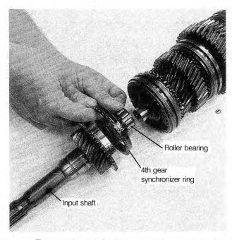
Fig. 7-30. Input shaft with 4th gear, 4th gear synchronizer ring, and roller bearing being removed.
