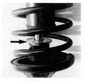
Fig. 5-8. Threaded collar (arrow) on top of strut housing retains shock absorber cartridge.
