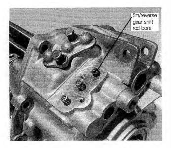
Fig. 7-17. Shift rod detent balls and springs installed into transmission case. Detent balls are under springs.
