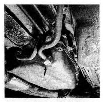
Fig. 7-9. Automatic transmission fluid filler dipstick/tube mounting nut (arrow).
