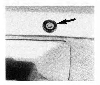
Fig. 6-19. Mounting bolt (arrow) for one-piece bumper. Remove bolts from both sides.
