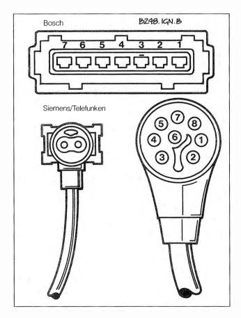
Fig. 4-2. Control unit connectors and terminal identification.
