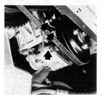
Fig. 7-18. Power steering pump mounting bolts (arrows).
