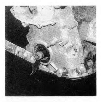
Fig. 6-1. Crankshaft oil seal being removed.
