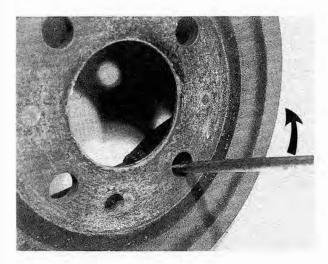
Fig. 6-3. Rear drum brake with screwdriver inserted into wheel bolt hole. Rotate screwdriver in direction of arrow to retract brake shoes.
