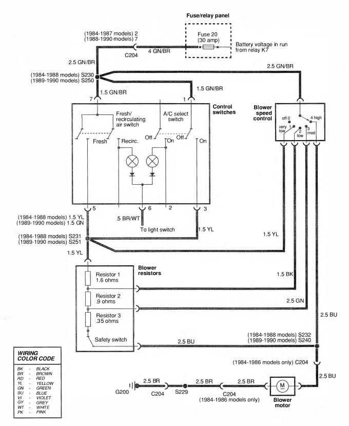
Fig. 11-3. Fresh air blower motor circuit for 1985 and later models. Circuit for 1984 models varies slightly.
