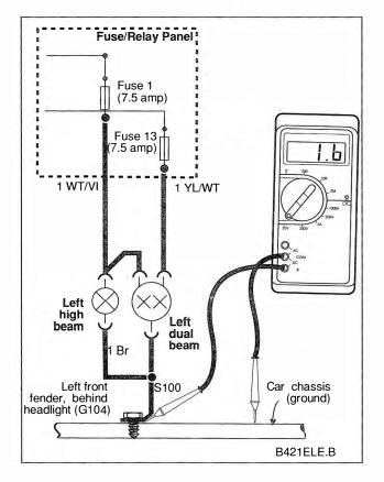
Fig. 3-6. Example of voltage drop test on dim headlights. Voltmeter showed 1.6 volt drop between ground connector and chassis ground. After removing and cleaning headlight ground connector (G104), voltage drop returned to normal (0.2 volts) and headlights were bright.
