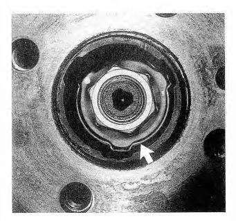
Fig. 6-8. View of rear hub showing axle nut and lockplate (arrow).
