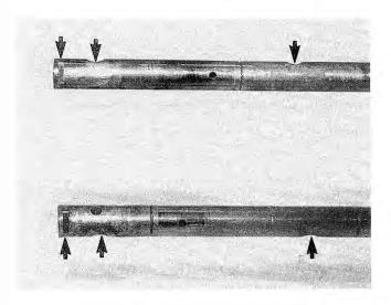
Fig. 4-36. Removed rocker arm shafts showing notches for front guide plate and cylinder head bolts (arrows).
