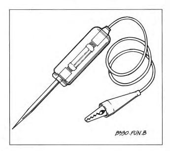
Fig. 4-13. Test light with alligator clip test lead.
