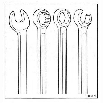
Fig. 4-2. Types of wrench heads. From left, open-end, 12point box-end, 6-point box-end, flare nut.
