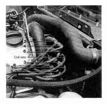
Fig. 5-11. Spark plugs wires correctly installed in distributor cap of 6-cylinder engine.
