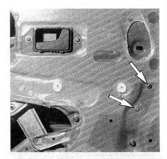
Fig. 5-23. Central locking drive securing nuts (arrows).
