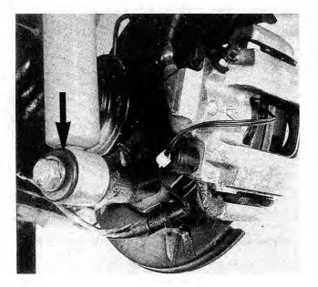
Fig. 6-1. Lower mount for rear shock absorber (arrow).
