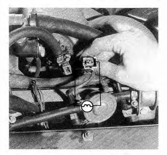
Fig. 6-12. Schematic view of test light connected across cold-start valve harness connector.
