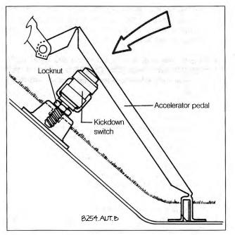
Fig. 4-8. Kickdown switch and accelerator pedal.
