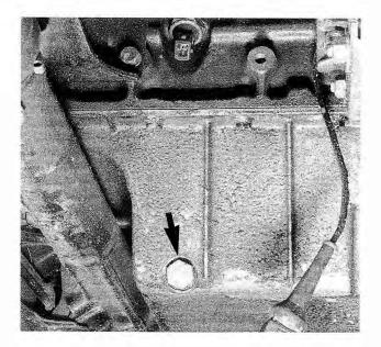
Fig. 4-3. Engine oil drain plug (arrow) in oil pan underneath engine (6-cylinder engine shown). Drain plug on 4-cylinder engine is similar.
