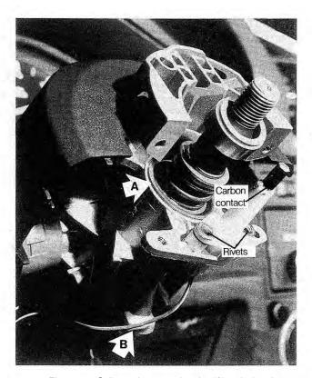
Fig. 7-11. Collar, spring, upper bearing (A) and related parts must be removed for access to steering lock mechanism. Shear bolt (B) fastens ignition/steering lock mechanism to steering column housing. Carbon contact is for horn.
