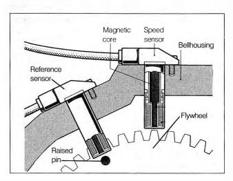
Fig. 5-2. Schematic of reference sensor and speed sensor on 1984 through 1987 325e(es) models. Courtesy Robert Bosch Corp.
