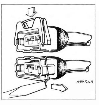
Fig. 3-5. Common versions of harness connectors. Harness connector with quick disconnect feature (top). Harness connector with retaining clip (bottom).
