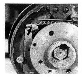
Fig. 6-7. Parking brake cable attached to rear brake shoe (arrow).
