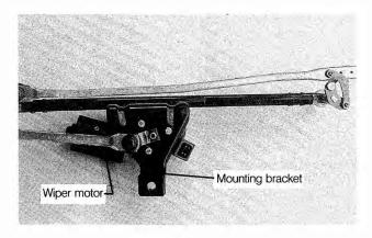
Fig. 8-7. Wiper linkage assembly with wiper motor.
