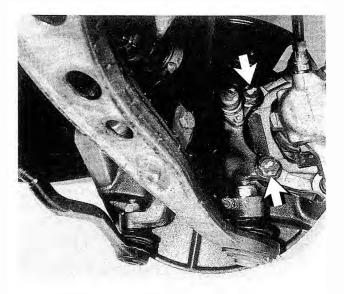
Fig. 5-19. Front brake caliper mounting bolts (arrows). Right (passenger) side shown.
