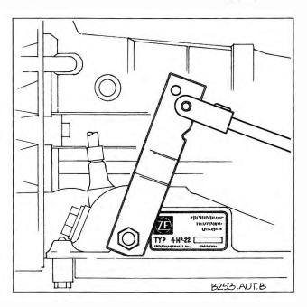
Fig. 3-10. Location of data plate on automatic transmission.
