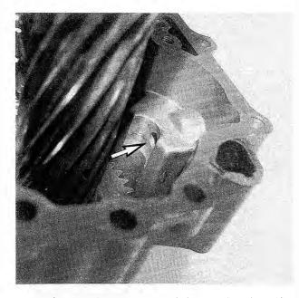
Fig. 7-20. Area of rear transmission case (arrow) requiring gasket sealer.
