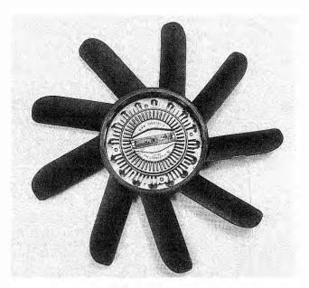
Fig. 4-17. Radiator cooling fan and clutch assembly.
