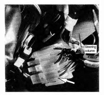
Fig. 10-12. Ignition switch harness connector C200 (arrow). Lower steering column trim removed from steering column. Make continuity tests at switch side of connector.
