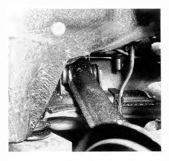
Fig. 6-14. Outer rear suspension trailing arm mount on top of rear axle carrier.
