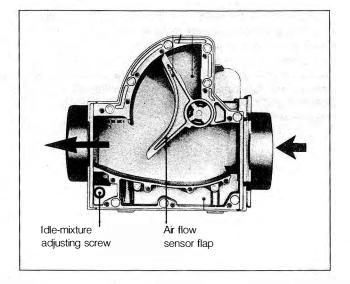
Fig. 5-2. Cutaway view of air flow sensor. Arrows indicate direction of air flow. Courtesy Robert Bosch Corp.
