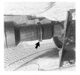
Fig. 4-3. Clamping sleeve for sliding coupling (arrow) to be loosened.
