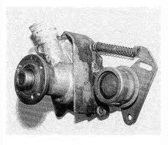
Fig. 4-14. Relationship of camshaft belt tensioner pulley, tensioner spring and pin, and coolant pump.
