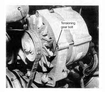
Fig. 6-2. Alternator mounting bolts (A and B), and pivot bolt
