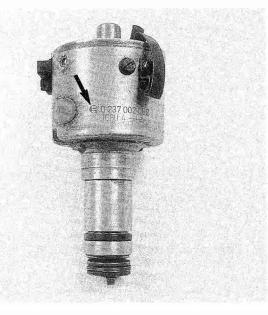
Fig. 4-12. Distributor code number location (arrow). Distributor shown is not one of those covered by this manual.
