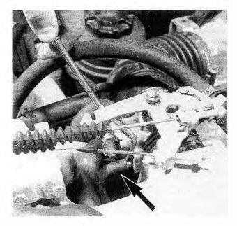
Fig. 6-28. Small vacuum hose from charcoal canister (arrow) being removed and vented to atmosphere.
