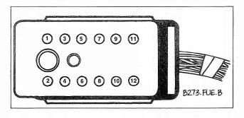
Fig. 6-19. Idle speed control unit harness connector terminal identification. Terminal numbers are also printed on connector. Remove trim panel above glove compartment to access control unit.
