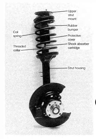
Fig. 5-1. Front suspension strut assembly.
