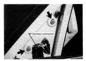
Fig. 5-28. Side mirror housing mounting bolts (arrows), behind small trim panel or radio speaker.
