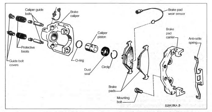
Fig. 7-14. Exploded view of rear brake caliper.
