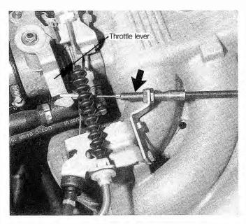
Fig. 3-2. Transmission accelerator cable (arrow).
