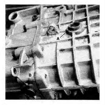
Fig. 7-4. Remove oil filler plug (A) to check transmission lubricant level. Remove oil drain plug (B) to replace lubricant. Use 17 mm hex wrench to remove plugs.
