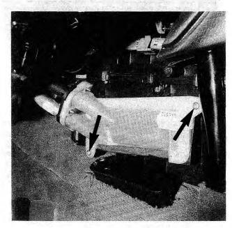
Fig. 4-24. Heater core mounting screws (arrows).
