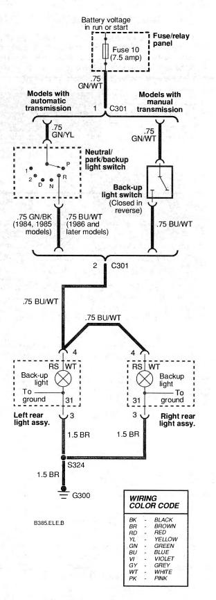
Fig. 10-10. Back-up lights circuit.
