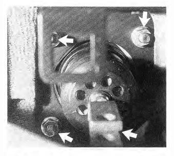
Fig. 4-5. Vacuum booster mounting nuts (arrows) as viewed from inside the passenger compartment.
