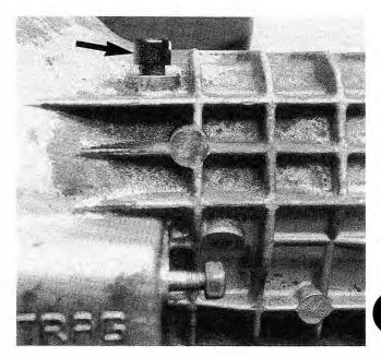
Fig. 7-43. Manual transmission vent (arrow). Check vent for free movement up and down.
