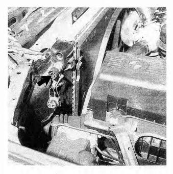
Fig. 4-22. Single thermo-switch (arrow) on 325i(is) models. Connector shown disconnected from switch.
