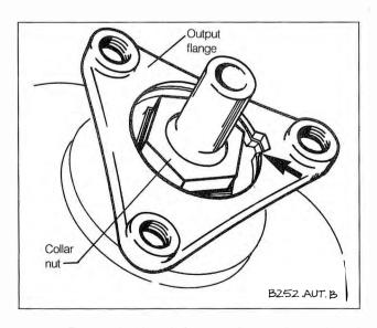
Fig. 5-7. Locking tab for output flange collar nut (arrow). Bend tab out of groove to remove nut.
