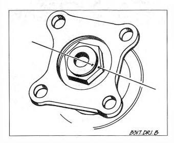
Fig. 5-8. Final drive input shaft, collar nut, and flange, showing matching marks made with punch.
