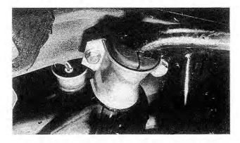
Fig. 5-21. Brackets and rubber bushings mount stabilizer bar to front suspension subframe.
