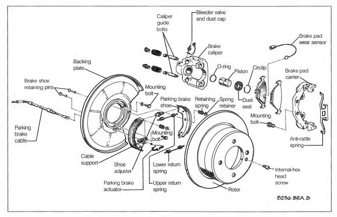
Fig. 7-1. Exploded view of rear disc brake assembly.
