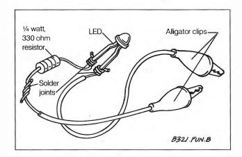
Fig. 3-4. Do-it-yourself LED test light for safe testing of ignition, fuel injection, and emission control circuits.
