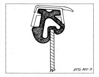
Fig. 8-4. Correct fit of convertible windows against window seals.
