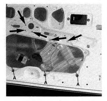
Fig. 5-14. Window regulator retaining screws (arrows) and wire ties (A). Plastic moisture barrier must be removed for access.
