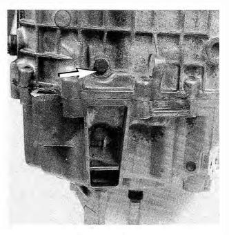
Fig. 7-5. Reverse gear shaft retaining bolt (arrow) in front transmission case.
