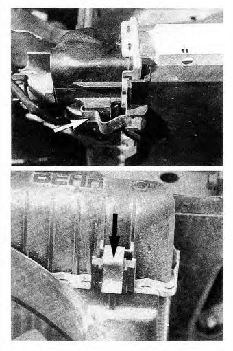
Fig. 4-27. Radiator shroud mounting clips used on 1984-1987 6-cylinder models (top) and all 4-cylinder models (bottom). Clips on 1988-1990 models are similar.
