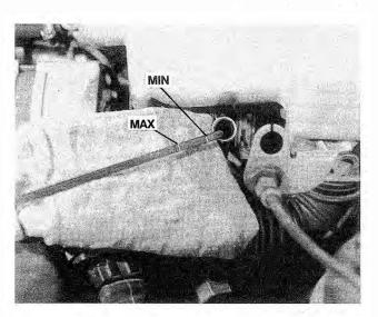
Fig. 4-1. Maximum (MAX) and minimum (MIN) oil level marks on dipstick.
