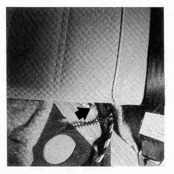
Fig. 3-8. Ground point G300 (arrow) for fuel pumps beneath rear seat bottom on driver's side. Ground point G202 (not shown), used on convertible model only, is also beneath rear seat on passenger's side.
