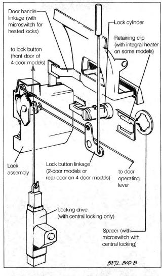
Fig. 5-21. Phantom view of lock linkage used on front doors of 2-door models with central locking. Linkage differs slightly for other door applications.
