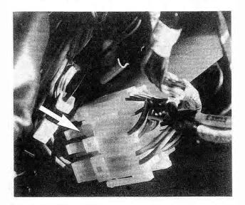
Fig. 8-3. Wiper/washer switch harness connector (arrow).
