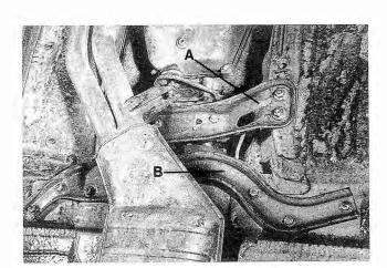
Fig. 5-4. Rear transmission support (A) and reinforcement bar (B) to be removed.
