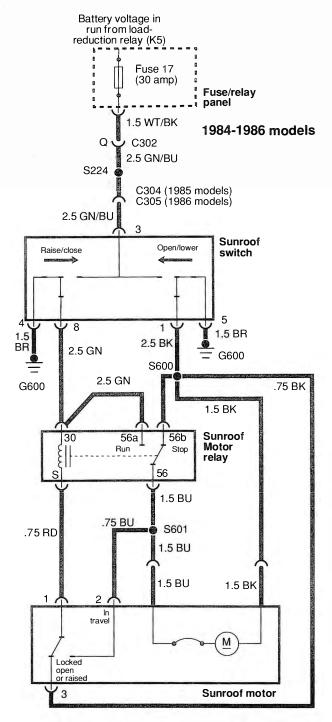
Fig. 12-1. Circuit diagram for the power sunroof on 1984 through 1986 models (left) and 1987 through 1990 models (right).
