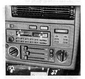
Fig. 4-25. To release heater trim panel for access to back of operating levers, remove screws from underneath (A) and behind switches (B).
