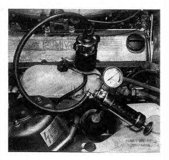
Fig. 3-2. Pressure tester shown installed on expansion tank of 6-cylinder engine. On 4-cylinder engine, install pressure tester in place of radiator cap.
