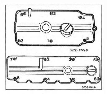
Fig. 4-5. Cylinder head cover mounting nut tightening sequence on 4-cylinder engines (top) and 6-cylinder engines (bottom).
