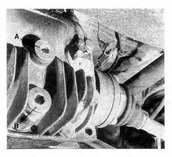
Fig. 7-12. Final drive oil filler plug (A) and oil drain plug (B).
