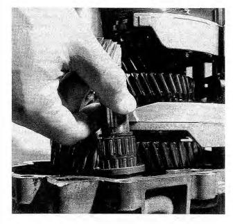
Fig. 7-7. Reverse gear shaft being withdrawn from transmission case.
