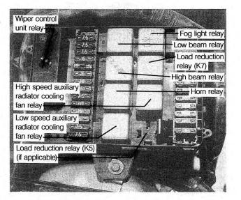
Fig. 14-1. Fuse/relay panel on BMW models covered by this manual. Low beam check relay is on underside of panel and is integrated into panel's printed circuit.
