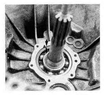
Fig. 7-26. Input shaft bearing depth in case (dimension A).
