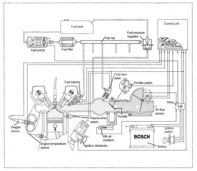
Fig. 5-1. Schematic view of L-Jetronic fuel injection system. Art courtesy of Robert Bosch Corporation
