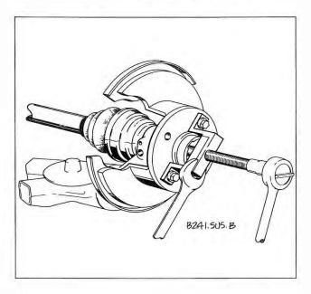
Fig. 6-9. Puller being used to press rear stub axle from wheel hub to remove axle shaft.
