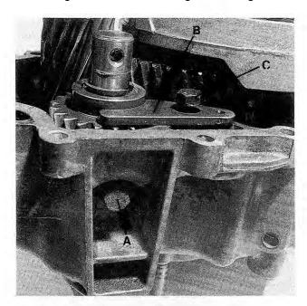
Fig. 7-6. Reverse gear shaft retaining bolt (A), retaining bracket (B), and bracket mounting bolt (C).
