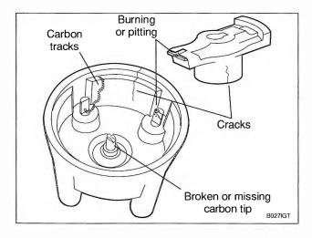
Fig. 3-2. Distributor cap and rotor. Inspect cap and rotor at contact points.
