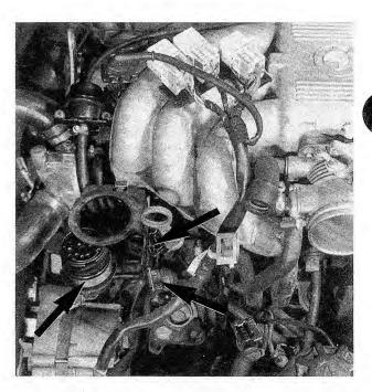
Fig. 5-23. Reference and speed sensor connectors and diagnostic connector removed from bracket (arrows).
