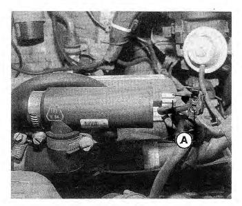
Fig. 5-13. Ammeter connected to plastic idle air stabilizer valve (shown schematically) to measure current from the idle speed control unit.
