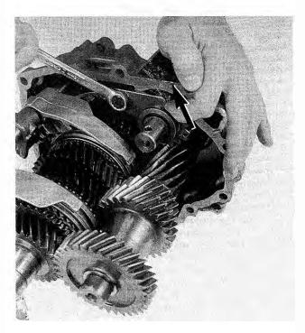
Fig. 7-21. Reverse gear shaft retaining bracket correctly positioned. Apply outward pressure (arrow) and then tighten bolt.
