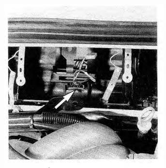
Fig. 11-4. Series resistor plate behind blower motor housing (arrow).
