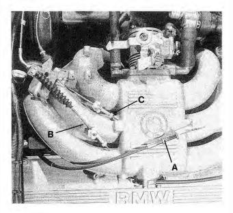
Fig. 6-6. Automatic transmission accelerator cable (A), cruise control cable (B), and accelerator cable (C).
