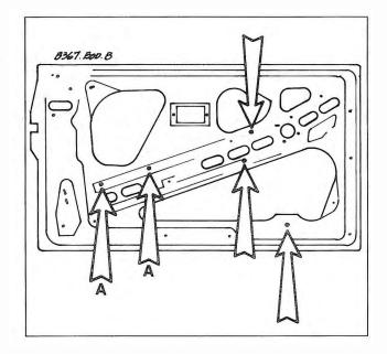
Fig. 8-5. Screws to be loosened (A) to make parallel fit of window glass. Other arrows do not apply to this procedure.
