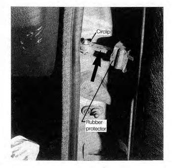
Fig. 5-2. Door check rod (arrow). Remove circlip and press out pin.
