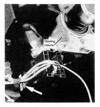
Fig. 10-3. Turn signal/emergency flasher relay (arrow) and harness connector. Flasher is located beneath steering column trim, below steering wheel.
