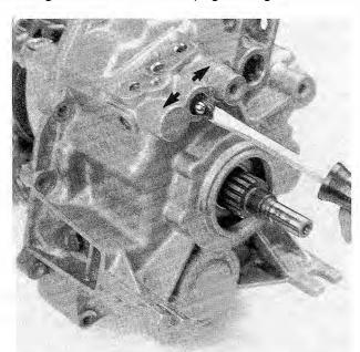
Fig. 7-15. Shift rod detent balls being installed into transmission rear case. Arrows indicate position of balls.
