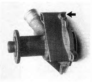
Fig. 4-16. Coolant pump detent (arrow) for camshaft drive belt tensioner spring.
