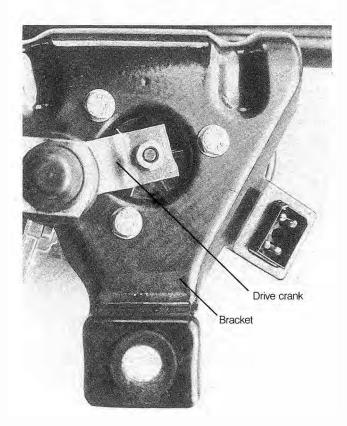
Fig. 8-8. Wiper motor assembly. Mark position of drive crank on bracket before removing motor from bracket.
