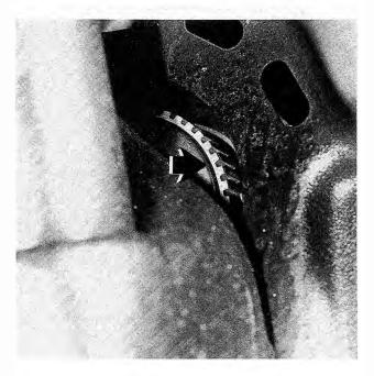
Fig. 4-13. Front-left ABS pulse wheel (arrow).
