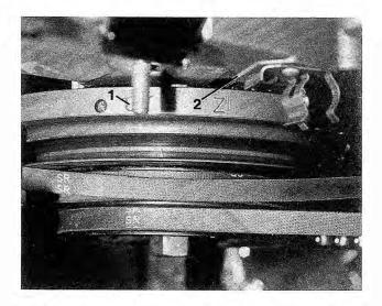
Fig. 4-61. Top Dead Center (TDC or 0/T) mark (1) on vibration damper should be aligned with mark on drive belt cover (2).
