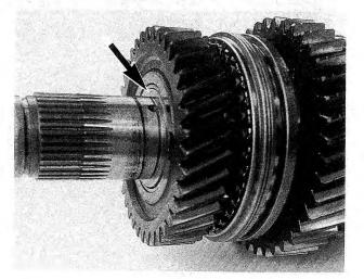
Fig. 7-41. Output shaft bearing surface protruding above second gear shoulder (arrow).
