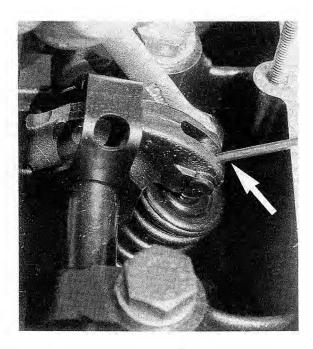
Fig. 4-28. Valve clearance being adjusted. Stiff wire hook inserted into hole in eccentric (arrow).
