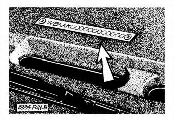
Fig. 3-6. Location (arrow) of vehicle identification number (VIN) on 1984-1990 BMW cars.
