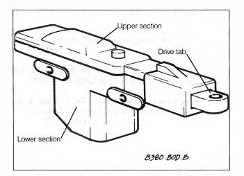
Fig. 5-26. Central locking system locking drive. See Table a. for correct identification of drives.
