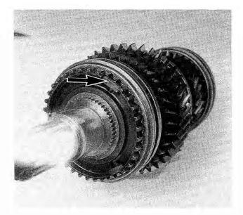
Fig. 7-35. Guide sleeve operating dog correctly installed with beveled edge facing operating sleeve (arrow). On early transmissions, dog with stepped side faces operating sleeve.
