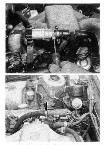
Fig. 5-15. Adjusting idle air stabilizer valve. Top On metal valve, adjusting screw is external. Bottom On plastic valve, adjusting screw is visible after removing hose (arrow).
