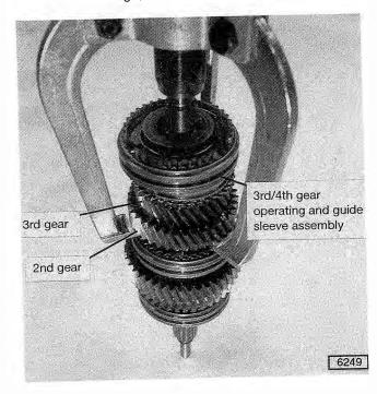
Fig. 7-32. 3rd gear cluster and 2nd gear being removed from output shaft of Getrag 260 transmission.
