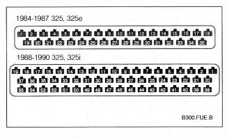
Fig. 6-23. Terminal identification for 35-point Motronic control unit connector (top) and 55-point Motronic 1.1 control unit connector (bottom).
