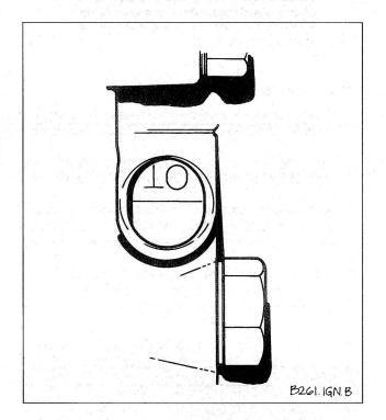
Fig. 4-14. Timing mark used to time models with 0 237 002 080 distributors.
