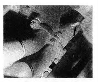
Fig. 6-8. Oxygen sensor mounted in exhaust manifold (arrow) on 1984 318i model as viewed from beneath car. Location of sensor varies between models.
