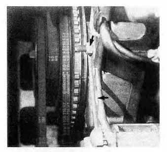
Fig. 4-9. Upper alternator bracket and mounting nut and bolt (arrows).
