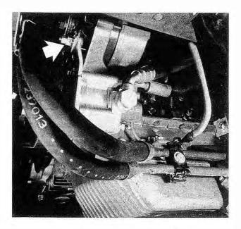
Fig. 7-19. Power steering pump belt tension adjuster (arrow).
