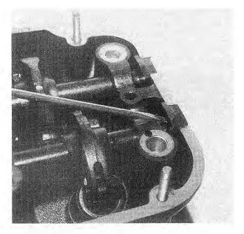
Fig. 4-39. Rubber retaining plug being removed from cylinder head.
