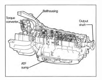
Fig. 1-1. Phantom view of 4-speed ZF 4 HP 22 automatic transmission.
