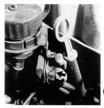
Fig. 5-7. Pulse sensor connector for 325i(is) engine (arrow).
