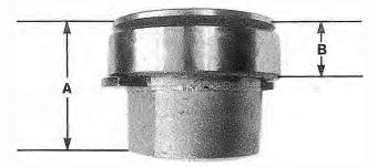
Fig. 5-13. Clutch release bearing should be checked for wear at dimension **A** and dimension **B**.
