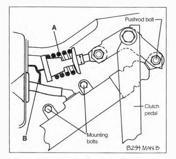
Fig. 5-6. Clutch pedal over-center helper spring (A) and spring guide (B).
