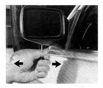
Fig. 5-29. Insert screwdriver as shown to engage tab on mirror-glass locking ring, then push in either direction to unlock glass.
