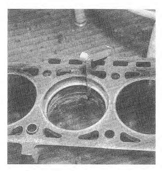
Fig. 6-7. Piston ring end gap being checked in cylinder block using feeler gauge.
