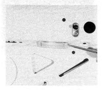
Fig. 4-17. Luggage compartment light assembly being pried out.
