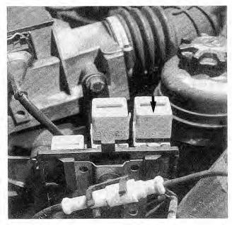
Fig. 5-4. Oxygen sensor heater relay (arrow). Relays shown with protective cover.
