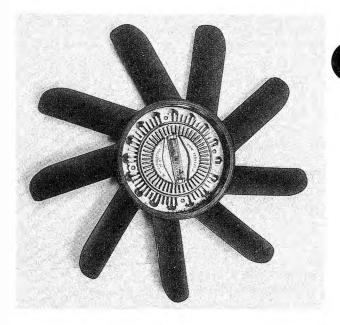
Fig. 3-1. Primary cooling fan and clutch assembly.
