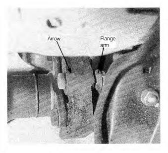
Fig. 4-9. When attaching flexible coupling to driveshaft or to transmission flange, arrows must point toward flange arms as shown.
