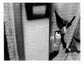
Fig. 6-14. Mounting nut for rear door body side molding is beneath rubber plug (arrow).
