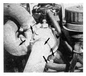
Fig. 4-50. Coolant hoses to be removed from cylinder head (arrows).
