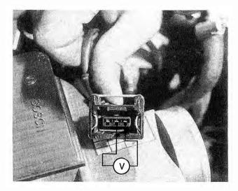
Fig. 6-17. Schematic view of voltmeter being used to test idle stabilizer valve voltage signal from the control unit, on models with 3-wire valves (Motronic 1.1).
