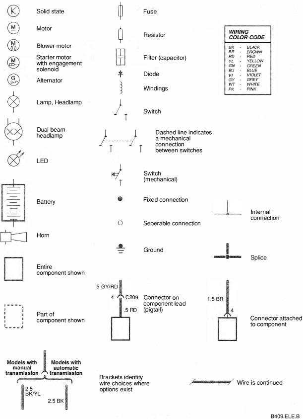
Fig. 3-9. Wiring and component symbols in the wiring diagrams in this section of the manual.
