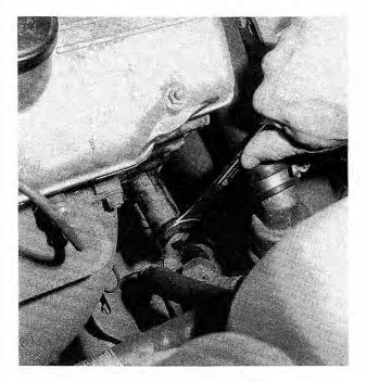
Fig. 4-18. Camshaft timing chain tensioner piston being removed.
