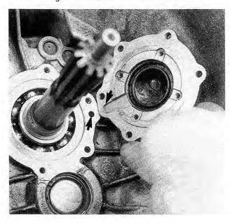
Fig. 7-28. Clutch guide seal oil groove and transmission case oil bore (arrows).
