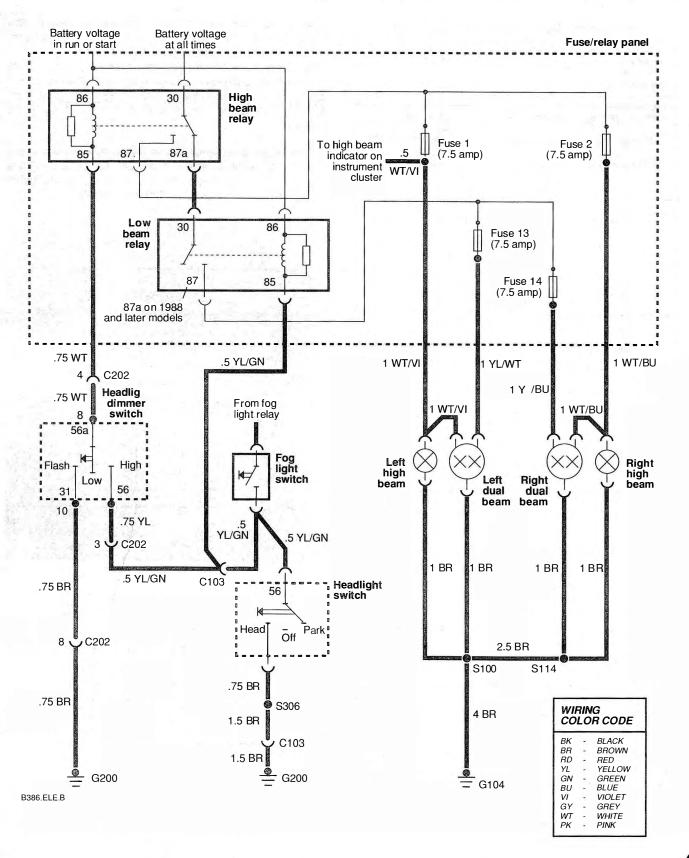
Fig. 10-2. Headlight circuit for models without active check control. Circuit may vary slightly on some models.
