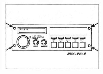
Fig. 4-12. Access holes (arrows) for retaining clips of early BMW radios. Release clips by inserting stiff wire in holes.
