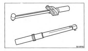
Fig. 4-10. Torque wrenches. Inexpensive beam-type (top) is adequate but must be read visually. Ratchet-type (bottom) can be preset to indicate when torque value has been reached.
