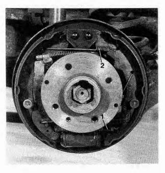
Fig. 6-5. Rear brake lower return spring (1) and upper return spring (2).
