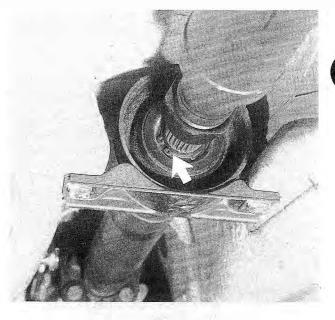
Fig. 4-12. Center bearing circlip (arrow) to be removed. Driveshaft shown installed.
