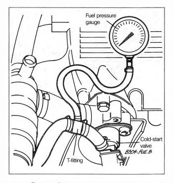
Fig. 5-22. Fuel pressure gauge connected between coldstart valve and supply line.
