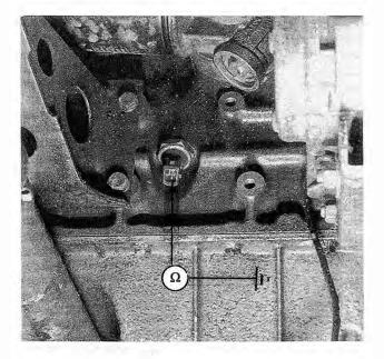
Fig. 7-3. Oil pressure switch being tested using an ohmmeter (shown schematically). Switch on 6-cylinder model shown. Switch on 4-cylinder model is similar.
