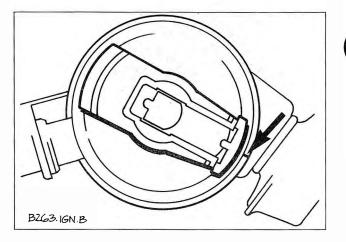
Fig. 4-8. Distributor rotor aligned with No. 1 cylinder TDC mark (arrow) on distributor housing.
