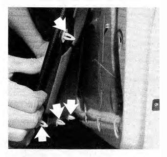
Fig. 5-12. Door interior trim panel being removed, showing securing clips (arrows).
