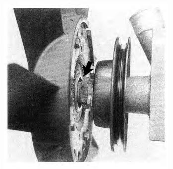
Fig. 4-18. Nut (left-hand thread) on fan clutch (arrow).
