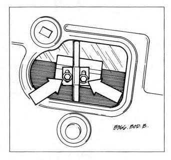
Fig. 5-13. Bolts (arrows) that secure window glass to window regulator.
