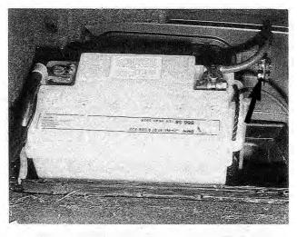
Fig. 3-12. Ground point G100 (arrow) from battery to chassis on all 325 models with battery in left side of trunk.
