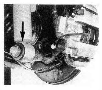
Fig. 6-5. Lower mount for rear shock absorber (arrow).
