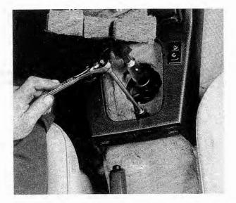
Fig. 4-7. Console mounting nut being removed.
