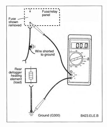
Fig. 3-4. Ohmmeter being used to check for a short circuit to ground.
