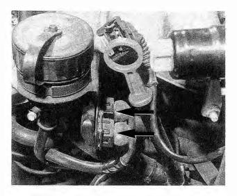
Fig. 4-58. Reference point sensor and speed sensor connectors (arrows).
