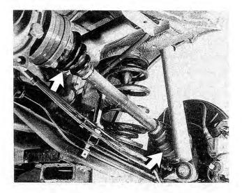
Fig. 6-7. Drive axle and CV joints. Rubber boots (arrows) retain lubricant and protect joints from dirt.
