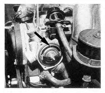
Fig. 4-8. Thermostat correctly positioned in coolant outlet. Arrow shaped mark (arrow) must point up.
