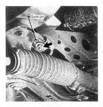
Fig. 5-25. Left engine mount nut (arrow) as viewed from under the car.
