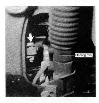
Fig. 5-10. Location of engine damper. Remove damper through-bolt (arrow).
