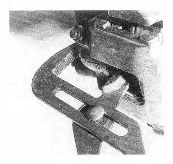
Fig. 7-5. Water pump pliers being used to carefully push piston into caliper.
