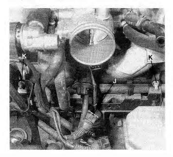
Fig. 5-22. Fuel injector wiring harness connector (j) and bracket mounting nuts (k).
