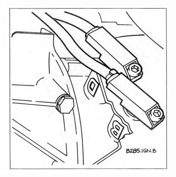
Fig. 5-6. Bellhousing reference sensor position (B) and speed sensor position (D).
