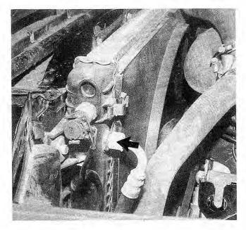
Fig. 4-28. Automatic transmission cooler line on radiator of 6-cylinder engine (arrow). Transmission cooler lines on 4-cylinder engine are at radiator bottom.
