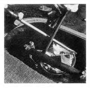
Fig. 4-7. Transfer pump and fuel gauge sending unit being removed from fuel tank. Use two screwdrivers to engage lugs on housing.
