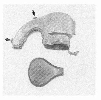
Fig. 4-7. Distributor cap protective covers installed on 4cylinder engines. Pry cap apart at points indicated by arrows.
