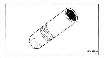
Fig. 4-5. Spark plug socket.
