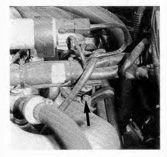
Fig. 3-7. Ground point G102 (arrow) for fuel injection system on all 318i models (rear of engine, below no. 4 fuel injector).
