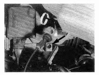
Fig. 6-30. Air flow sensor idle mixture screw (arrow), beneath anti-tampering plug.
