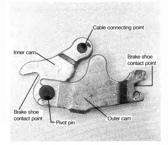
Fig. 7-12. Parking brake actuator components used on cars with rear disc brakes.
