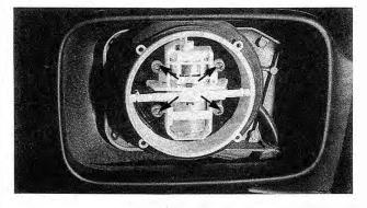
Fig. 5-30. Motor and mounting screws (arrows) for electric side mirrors.
