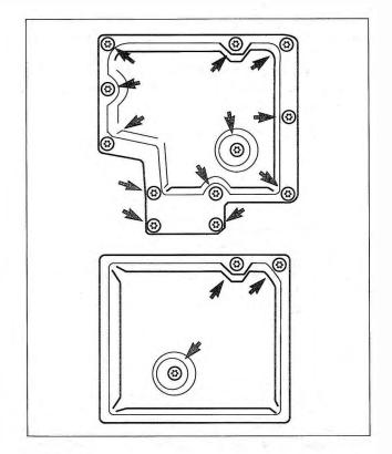
Fig. 7-11. Transmission fluid strainer mounting bolts (arrows) for 3-speed transmission (3 HP 22) (top), and 4-speed transmission (4 HP 22) (bottom).
