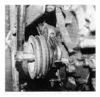
Fig. 4-25. Vibration damper secured with wrench while mounting nut is tightened.
