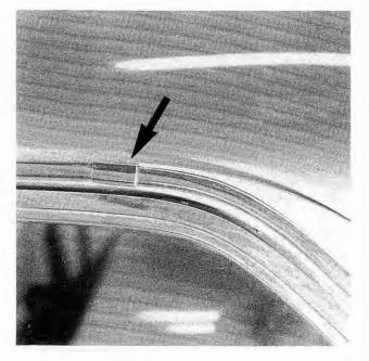
Fig. 6-16. Clip on rain gutter molding (arrow) to be moved back.
