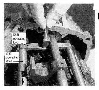
Fig. 7-8. Shift operating lever locking pin being removed. Slide out shaft in direction of arrow.
