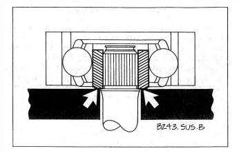
Fig. 6-11. When pressing inner CV joint from axle shaft, support joint on inner hub only (arrows).
