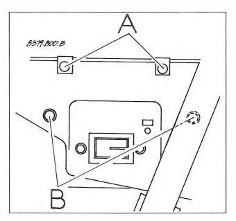
Fig. 8-7. Convertible rear window adjustment screws for parallel fit (A) and vertical fit (B).
