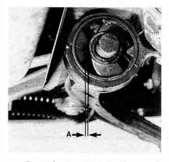
Fig. 5-12. Control arm rubber bushing. Measure gap (A) with car at rest on ground and loaded. See text.
