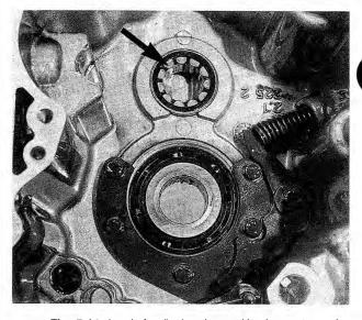
Fig. 7-14. Layshaft roller bearing position in rear transmission housing with large side of cage facing up (arrow).
