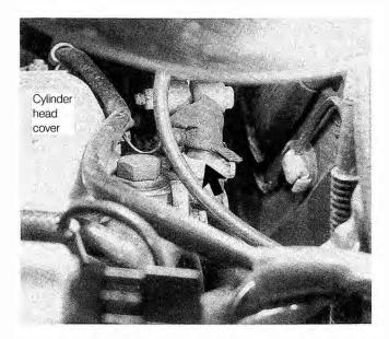
Fig. 7-2. Oil pressure switch on 4-cylinder engine (arrow).
