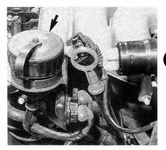
Fig. 2-2. Diagnostic connector in engine compartment (arrow).
