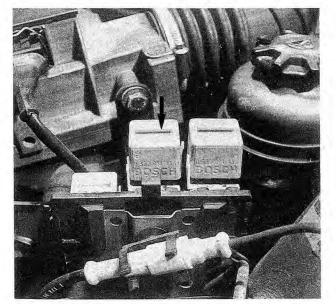
Fig. 3-2. Auxiliary relay panel near left shock tower on 6cylinder engine. Remove cover from panel and remove main relay (arrow).
