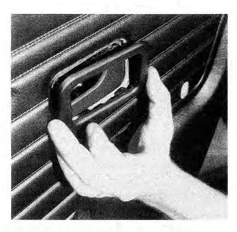
Fig. 5-7. Door handle trim being removed. Slide trim to rear then pull off.
