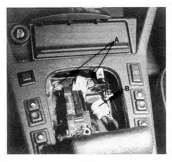
Fig. 4-5. Selector lever assembly showing screws (A) and wiring harness (B).
