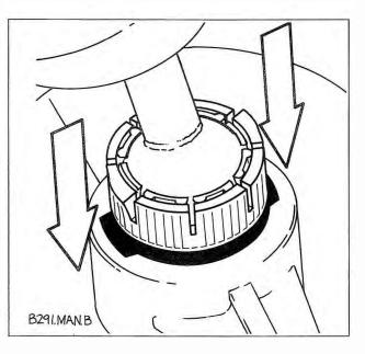
Fig. 4-6. Shift lever being installed.
