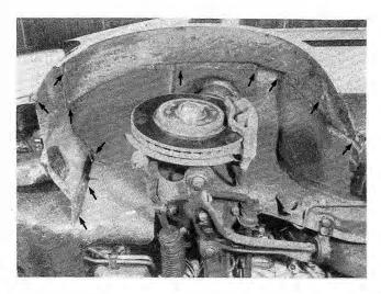
Fig. 6-12. Wheelhouse liner mounting bolts (arrows).
