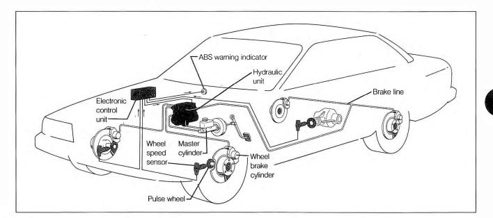
Fig. 4-12. Schematic representation of typical anti-lock braking system (ABS). Exact location and configuration of components may vary.
