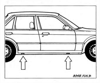
Fig. 3-1. Jacking points for use with BMW-supplied jack.
