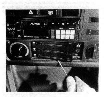
Fig. 4-29. Removing air conditioning control switch assembly trim plate.
