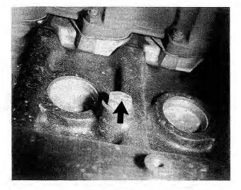
Fig. 4-2. Typical location of coolant drain plug (arrow) on right side of engine (6-cylinder engine shown).
