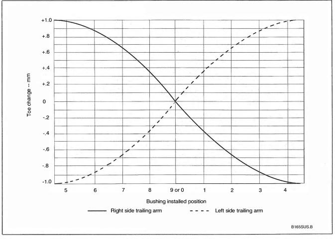
Fig. 6-18. Nominal toe correction (mm) vs. installed position of trailing arm eccentric bushings. Notice that positions for left and right side trailing arms are different.
