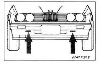
Fig. 6-3. Front towing eyes (arrows) used when flat-towing cars.
