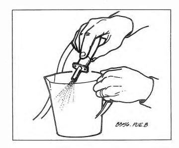
Fig. 6-11. Cold-start valve operation being checked.
