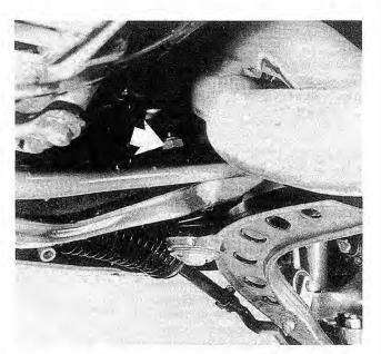
Fig. 5-15. Self-locking nut (arrow) secures ball joint to subframe.
