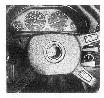
Fig. 7-4. Large nut secures steering wheel to steering column. Mark wheel and steering column shaft prior to removal to ensure proper alignment for reinstallation.
