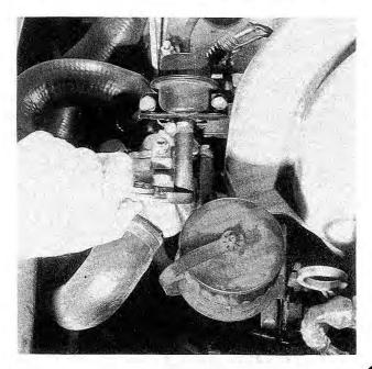
Fig. 6-26. Fuel pressure regulator return hose being clamped shut to check fuel pump delivery pressure.
