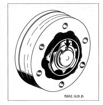
Fig. 6-10. Circlip (arrow) securing inner CV joint to axle shaft. Always replace.
