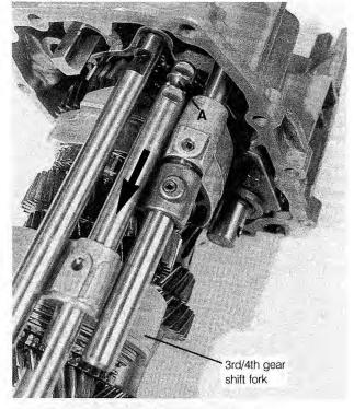
Fig. 7-11. 3rd/4th gear shift rod being removed. Arrow shows direction of removal. Note small pin (A) in end of rod.
