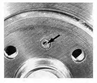
Fig. 5-8. Front rotor mounting screw (arrow).
