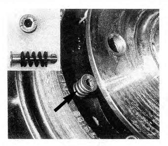
Fig. 7-11. Rear parking brake shoe retaining spring and spring retainer (arrow). Inset shows retainer assembly.
