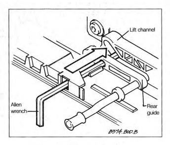
Fig. 7-6. Allen wrench inserted through rear guides to lock guides in place. Lock both sides.
