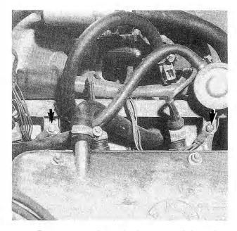
Fig. 4-28. Fuel rail mounting bolts on 4-cylinder engines (arrows).
