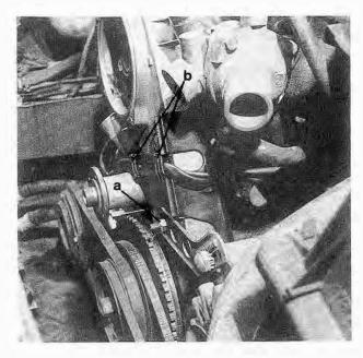
Fig. 4-13. Upper alternator mounting bracket nut (a) and wire holder retaining clips (b) on camshaft drive belt cover.
