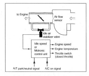
Fig. 6-1. Schematic of idle speed control system.
