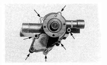
Fig. 4-11. Coolant pump mounting points (arrows) on 4-cylinder engine.
