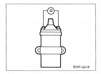
Fig. 3-5. Primary coil resistance being measured than ohmmeter (shown schematically) betweer. arminals 1 and 15. Measurement of secondary resistance is similar.
