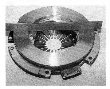
Fig. 5-12. Clutch pressure plate friction surface being checked for flatness using straightedge.
