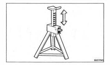
Fig. 4-8. Jack stand for safely supporting car to work underneath.
