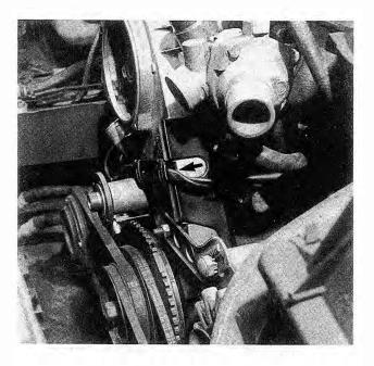
Fig. 5-8. Pulse sensor wiring routed through protective covering (arrow).
