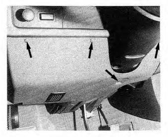
Fig. 4-1. Retaining screws (arrows) to be removed from leftside instrument panel trim.
