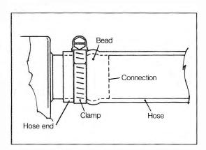
Fig. 4-6. Hose clamp correctly installed on hose end.
