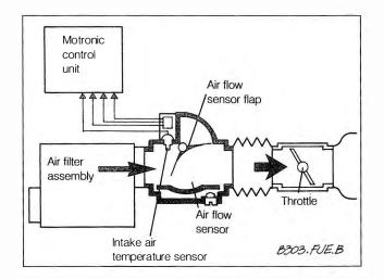
Fig. 6-2. Schematic of air flow sensor and related components. Arrows indicate direction of air flow.
