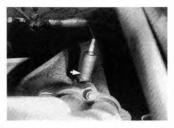
Fig. 1-2. Oxygen sensor (arrow) installed in 4-cylinder exhaust manifold.
