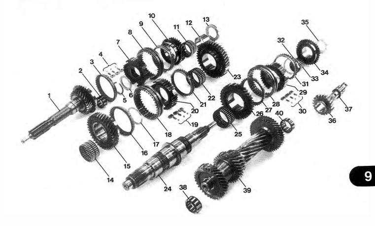
Fig. 7-29. Getrag 240 and 260 gear train components.
