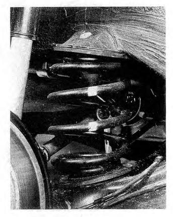
Fig. 6-6. Normal installed position of rear coil spring.
