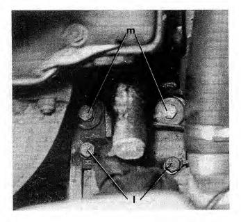
Fig. 5-9. Air conditioning compressor mounting bolts. Loosen outer bolts (I) and remove inner bolts (m).
