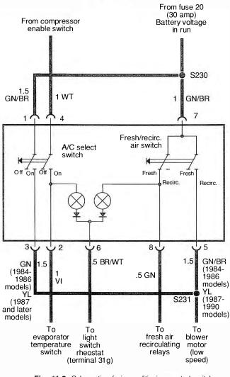
Fig. 11-2. Schematic of air conditioning control switch assembly.
