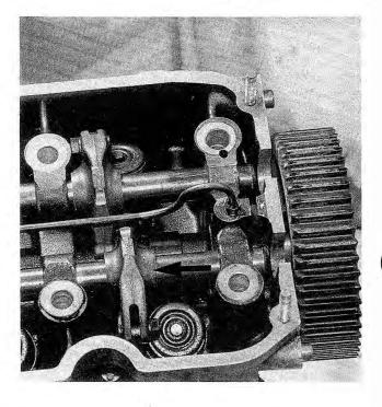
Fig. 4-40. Rocker arm positioned (arrow) for removal of exhaust-side rocker arm shaft.
