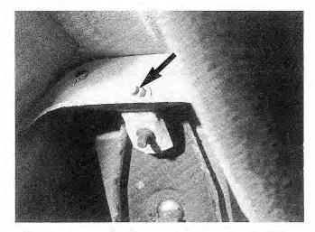
Fig. 4-7. Shift console rear mounting nut to be removed (arrow). Model with sheet-metal console shown. Aluminum console is similar.
