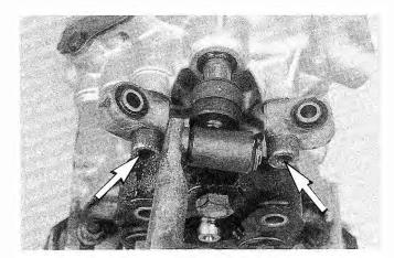
Fig. 4-8. Shift console-to-transmission mounting bolts (arrows) to be removed. Transmission shown removed.
