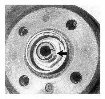
Fig. 5-18. Collar nut locked into front stub axle. Unlock nut by breaking locked portion (arrow) with chisel.
