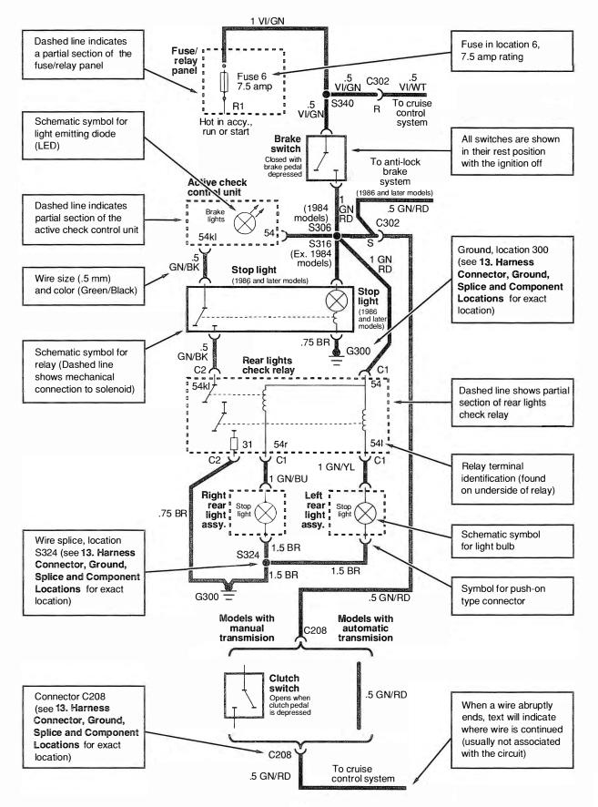
Fig. 3-8. Sample wiring diagram of stop light circuit on models with active check control.
