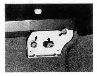
Fig. 6-27. Trunk lock mounting bolts (arrows).
