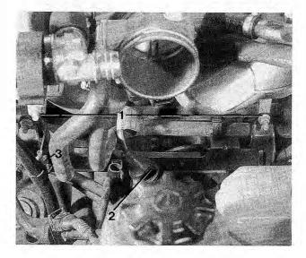
Fig. 4-54. Mounting nuts for wire harness retaining bracket (1), fuel injector harness connector (2), and oil dipstick mounting bracket (3).
