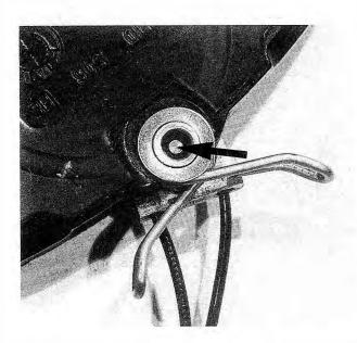
Fig. 5-5. Front brake pad and wear sensor. Remove sensor from pad by driving pin (arrow) down.
