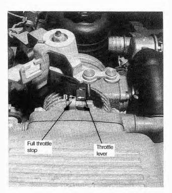
Fig. 4-24. Correct amount of clearance at full-throttle stop (dimension B). 6-cylinder engine shown, 4cylinder engine similar.
