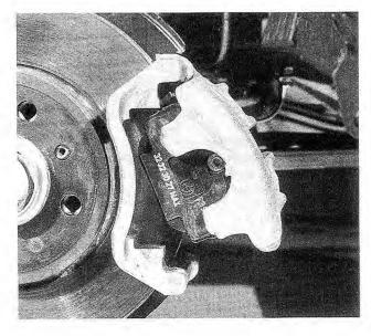
Fig. 5-4. Brake caliper being pivoted up to remove front brake pads.
