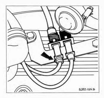
Fig. 4-3. Reference point sensor and speed sensor connector on 1984 and 1985 6-cylinder head cover.
