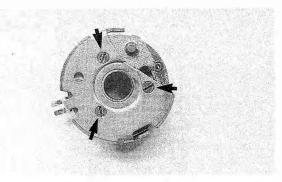
Fig. 4-11. Impulse coil mounting screws on underside of distributor base plate (arrows).
