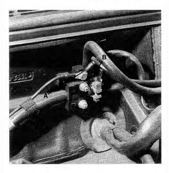
Fig. 4-1. Battery junction block in rear of engine compartment on models with battery in trunk.
