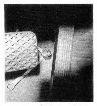
Fig. 4-25. Accelerator pedal stop locknut being loosened using two open end wrenches. Total height (measured from floor beneath carpet) should be 55 mm (2.165 in.) on automatic transmission or 60 mm (2.362 in.) on manual transmission.
