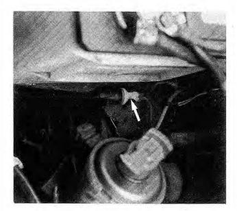
Fig. 5-1. Oxygen sensor connector (arrow) on early 1984 318i model (near left-hand side of battery). Connector on late 1984 and all 1985 318i models is similar.
