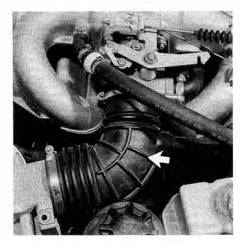
Fig. 3-3. Intake air duct (arrow) can crack or become loose. Be sure to check bottom side of duct. Air bypass hoses and hose fittings are also suspect. Bend air duct and hoses to detect cracks. 6-cylinder engine shown, 4-cylinder is similar.
