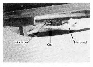
Fig. 7-5. Rear guide pin engaged in sunroof trim panel clip. Sunroof shown raised for clarity.
