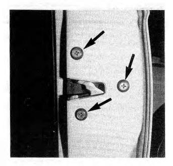
Fig. 5-24. Lock assembly securing bolts (arrows) on edge of door.
