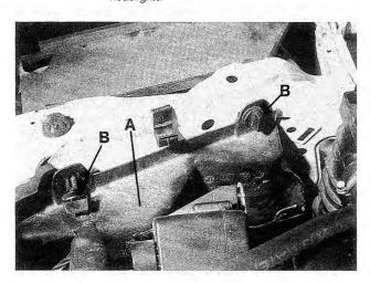
Fig. 6-4. Headlight cover (A) in front part of engine compartment. Turn fasteners (B) 90° to remove cover.
