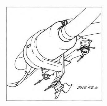
Fig. 4-16. Fuel pump bracket mounting points (arrows).
