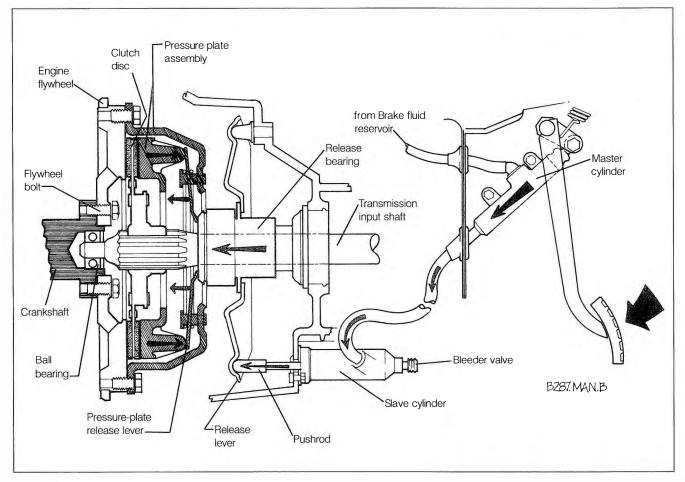
Fig. 5-1. Schematic view of hydraulic clutch components.
