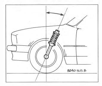
Fig. 4-2. Caster: angle of steering axis inclination from vertical. Caster is non-adjustable on cars covered by this manual.
