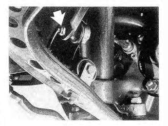
Fig. 5-4. Nut (arrow) fastens stabilizer bar to stabilizer bar connecting link. Right (passenger) side shown.
