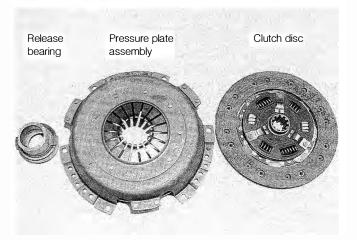
Fig. 5-2. Clutch components that are usually replaced when the clutch is overhauled.
