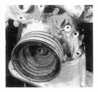
Fig. 4-15. Top Dead Center (TDC) mark on vibration damper aligned with mark on timing chain cover.
