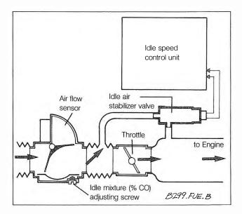
Fig. 5-12. Schematic view of idle air stabilization system showing idle air stabilizer valve and idle speed control unit
