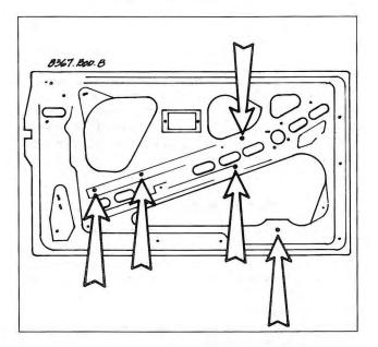
Fig. 5-15. Additional screws (arrows) on convertible front windows to be removed for window regulator removal.
