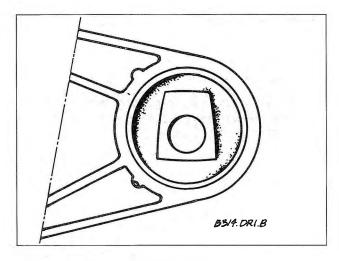
Fig. 5-5. Installed orientation of final drive rubber mounting bushing.
