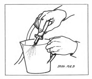
Fig. 5-9. Cold-start valve operation being checked.
