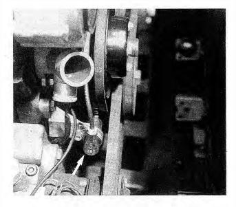
Fig. 5-3. Pulse sensor on 325i(is) and 1988 through 1990 325 engine (arrow).
