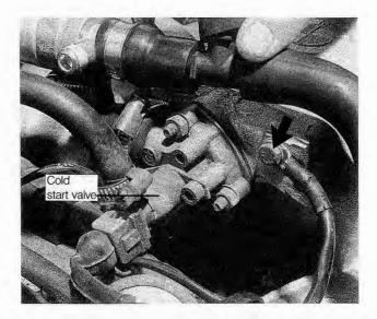
Fig. 3-6. Ground G101 (arrow) for fuel injection system on 1984 and most early 1985 318 imodels (next to cold start valve).
