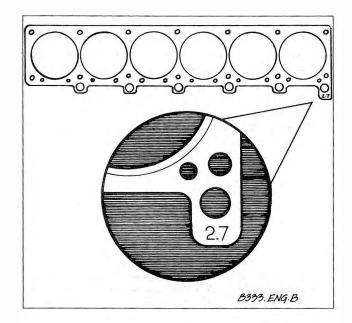
Fig. 4-63. Engine displacement code stamp on cylinder head gasket flange.
