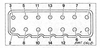
Fig. 4-62. Cylinder head bolt loosening sequence.
