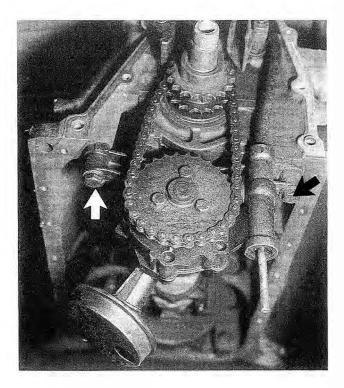
Fig. 7-8. Oil pump mounting bolts (arrows). Type of oil pump varies between models.
