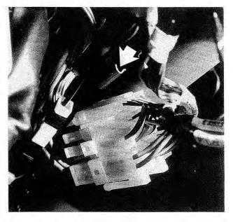
Fig. 7-9. Main harness connector cluster for steering column wiring. Connector snaps into bracket (arrow) on top of column housing. (1989 model shown).
