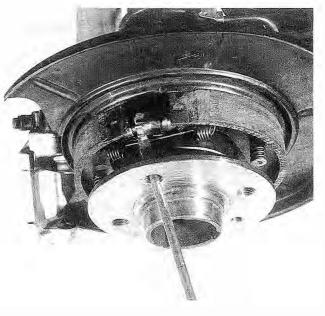
Fig. 7-10. Screwdriver inserted into lug bolt hole on left rear wheel to adjust parking brake shoes. Shown with brake drum removed for clarity.
