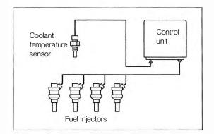
Fig. 5-1. Schematic of coolant temperature sensor used to adapt fuel system for warm-up enrichment. Injectors stay open longer when engine is cold based on cold engine signal from sensor.
