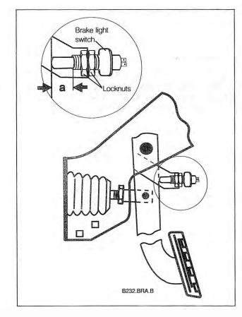
**Fig. 4-9.** Schematic of brake light switch. Adjust so that dimension **a** is  $5^{+0}_{-0}$ mm ( $0.2^{+0.4}_{-0.0}$ in.).
