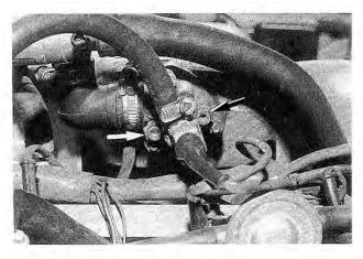
Fig. 5-8. Cold-start valve mounting screws (arrows).
