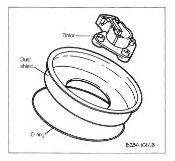
Fig. 5-10. Ignition rotor, distributor cap dust shield and O-ring.
