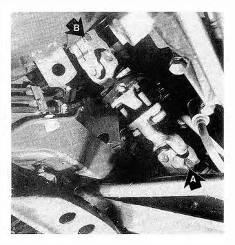
Fig. 7-14. Steering universal joint shaft with universal joints and rubber coupling. Lower bolt (A) fits in slot on steering gear pinion shaft and must be completely removed. Loosen upper bolt (B) to aid removal of universal joint shaft.
