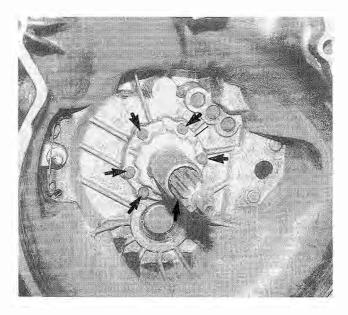
Fig. 7-46. Guide sleeve bolts (arrows) to be removed. Getrag 240 transmission shown.
