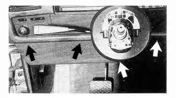
Fig. 7-6. Turn fasteners (arrows) 1/4 turn counterclockwise to release lower left-side instrument panel trim for access to instrument column.
