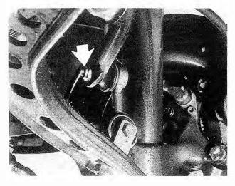
Fig. 5-14. Nut (arrow) fastens stabilizer bar to stabilizer-bar connecting link. Right (passenger) side shown.
