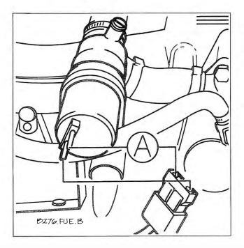
Fig. 6-18. Schematic view of ammeter connected to idle air stabilizer valve to measure current from control unit, on models with 2-wire valves (325e).
