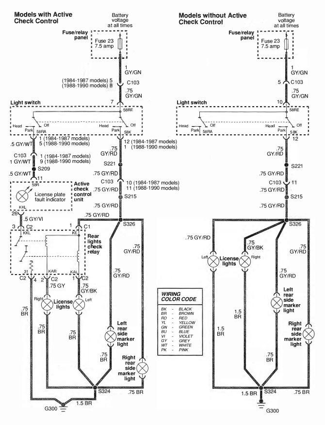
Fig. 10-7. License plate lights and rear side marker lights circuit.
