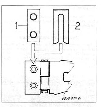
Fig. 5-4. Door hinge showing location of shims between hinge and door. Initial adjustment made with shim style 1. Fine adjustment made with shim style 2 (available in 1.0 mm or 0.5 mm thickness).
