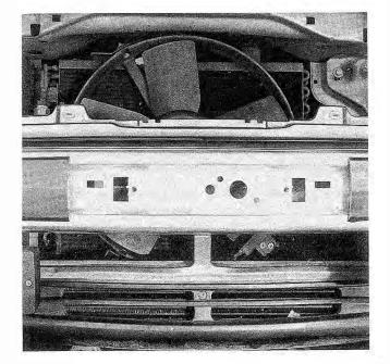
Fig. 4-20. Auxiliary cooling fan assembly viewed from front. Shown with grille removed for clarity.
