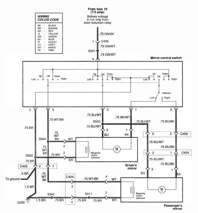
Fig. 12-6. Power mirrors circuit. Mirrors with single motor shown. Mirrors with dual motors are similar.
