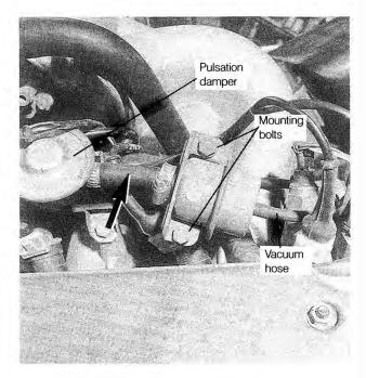
Fig. 5-23. Clamp shut fuel pressure regulator return hose at point indicated by arrow.
