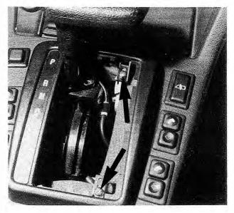
Fig. 4-6. Screws to be removed (arrows) for removal of shift lever trim panel.
