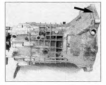
Fig. 3-9. Location (arrow) of transmission identification code for 5-speed manual transmission.
