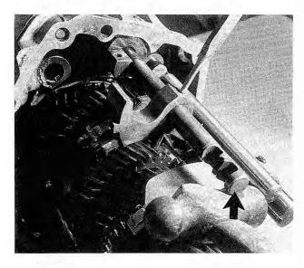
Fig. 7-9. Selector shaft operating lever rolled pin being driven in. Support end of shaft (arrow) while driving pin.
