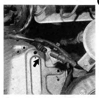
Fig. 5-2. Oxygen sensor connector (arrow) on 1986–1988 325i(is) models. Connectors on 325e(es) models and all 1989–1990 models are similar.
