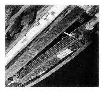
Fig. 7-10. Oil cooler mounting points (arrows).
