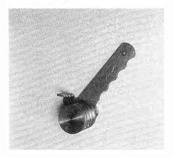
Fig. 4-2. Typical tube bender used to shape replacement brake lines.
