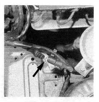
Fig. 5-14. Oxygen sensor connector disconnected (arrow). Types of connectors may vary between models.
