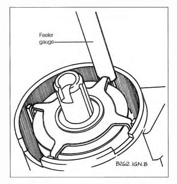
Fig. 4-4. Impulse generator air gap being checked with feeler gauge. Align trigger-wheel tab with impulse-generator tab as shown.
