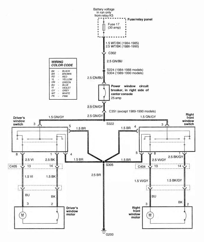
Fig. 12-5. Power window circuit for 2-door sedan models. Late 1986 through 1990 models use lighted switches (not shown).
