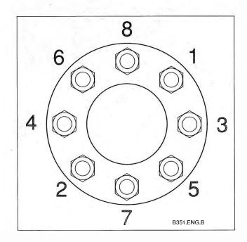
Fig. 6-10. Flywheel or drive plate mounting bolt tightening sequence.
