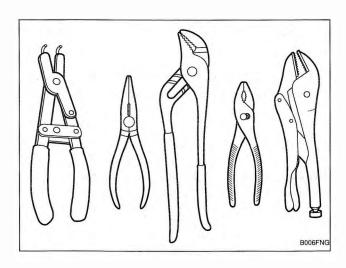
Fig. 4-6. Pliers. From left, snap-ring, needlenose, channel lock, common, locking.
