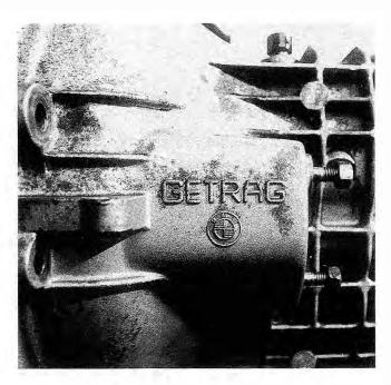
Fig. 3-8. Manufacturers stamp for Getrag manual transmissions. ZF transmissions are similar.
