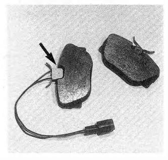
Fig. 4-11. Front left brake pads with brake pad wear sensor (arrow).
