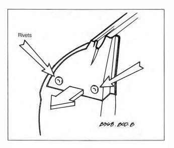
Fig. 5-18. Door trim and securing rivets (arrows) on convertible models.
