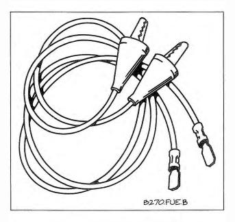
Fig. 4-15. Jumper wires with alligator clips. Flat connectors shown are for electrical testing at harness connectors.
