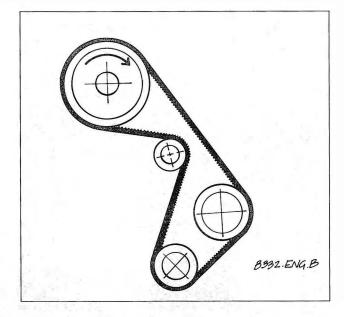
Fig. 4-6. Camshaft drive belt configuration with tensioner and sprockets. Arrow shows engine rotation direction.
