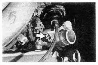
Fig. 3-5. Coolant temperature sender (brown/violet wire) on 4-cylinder engine (top arrow) and 6-cylinder engine (bottom arrow).
