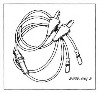
Fig. 5-19. Test leads made with flat connectors, alligator clips, and in-line fuse. Test leads used to make contact without spreading or damaging terminals in control unit connector.
