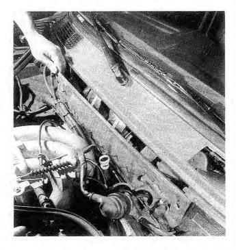
Fig. 4-30. Firewall access cover being removed.
