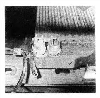
Fig. 4-21. Thermo-switches for radiator cooling fan lowspeed (left) and high-speed (right) on 4-cylinder engine (viewed from beneath).
