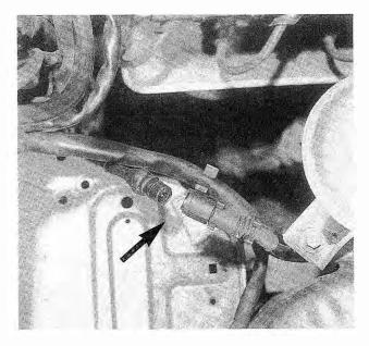
Fig. 6-29. Oxygen sensor harness connector (arrow).
