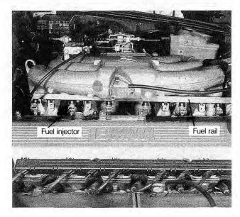
Fig. 4-27. Fuel rail is common fuel supply to injectors. Fuel rail from 325i model shown.
