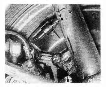
Fig. 5-2. Electrical connection at front strut for brake pad wear indicator (A). Internal-hex-head screw (B) secures ABS sensor.
