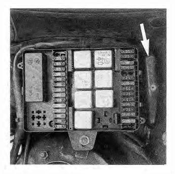
Fig. 5-17. Fuse/relay panel harness connector cover (arrow) on 1984 and 1985 models.
