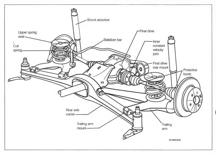
Fig. 1-2. Rear suspension assembly.
