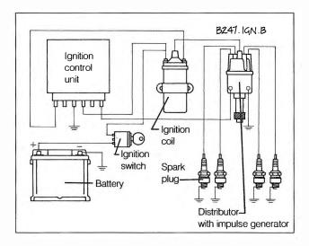
Fig. 1-1. Schematic representation of Transistorized Coil Ignition with impulse generator (TCI-i) installed on 4-cylinder engines.
