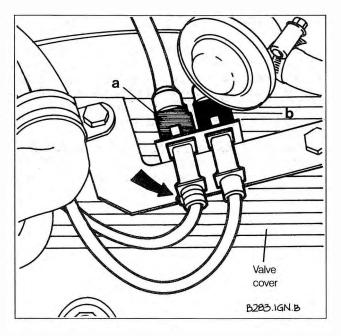
Fig. 5-4. Gray reference sensor connector (a) and black speed sensor connector (b) for 1984 and 1985 325e(es) engine. Reference sensor also marked with a ring (arrow).
