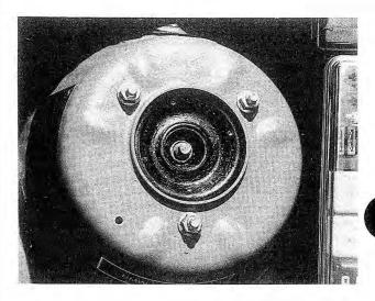
Fig. 5-6. Strut mounting nuts in engine compartment.
