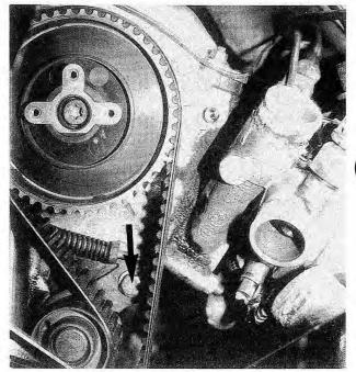
Fig. 4-13. Upper mounting bolt for camshaft drive belt ten-
