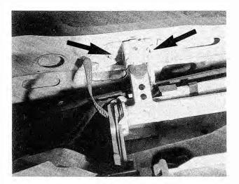
Fig. 6-20. Left-side hood mounting bolts (arrows). Remove bolts from right side also.
