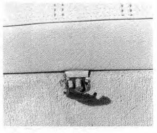
Fig. 4-40. Rear seat mounting bolt on seat with spring suspension. Remove bolts from both sides.
