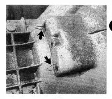
Fig. 5-10. Release lever retaining spring tabs (arrows). Squeeze tabs to remove spring
