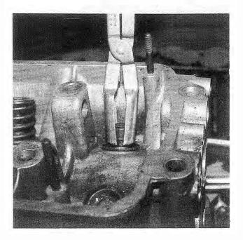
Fig. 4-42. Valve stem oil seal being removed from valve guide using special removal tool.
