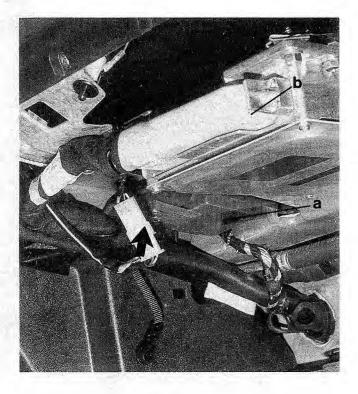
Fig. 5-2. Idle speed control unit (a) L-Jetronic control unit (b) harness connectors. White 3-point harness connector at arrow.
