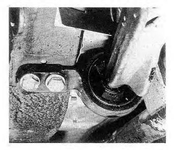
Fig. 5-13. Bracket for rubber bushing mounts to underbody with two bolts.
