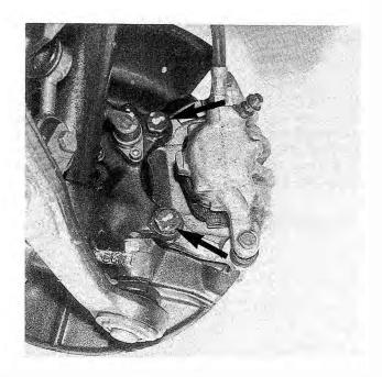
Fig. 5-11. Front brake caliper mounting bolts (arrows).
