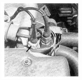
Fig. 5-11. Coolant temperature sensor (arrow). Remove connector and connect ohmmeter across sensor terminals to test.
