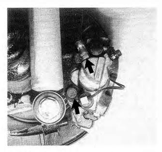
Fig. 7-7. Rear disc brake pad carrier mounting bolts (arrows).
