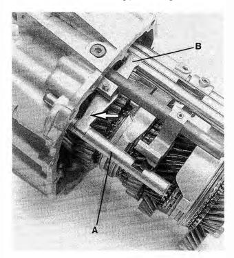
Fig. 7-19. Shift operating shaft (A) and shift operating lever(B) correctly installed in transmission. Groove in lever should be up and facing left (arrow).
