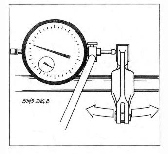
Fig. 4-34. Dial indicator being used to check rocker arm wear.
