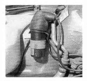
Fig. 5-1. Ignition coil with protective cover.
