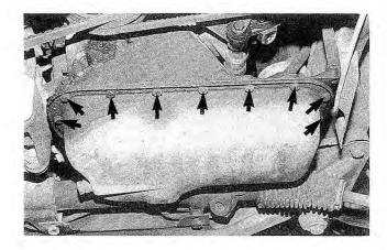
Fig. 7-6. Lower oil pan retaining bolts (arrows).
