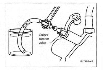
Fig. 4-1. Container (partially filled with brake fluid) connected to caliper bleeder valve with clear tubing for bleeding brakes. Bleeding rear drum brake wheel cylinder is similar.
