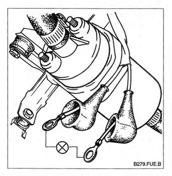
Fig. 4-13. Voltage supply to fuel pump being checked with test light (shown schematically). Externally mounted fuel pump shown.
