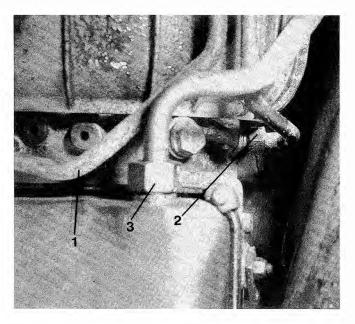
Fig. 5-1. ATF cooler lines for 4 HP 22 transmissions are at 1 and 2. ATF filler tube is at 3. Cooler lines on 3 HP 22 transmission are similar.
