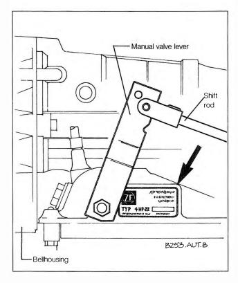
Fig. 1-4. Location (arrow) of automatic transmission data plate.
