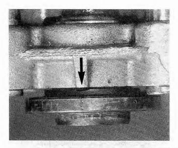
Fig. 4-31. Camshaft flange mark aligned with cast mark on cylinder head (arrow).
