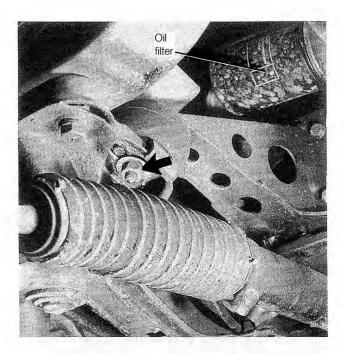
Fig. 5-12. Mounting nut for right engine mount (arrow) as viewed from beneath car. Left engine mount is similar.
