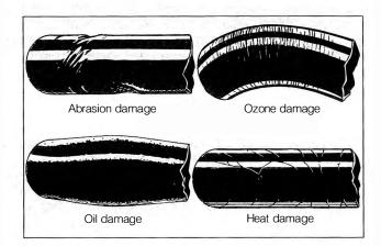
Fig. 6-6. Examples of damage to coolant hoses. Any of conditions shown is cause for replacement.
