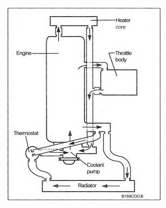
Fig. 1-1. Schematic view of cooling system components and hose routing showing coolant flow (arrows) for 4-cylinder engine.
