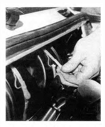
Fig. 4-31. Blower motor housing retaining straps being removed.
