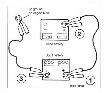
Fig. 6-1. Battery jumper cables connections. Numbers indicate correct sequence for cable attachment.
