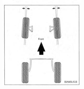
**Fig. 4-3.** Illustration of toe-in of front wheels. Toe angle is the measurement of how far the wheels point away from the direction of travel. The total toe specification is the sum of the toe angles of both wheels.
