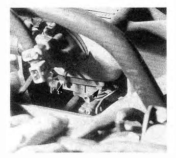
Fig. 5-6. Front throttle housing mounting nuts (arrows). Rear mounting nuts not visible.
