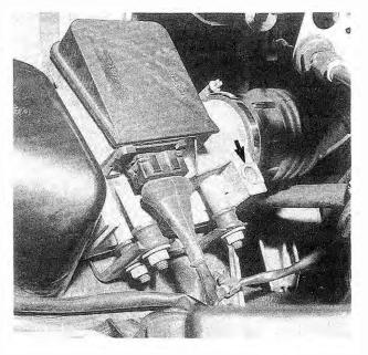
Fig. 5-24. Idle mixture adjusting screw in corner of air flow sensor (arrow).
