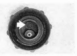
Fig. 3-4. Inside of radiator cap showing location of vacuum valve (arrow).
