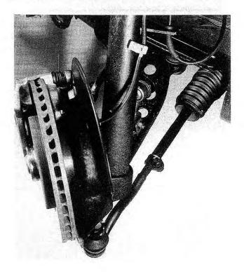
Fig. 4-6. Tie rod end and rubber boot shown in correct position (not twisted).
