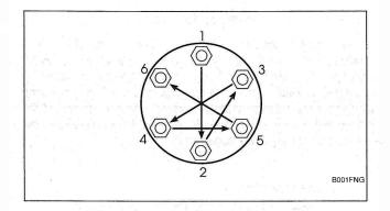
Fig. 3-2. Sequence for alternately tightening multiple fasteners.
