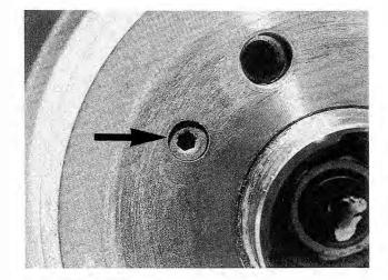
Fig. 7-8. Rear rotor mounting screw (arrow).
