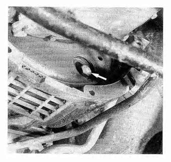
Fig. 5-3. Torque converter mounting bolt (arrow). Rotate torque converter for access to all bolts.
