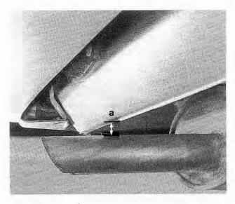
Fig. 4-5. Clearance (a) between tailpipe and body.
