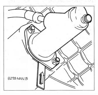
Fig. 5-3. Slave cylinder pushrod travel being checked with metal strip.
