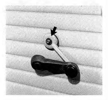
Fig. 5-8. Window crank and mounting screw (arrow). Trim and crank may differ slightly on other models.
