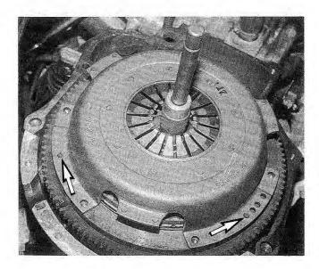
Fig. 5-14. Pressure plate guide pins (arrows). Note use of pilot tool to align clutch disc.
