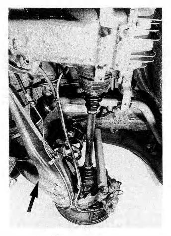
Fig. 6-12. Rear suspension trailing arm (arrow) installed position.
