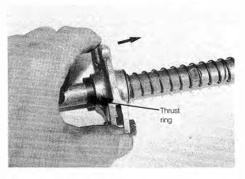
Fig. 4-35. Remove rocker arm retainer (snap ring) by sliding rocker arm and thrust ring in (arrow) and prying off snap ring.
