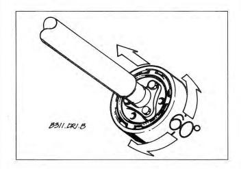
Fig. 4-6. On models with vibration damper, turn damper 60° in either direction before pulling driveshaft off transmission flange.
