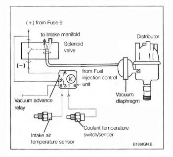
Fig. 4-16. Schematic view of vacuum advance system. Vacuum is switched on and off at solenoid valve by the electronic relay.
