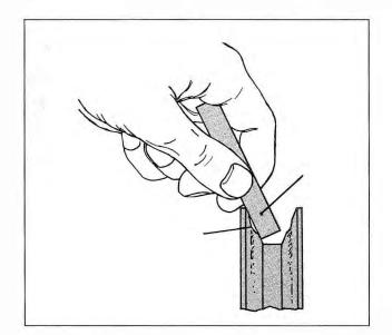
Fig. 6-4. V-belt pulley being checked for wear using a straight edge. A worn pulley may be the cause of a noisy belt, especially if the belt is new.
