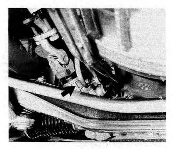
Fig. 7-2. Power steering control valve (arrow) is part of steering gear. Universal joint shaft connects steering column to steering gear pinion at control valve.
