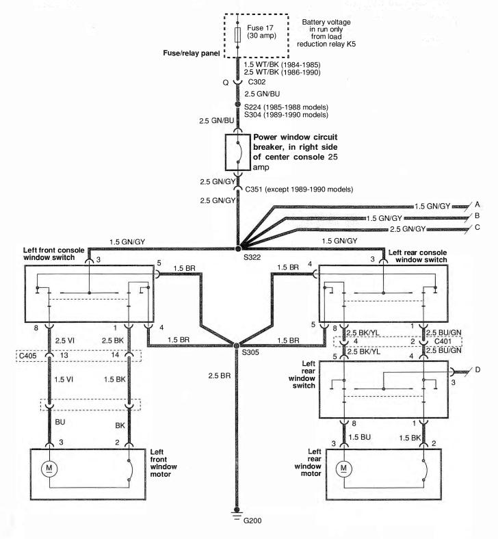
Fig. 12-4. Power window circuit for 4-door sedan and convertible models. Late 1986 through 1990 models use lighted switches (not shown). Circuit on convertible model may vary slightly. (continued on next page)
