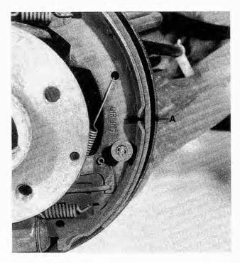
Fig. 7-3. Rear brake lining thickness being checked after brake drum is removed. Dimension A shows minimum brake lining thickness.
