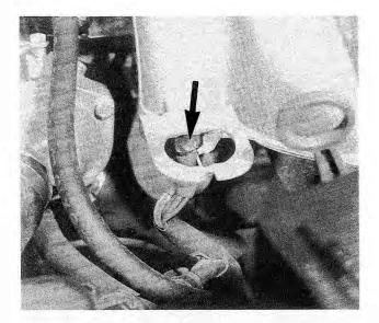
Fig. 3-10. Ground point G103 (arrow) on 325, 325e, and 325es models with 2.7 eta engine (left side of engine, beneath diagnostic connector).
