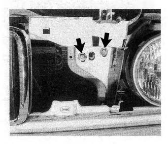
Fig. 6-24. Hood lock mounting bolts (arrows).
