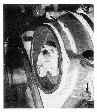
Fig. 4-8. Upper camshaft drive belt cover mounting bolts (arrows).
