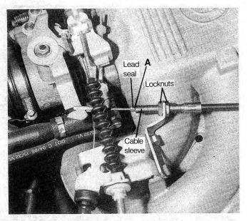
Fig. 4-7. Transmission accelerator cable adjustment point. Check distance A at idle and at kickdown position. Six-cylinder shown. Four-cylinder models are similar.
