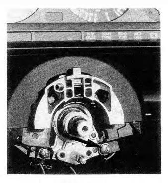
Fig. 8-4. Location of ground wire for wiper/washer switch (arrow).
