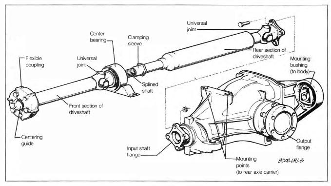
Fig. 1-1. Driveshaft and final drive assemblies.
