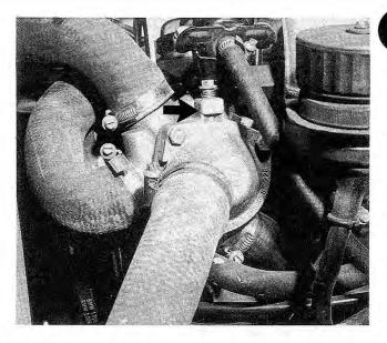
Fig. 4-4. Location of bleeder screw on thermostat housing of 6-cylinder engine (arrow).
