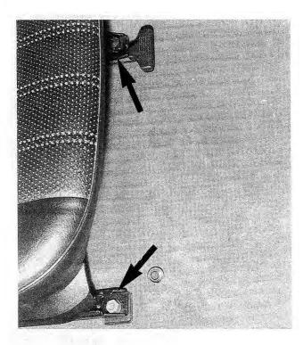
Fig. 4-39. Front-seat mounting nuts at front of seat rails (arrows). One nut cover is shown removed. Also remove two nuts at rear of seat rails.
