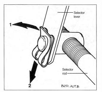
Fig. 4-3. Selector rod being disconnected from bottom of lower selector lever. Lift tab of retaining clip (direction 1) and slide clip off (direction 2).
