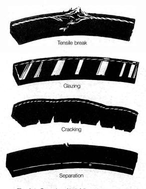
Fig. 6-1. Examples of belt failure.
