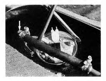
Fig. 4-4. Transfer pump output hose disconnected and plugged (arrow).
