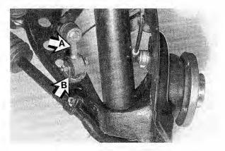
Fig. 5-22. Stabilizer bar connecting link (A) and control arm mounting bracket (B). Left (driver's) side shown.
