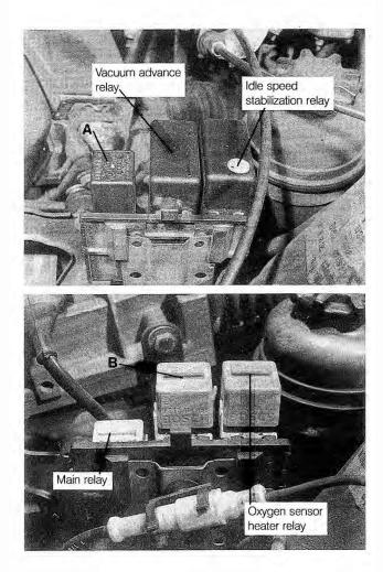
Fig. 4-2. Fuel pump relay location on 4-cylinder engine (A) and 6-cylinder engine (B).
