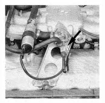
Fig. 6-10. Cold-start valve (arrow) controlled by thermo-time switch is used to provide extra fuel for cold starting.
