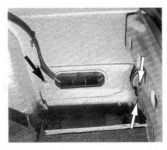
Fig. 6-18. Mounting nuts and bolt inside trunk (arrows) for right rear side piece on three-piece bumpers. Left side is similar. Additional mounting bolt and nut are at rear edge of wheel housing.
