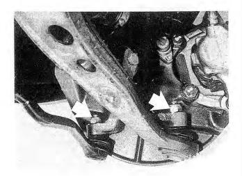
Fig. 5-5. Self-locking nuts (arrows) secure the control arm to the strut housing and the tie rod to the steering arm.
