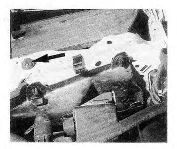
Fig. 6-21. Hood stop (arrow). Screw stops all the way in on both sides before making any hood adjustments.
