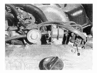
Fig. 5-7. Cold-start valve (A) and thermo-time switch (B) used to provide extra fuel for cold starting. Thermotime switch has brown connector.
