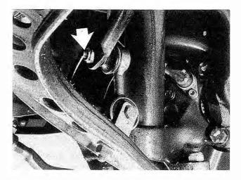
Fig. 5-20. Nut (arrow) fastens stabilizer bar to stabilizer bar connecting link. Right (passenger) side shown.
