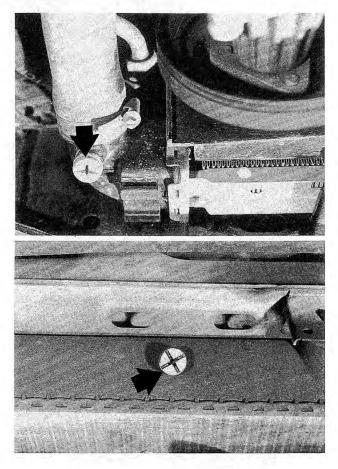
Fig. 4-1. Location of radiator drain plug on 6-cylinder engine (top arrow) and 4-cylinder engine (bottom arrow).
