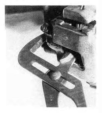
Fig. 5-6. Water pump pliers being used to carefully push piston into caliper.
