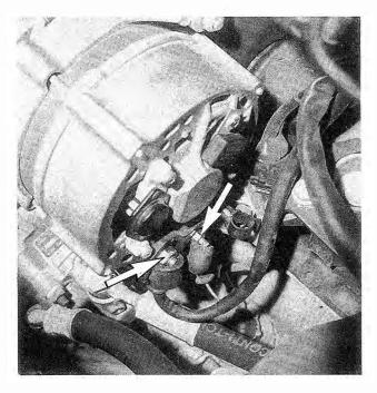
Fig. 5-2. Alternator wiring mounting nuts and wiring on models with 6-cylinder engine (arrows). Models with 4-cylinder engine have additional ground wire.
