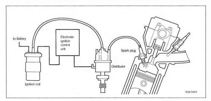
Fig. 1-3. Schematic representation of basic ignition system.
