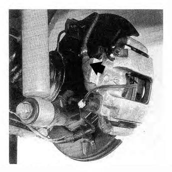
Fig. 7-15. Rear brake caliper brake hose fitting (arrow).
