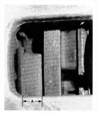
Fig. 7-2. Disc brake pad wear being checked through opening in caliper. Minimum brake pad thickness shown by dimension **A**.
