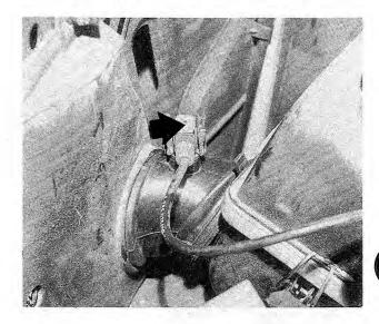
Fig. 5-4. Intake air temperature sensor (arrow).
