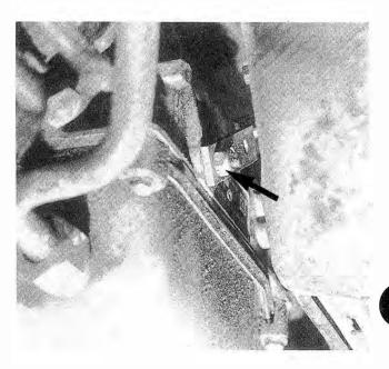
Fig. 5-8. Manual valve lever and nut on transmission to be removed for replacement of seal.
