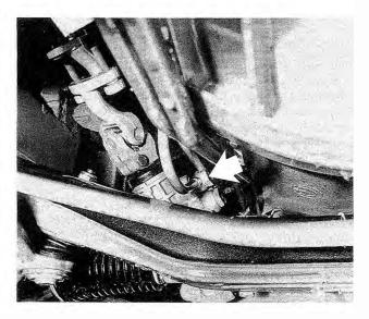
Fig. 7-15. Power steering pressure line connection (arrow) at steering control valve.
