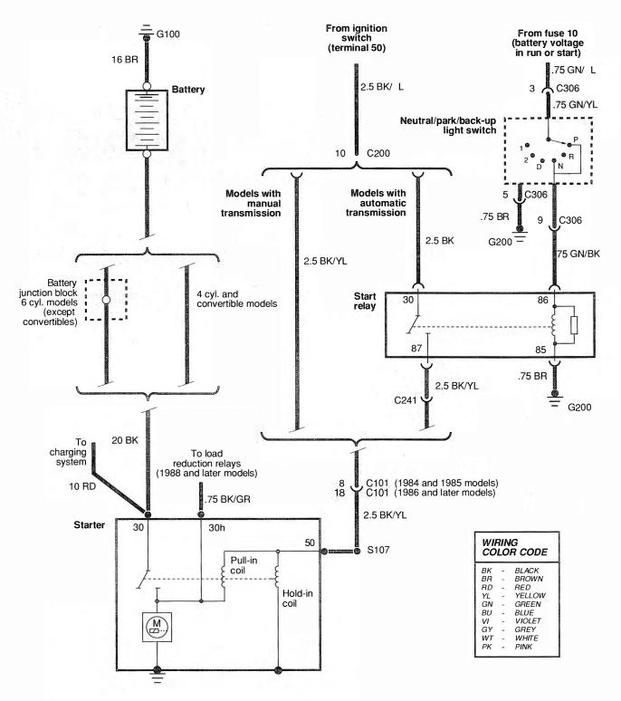
Fig. 6-1. Starting system circuit diagram. Circuit may vary slightly on some models.
