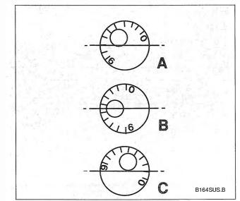
Fig. 6-17. Examples of matching eccentric bushing installation marks to imaginary reference line. A is set at "7". B is set at "4½" (maximum correction). C is set at "1".
