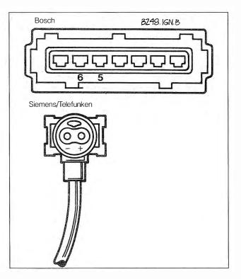
Fig. 4-3. Ignition control unit connectors and terminals used to check impulse generator resistance.
