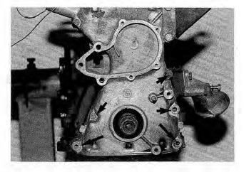
Fig. 4-20. Lower timing chain cover mounting bolts (arrows).
