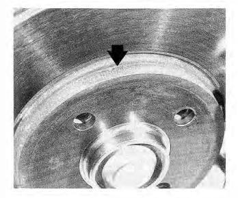
Fig. 5-9. Front rotor minimum dimension stamped on rotor hub (arrow).
