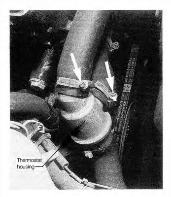
Fig. 4-9. Location of hose clamps (arrows) and thermostat housing on 4-cylinder engine.
