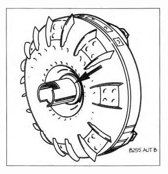
Fig. 5-6. Torque converter removed from engine showing bearing surface (arrow) that should be checked for scoring or wear.
