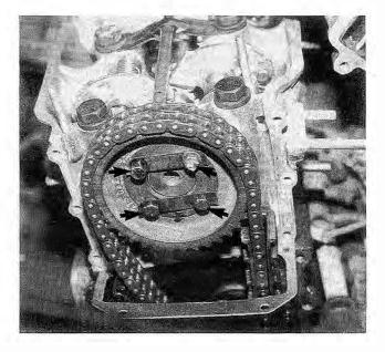
Fig. 4-21. Camshaft drive sprocket mounting bolts (arrows). Sprocket shown with locking tabs.
