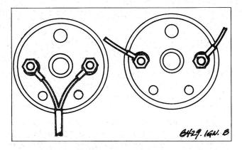
Fig. 3-4. Coil wiring correctly positioned (left) and incorrectly positioned (right). Wires terminals should not touch or come close to metal coil housing.
