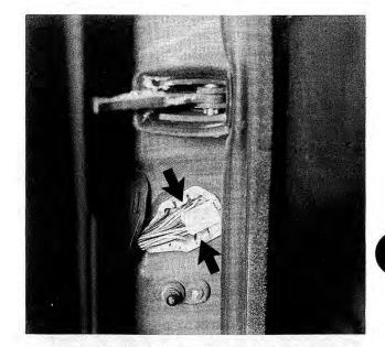
Fig. 5-3. Door wiring connector (arrow) for front doors.
