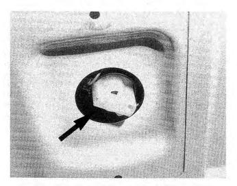
Fig. 4-18. Center stop light housing (arrow) in trunk, for 1988 and later models. Stop light for 1987 and earlier models is reached from inside passenger compartment.
