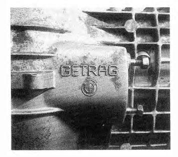
Fig. 1-3. Manufacturer's stamp for Getrag transmissions. ZF transmissions are similar.
