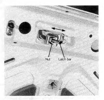
Fig. 6-26. Trunk lid latch. To adjust, turn nut to move latch bar in or out (arrows).
