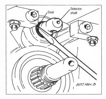
Fig. 7-45. Selector shaft oil seal being pried out with screwdriver. Take care not to scratch selector shaft.
