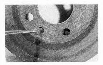
Fig. 6-2. Rear drum brake mounting screw being removed. Brake drum shown removed for clarity.
