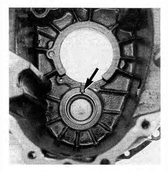
Fig. 7-49. Layshaft bearing shell correctly installed in front case, with oil passage aligned with hole in case (arrow).
