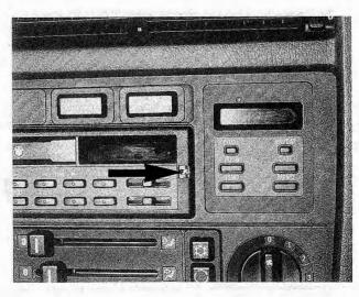
Fig. 4-13. Access hole (arrow) for internal-hex head screw used to retract retaining clip on late model BMW radios.
