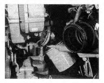
Fig. 4-4. Engine oil filter located in left-hand (driver's) side of engine. Air Filter housing shown removed from car.
