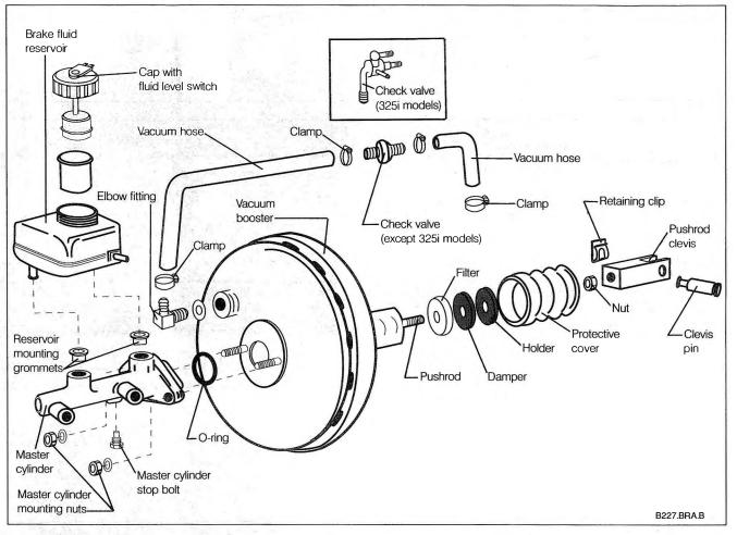
Fig. 4-3. Master cylinder and vacuum booster assembly.
