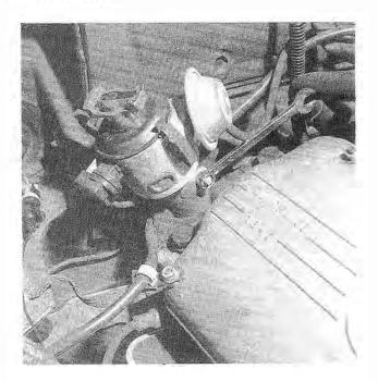
Fig. 4-9. Distributor clamping nut being loosened.
