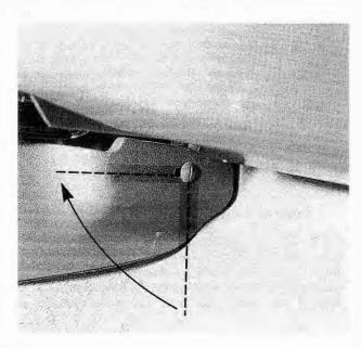
Fig. 4-10. Console retainer. To unlock, turn 90° (1/4 turn) counterclockwise. Remove retainers from both sides.
