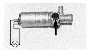
Fig. 6-15. Schematic view of battery voltage being applied to idle air stabilizer valve. Valve piston (arrow) should close when voltage is applied.
