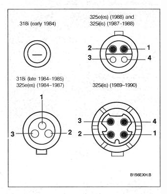
Fig. 5-3. Identification of terminals at oxygen sensor harness connectors. Wiring harness side shown. Terminals are also identified on connector.
