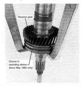
Fig. 7-37. Reverse gear assembly being installed on output shaft.
