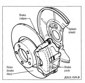
Fig. 1-7. Disc brake assembly showing disc, caliper, and splash shield. Caliper assembly holds pads with friction material.
