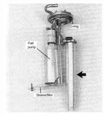
Fig. 4-18. Fuel pump assembly. Fuel gauge sending unit shown removed from assembly (arrow).
