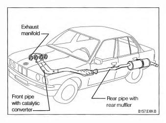
Fig. 1-1. Typical two-piece BMW 3-series exhaust system. Exact configuration varies from model to model.
