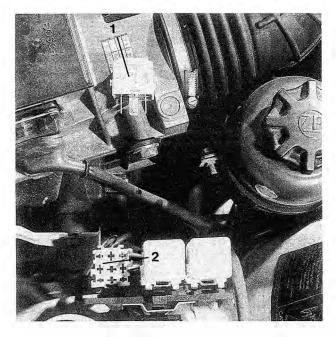
Fig. 6-24. Main relay (1) removed from relay socket (2).
