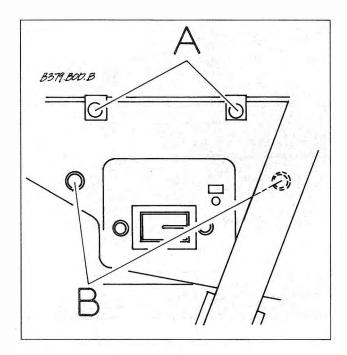
Fig. 5-16. Convertible rear window regulator mounting screws (B). Screws at A do not apply to this procedure.
