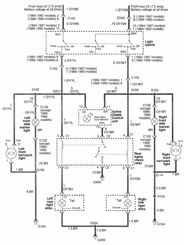
Fig. 10-8. Parking lights, front side marker lights, and taillights circuit. Circuit may vary slightly on some models. (continued on next page)
