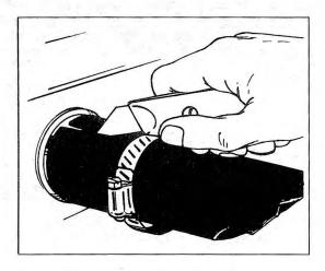
Fig. 4-5. Stuck hose being removed by cutting.
