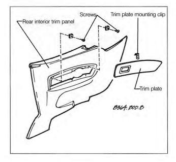
Fig. 4-36. Exploded view of rear interior trim panel on convertible models. Trim panel must be removed for access to upper anchor for front seat belt.
