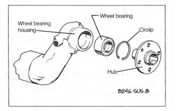
Fig. 6-19. Trailing arm wheel bearing housing, hub, and wheel bearing. Hub is driven out from behind after removing drive axle and outer CV joint. Bearing is pressed out after removing circlip from wheel bearing housing.
