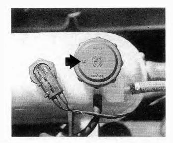
Fig. 3-3. Expansion tank cap (6-cylinder engine) showing opening pressure specification (arrow).
