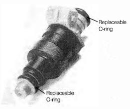
Fig. 4-26. Electric fuel injector. O-rings seal injector to intake manifold and fuel rail.
