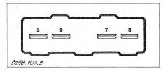
Fig. 5-4. Air flow sensor terminal identification used for testing potentiometer.
