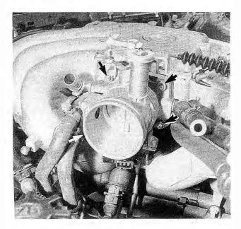
Fig. 6-9. Throttle housing mounting bolts (arrows).
