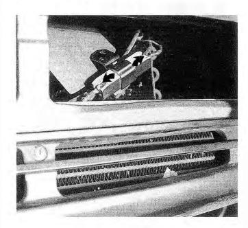
Fig. 4-23. Auxiliary cooling fan low speed resistor and electrical connectors (arrows). Resistor shown removed from fan housing for clarity.
