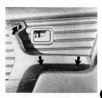
Fig. 5-9. Front armrest screws to be removed (arrows). Upper screw is behind trim piece or power mirror switch, which should be pried out.
