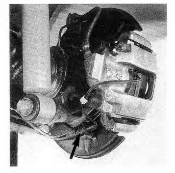
Fig. 7-2. Brake pad wear sensor connector for right-rear wheel (arrow).
