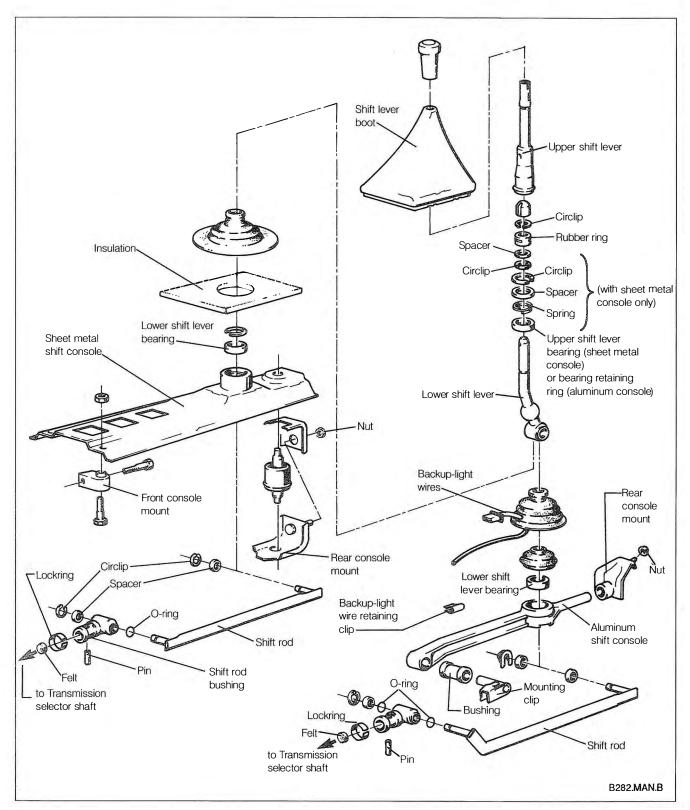
Fig. 4-1. Exploded view of shift mechanism.
