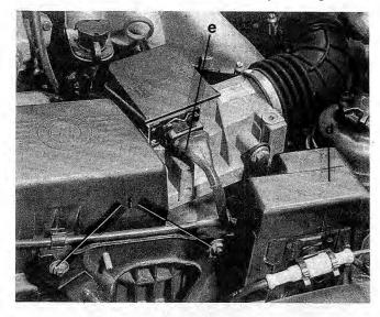
Fig. 5-19. Auxiliary relay panel (d), air flow sensor connector (e), air filter mounting nuts (f).
