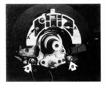
Fig. 7-8. Screws fasten steering column switches (A) and ground wires (B).
