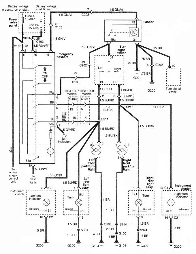
Fig. 10-4. Turn signal and emergency flashers circuit.
