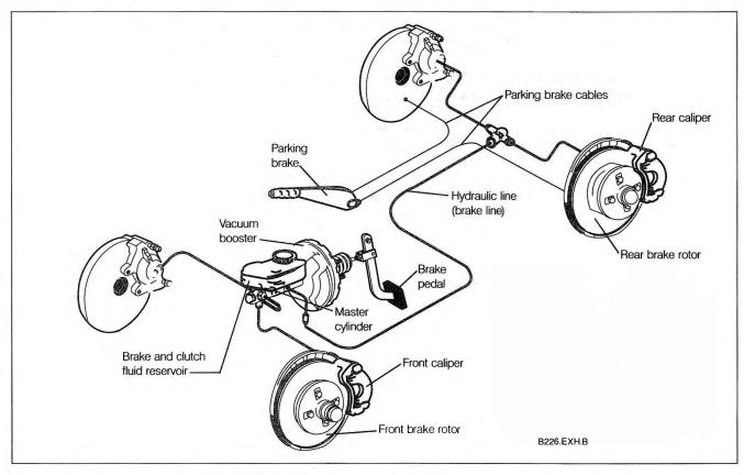
Fig. 1-1. Schematic view of dual-circuit brakes. Four-wheel disc brakes shown. Front disc and rear drum system is similar.
