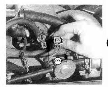
Fig. 5-10. Schematic view of test light connected across cold-start valve harness connector.
