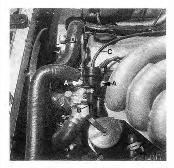
Fig. 6-27. Fuel pressure regulator mounting bolts (A), return fuel line (B), and vacuum line (C).
