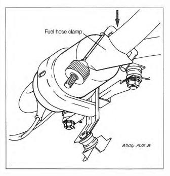
Fig. 4-15. Fuel pump inlet hose being pinched shut (arrow) with special clamp.
