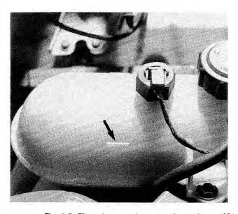
Fig. 6-5. Fill mark on coolant expansion tank on 1984 through 1987 6-cylinder engine (arrow). Expansion tank on 1988 and later models is slightly different. Coolant level should be at mark when engine is cold.
