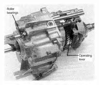
Fig. 7-18. Selector shaft with roller bearings being installed.
