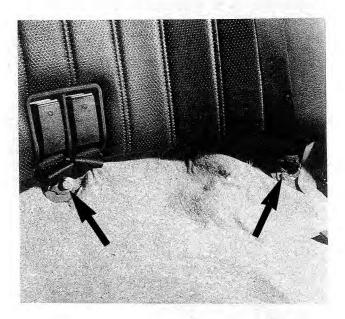
Fig. 4-37. Rear seat belt anchor bolts (arrows).
