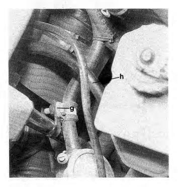
Fig. 5-6. Coolant hose clamp on intake manifold bracket (g) and charcoal canister vacuum hose (h).
