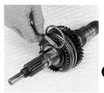
Fig. 7-39. 5th/reverse gear guide sleeve axial play being measured.
