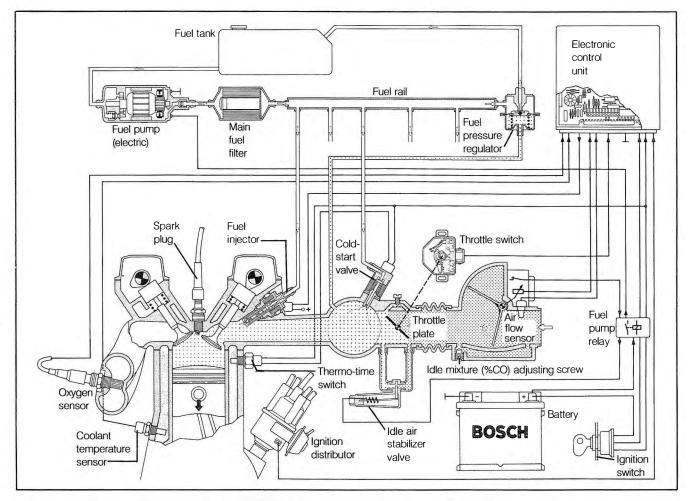
Fig. 1-1. Schematic of L-Jetronic System used on the 4cylinder (318i) engines. Courtesy Robert Bosch Corp.
