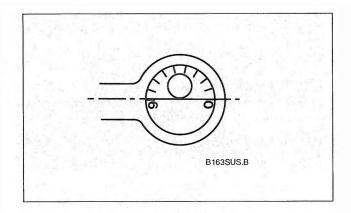
Fig. 6-16. Installed angle of eccentric bushing (which determines amount of toe correction) is measured from imaginary reference line (parallel to trailing arm as shown).
