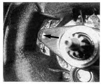
Fig. 5-16. Installed position of release lever. Note location of retaining clip (arrow).
