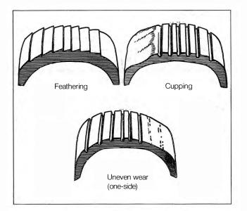
Fig. 3-4. Examples of uneven tread wear caused by misalignment and/or worn or damaged components. Feathering suggests incorrect alignment. Uneven wear on one side suggests incorrect alignment or repeated hard cornering. Cupping results from vibration, often caused by unbalanced tire or faulty shock absorber. Drawings courtesy of Goodyear Tire and Rubber Co.
