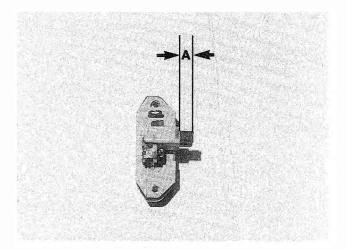
Fig. 5-3. Alternator brush length being checked. Length A of new brushes is 12 mm (15/32 in.). Replace brushes worn to 5 mm (7/32 in.) or less.
