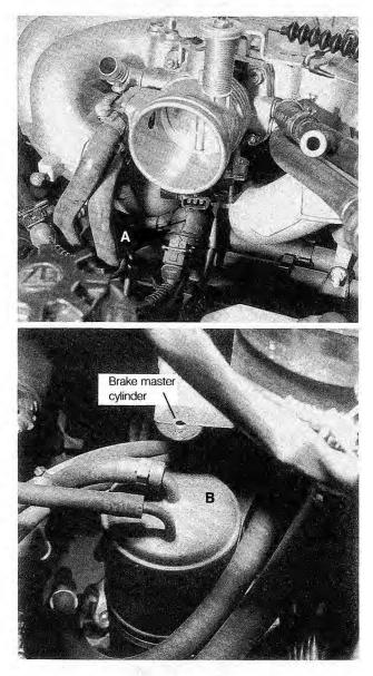
Fig. 4-21. Charcoal canister bypass valve (A) and charcoal canister (B) used with Motronic 1.1 engine management System.
