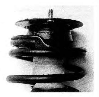
Fig. 5-7. Correct assembly of coil spring, rubber ring, and spring retainer.
