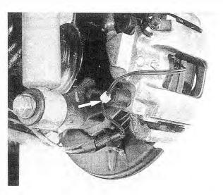
Fig. 7-6. Rear brake pad wear sensor shown correctly routed through clip (arrow).
