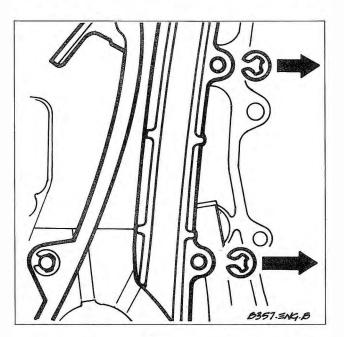
Fig. 4-22. Camshaft timing chain guide rail mounting circlips. Remove circlips in direction of arrows.
