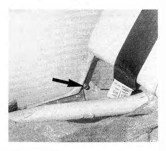
Fig. 4-41. Rear seat backrest mounting bolt (arrow). There is one on each side. On some models, bolts may be at center of backrest.
