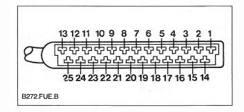
Fig. 5-17. Terminal identification for 25-point L-Jetronic control unit connector.
