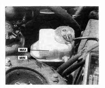
Fig. 7-1. Level indicators on brake fluid reservoir. Correct level is between MIN and MAX marks.
