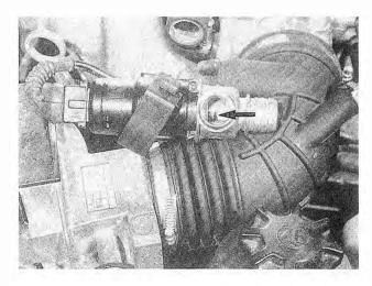
Fig. 6-16. Idle air stabilizer valve piston (arrow) in center position with harness connector connected and ignition on.
