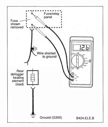
Fig. 3-5. Voltmeter being used to check for a short circuit to ground.
