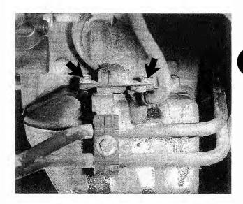
Fig. 7-5. Oil level sensor mounting nuts (arrows). Oil level sensor wiring harness can be separated at connector near bottom of alternator.
