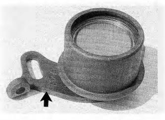
Fig. 4-7. Camshaft drive belt tensioner with stamp "Z 127" (arrow).
