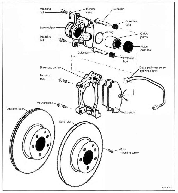
Fig. 5-1. Exploded view of front disc brake assembly.
