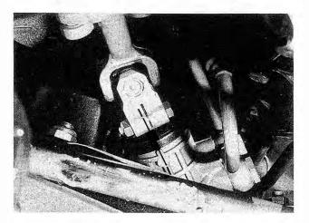
Fig. 7-5. Marks on steering gear housing align as shown when steering gear is centered and front wheels are in straight-ahead position.
