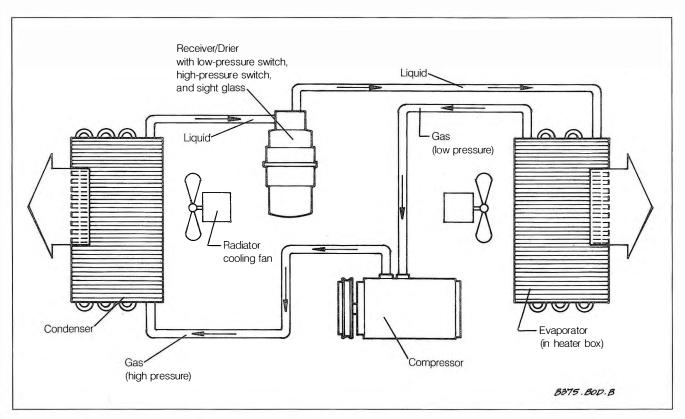
Fig. 9-1. View of typical BMW air conditioning system.
