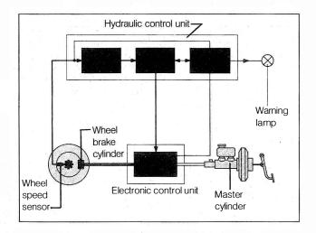
Fig. 1-2. Schematic representation of the ABS system used on cars covered by this manual.
