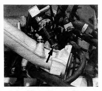
Fig. 3-5. Injector seals or O-rings (arrow) are a common source of air leaks, especially on high mileage engines. Injectors must first be removed to replace seals.
