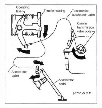
Fig. 4-1. Accelerator cable and transmission accelerator cable layout. Arrows show movement of operating lever and transmission cable when accelerator pedal is depressed.
