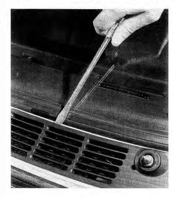
Fig. 8-6. Ventilation grill being removed from body. Wrap tip of screwdriver with tape to protect paint.
