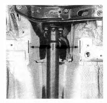
Fig. 4-1. Driveshaft side-to-side alignment. Driveshaft should be centered between the edges of the drive-shaft tunnel as shown.
