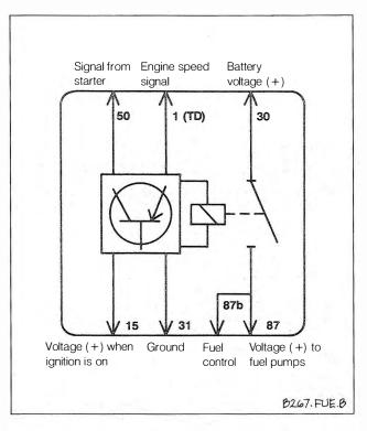
Fig. 4-10. Schematic view of fuel pump relay and circuits on models with 4-cylinder engine.
