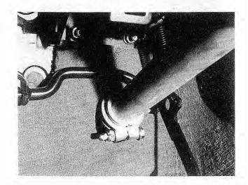
Fig. 7-3. Firewall mounting point for steering column housing. Clamp attaches steering column housing to firewall mount.
