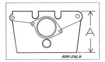
Fig. 4-66. Front view of cylinder head showing minimum resurfacing dimension (A). 6-cylinder engine shown.
