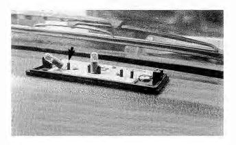
Fig. 6-9. Disconnected bulb terminal (arrow) of oxygen sensor warning light.
