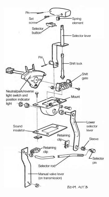
Fig. 4-2. Exploded view of automatic transmission selector lever and linkage.
