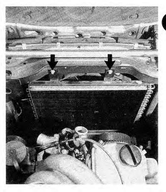
Fig. 4-25. Air conditioning condenser mounting bolts (arrows).
