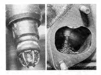
Fig. 3-1. Examples of carbon deposits on fuel injector (left) and intake valve (right). Carbon deposits can cause a rough idle, hard cold starting, and overall poor performance. Driving style is thought to be the main contributor to the problem. A car that is predominantly driven on short trips around town or in city traffic seems to increase the likelihood of deposits forming.
