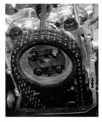
Fig. 4-26. Apply enough sealer to fill bores (arrows).
