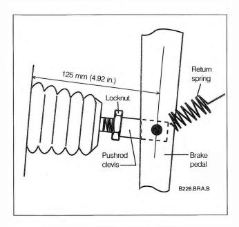
Fig. 4-7. Basic brake pedal pushrod adjustment as viewed from side.
