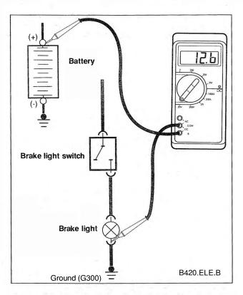
Fig. 3-2. Voltmeter being used to check for ground.
