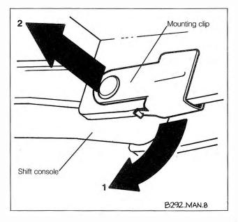
Fig. 4-9. Front mounting clip for aluminum shift console. Remove by first unclipping (1), and then sliding pin and clip out (2).
