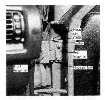
Fig. 5-1. Top hinge on front door, showing mounting hardware. Bottom hinge is similar, except mounting bolt installs from top.
