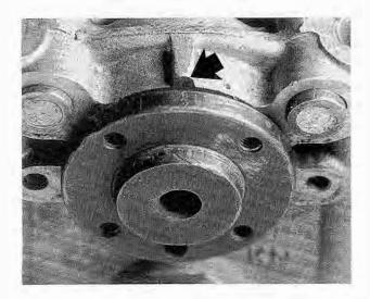
Fig. 4-23. Notch in camshaft flange aligned with mark on cylinder head (arrow).
