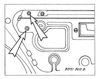
Fig. 5-20. Securing screws (arrows) for rear window frame.
