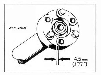
Fig. 4-13. When installing new driveshaft centering guide, check protrusion of guide as shown.
