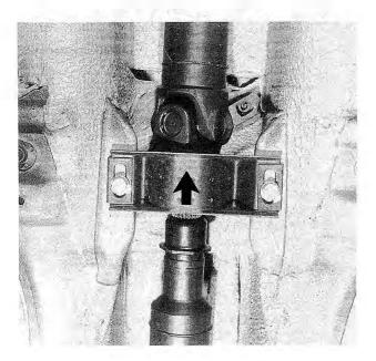
Fig. 4-8. Before tightening bolts, push center bearing towards the front (arrow) to preload it.
