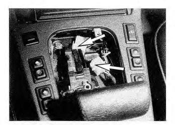
Fig. 10-6. Location of neutral/park/back-up light switch on cars with automatic transmission. Switch harness connector (C306) shown at arrow.
