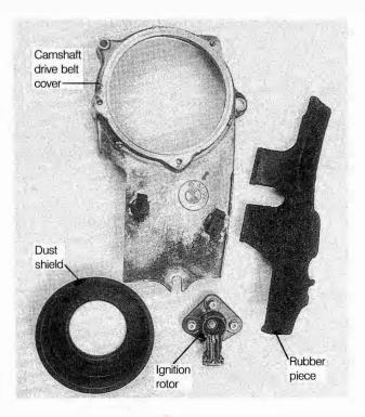
Fig. 4-14. Camshaft drive belt cover and rubber piece shown removed. Dust shield and ignition rotor also shown.
