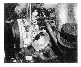
Fig. 4-7. 6-cylinder coolant outlet (on cylinder head) with thermostat housing, thermostat, and O-ring removed.
