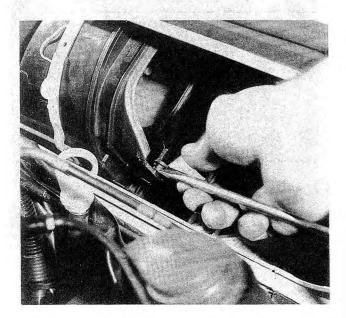
Fig. 4-34. Air recirculation flap being disengaged from blower motor housing. Disengage both sides.
