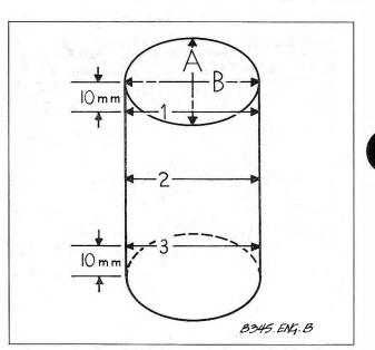
Fig. 6-6. Cylinder bore measuring points. Top (1) and bottom
