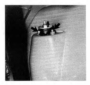
Fig. 6-2. Rear shock absorber upper mounting nuts (arrows) in trunk. Shown with trim partially removed for access.
