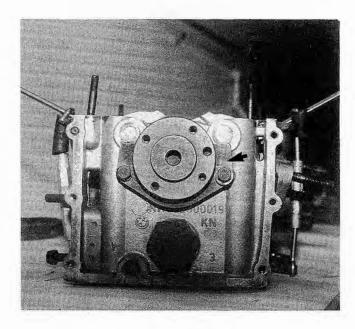
Fig. 4-29. Camshaft thrust plate (arrow).
