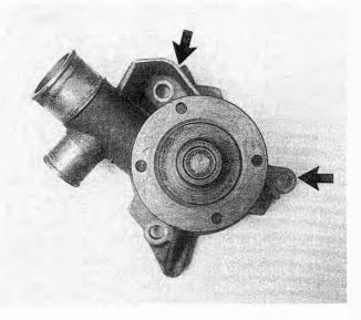
Fig. 4-15. Locations of coolant pump mounting bolts (arrows) which must be removed first.
