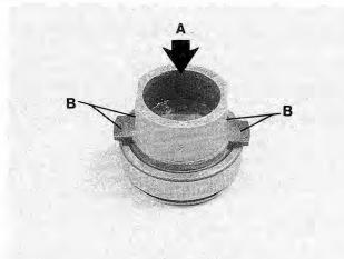
Fig. 5-15. Release bearing lubricating groove (A) and guides (B) to be greased.
