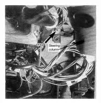
Fig. 7-2. Main ground connection for instrument cluster (arrow). Lower instrument panel trim removed.
