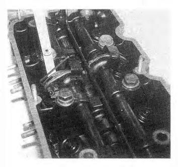
Fig. 4-27. Valve clearance being measured. Feeler gauge is inserted between rocker arm eccentric and valve.
