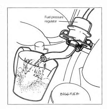
Fig. 4-9. Container being used to measure fuel delivery rate at output side of pressure regulator. Pressure regulator is mounted at end of fuel rail in engine compartment.
