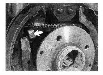
Fig. 6-6. Parking brake cable disconnected from attachment point (arrow) on rear shoe.
