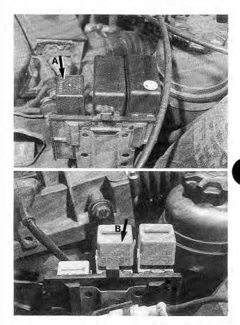
Fig. 4-12. Fuel pump relay location on 4-cylinder engines (A) and 6-cylinder engines (B).
