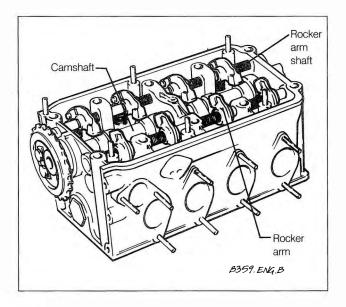
Fig. 1-1. Cylinder head and valve train for models with 4cylinder engine. Cylinder head for models with 6cylinder engine is similar.
