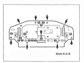
Fig. 7-3. Instrument cluster viewed from rear showing cover mounting screws (arrows).
