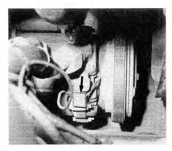
Fig. 11-1. Typical location of air conditioning compressor in-line diode (arrow).
