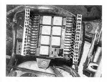
Fig. 14-3. Fuse/relay panel showing fuse locations.
