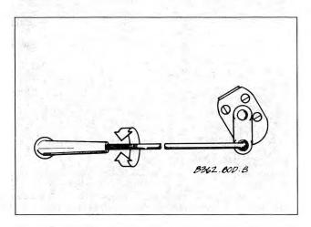
Fig. 4-28. Air recirculation flap control rod and motor. Adjust flap by unscrewing motor and turning to change length of rod.
