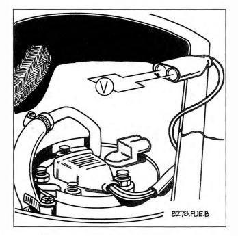
Fig. 4-3. Schematic view of voltage supply to transfer pump being checked at harness connector.
