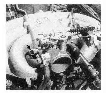
Fig. 6-7. Throttle housing, showing intake duct removed, and hose removed from idle air stabilizer valve (arrow).
