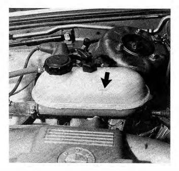
Fig. 4-3. Fill mark on coolant expansion tank on 6-cylinder engine (arrow). Coolant level should be at mark when engine is cold.
