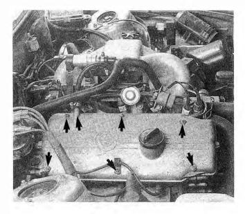
Fig. 4-1. Cylinder head cover mounting nuts, bolt, and breather hose (arrows).
