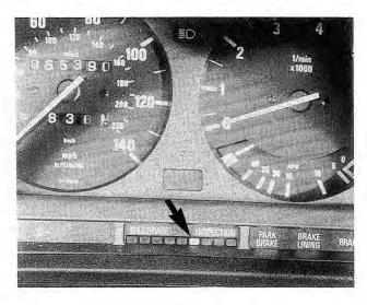
Fig. 2-1. Service indicator display in instrument panel (arrow).
