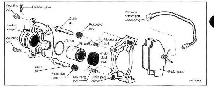
Fig. 5-10. Exploded view of front disc brake caliper.
