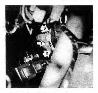
Fig. 4-22. Heater valve clamp (1) and flange bolts (2).
