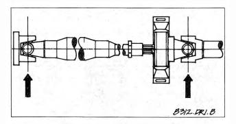
Fig. 4-7. If driveshaft sections are separated, make sure U-joints are on same plane as shown when driveshaft is reassembled.
