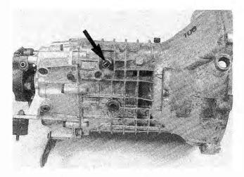
Fig. 10-5. Location of back-up light switch on manual transmission housing (arrow).
