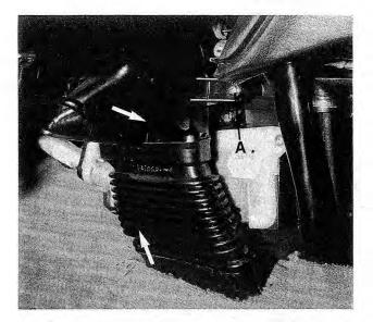
Fig. 4-21. Heater ducts (arrows). Remove screw (A) then gently pry out ducts.
