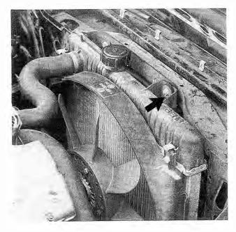
Fig. 4-29. Radiator mounting nut on cars with 4-cylinder engine (arrow).
