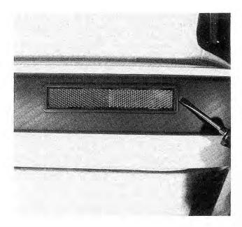
Fig. 6-8. Side marker lens being removed. Use screwdriver to pry at front of housing.
