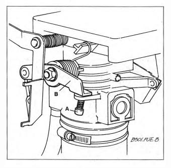
Fig. 5-5. Throttle adjusting screw with tamper-proof cap (A) and throttle lever (B).
