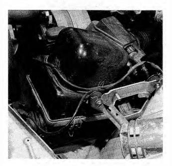
Fig. 5-1. Air filter housing in front left (driver's) side of engine compartment. Loosen nuts and unclip spring clips (arrows) to remove air filter.
