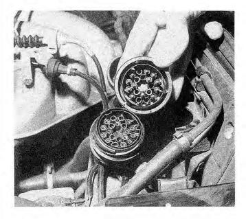
Fig. 5-18. Main harness connector separated on 1986 and later models.
