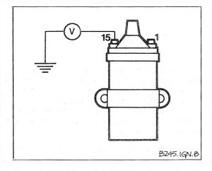
Fig. 3-1. Primary voltage to coil being checked with a voltmeter (shown schematically) between terminal 15 and ground. Coil terminal numbers are found on coil.
