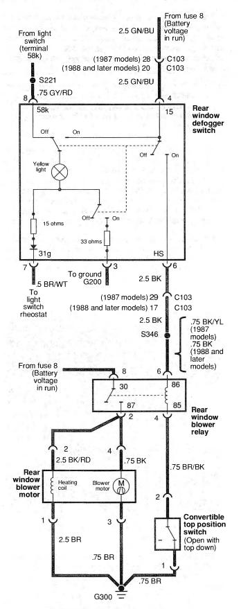
Fig. 11-6. Rear window defogger circuit for convertible models.
