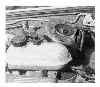
Fig. 3-11. Ground point G103 (arrow) on 325i models with 2.5i engine (on right shock tower).
