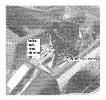
Fig. 6-11. Parking brake lever assembly showing cable connections and adjustment points.
