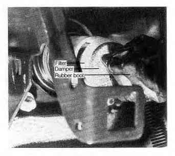
Fig. 4-6. Vacuum booster foam filter and damper as viewed from inside passenger compartment. (Rubber boot turned inside out for clarity.)
