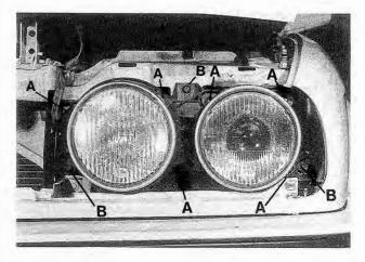
Fig. 6-2. Headlight assembly for models with two-piece halogen lights with replaceable bulb. Lensassembly retaining clips are at **A**. Headlight housing retaining screws for all models are at **B**.
