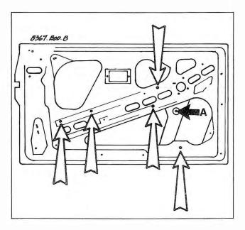
**Fig. 8-6.** Window stop adjustment point (A). Other arrows do not apply to this procedure.
