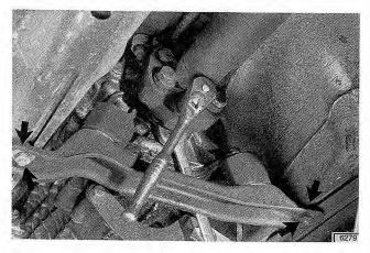
Fig. 6-1. Transmission support (arrows) to be removed.
