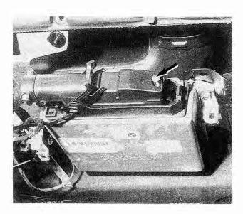
Fig. 6-22. 325i Motronic 1.1 control unit and connector. Retaining screw is shown at arrow. Other Motronic control unit connector is similar.
