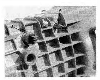
Fig. 7-3. Selector shaft lock pin and spring (A) and back-up light switch (B).
