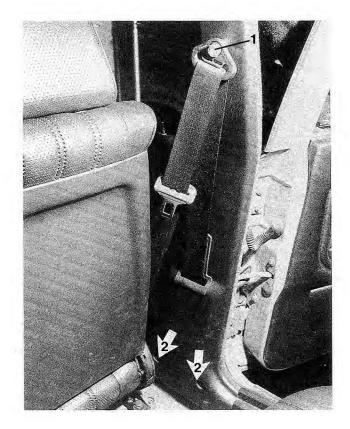
Fig. 4-35. B-pillar trim panel showing upper seat-belt anchor bolt (1) and panel retaining screws (2).
