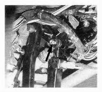
Fig. 5-5. Bolt (arrcw) that connects master cylinder pushrod to clutch pedal.
