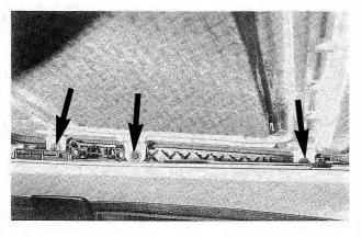
Fig. 7-4. Sunroof left-side mounting screws (arrows). Remove screws from both right and left sides.
