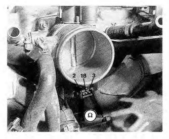
Fig. 6-20. Idle and Full throttle switch showing terminal identification.
