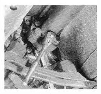
Fig. 4-4. Front driveshaft mounting bolts being removed.
