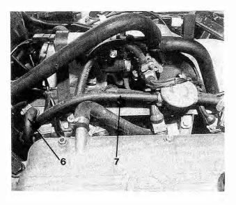
Fig. 4-46. Fuel supply line (6) and fuel return line (7).
