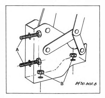
Fig. 8-1. Left-side convertible top mounting bolt (A) and mounting nuts (B). Remove nuts and bolts from both sides of frame.
