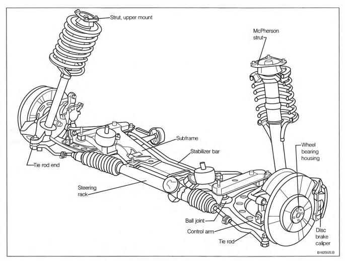
Fig. 1-6. Typical front suspension and steering system.
