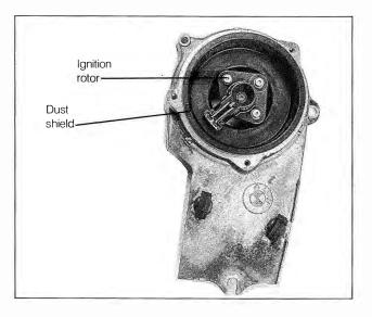
Fig. 3-3. Ignition rotor and dust shield. Front camshaft oil seal is behind dust shield.
