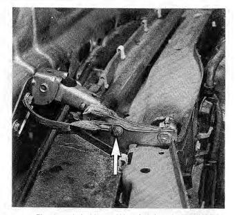
Fig. 6-22. Left-side hood hinge bolt (arrow) to be loosened for front hood height adjustments. Loosen bolts on right side also.
