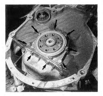
Fig. 6-2. Rear crankshaft oil seal carrier mounting bolts (arrows). Transmission, clutch assembly, and flywheel removed from engine.
