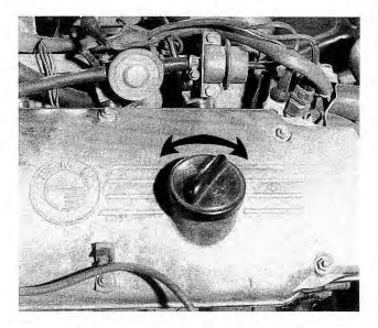
Fig. 4-2. Location of oil filler cap. Remove and install by turning (arrows).
