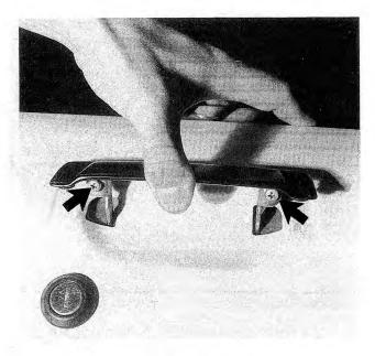
Fig. 5-25. Door handle retaining screws (arrows).
