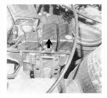
Fig. 4-17. Vacuum advance control relay (arrow). Similar relay in adjacent position with yellow dot on top is for idle speed stabilization (late 1985 models only). Small relay on 1984 and early 1985 models (not shown) is for deceleration fuel shut-off.
