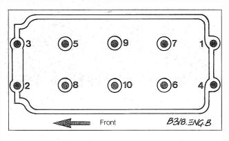
Fig. 4-48. Cylinder head b. <sup>1</sup>oosening sequence for 4-cylinder engine.
