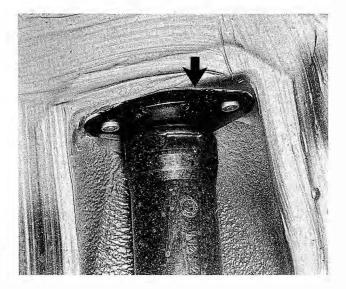
Fig. 6-3. Rear shock absorber upper mounting viewed from below. Notice location of gasket (arrow).
