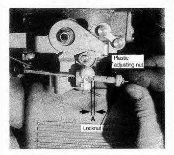
Fig. 4-22. Correct amount of slack in accelerator cable (A) on 6-cylinder engines. Adjust cable by turning plastic adjusting nut. On some models, it is necessary to first loosen a small locknut.
