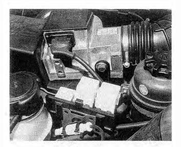
Fig. 4-56. Auxiliary relay panel (arrow) near left (driver's side) shock tower.
