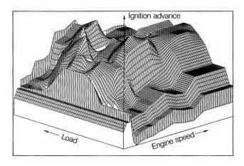
Fig. 5-1. Motronic ignition characteristic map. Courtesy Robert Bosch Corp.
