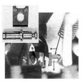
Fig. 4-4. Brake pedal return spring (a), retaining clip (b) and clevis pin (c) as viewed from inside passenger compartment. Inset shows removed clevis pin and clip.
