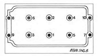
Fig. 4-49. Cylinder head bolt tightening sequence for 4-cylinder engine.
