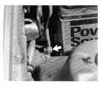
Fig. 3-13. Ground point G100 (arrow) from battery to chassis on all models with battery in engine compartment.
