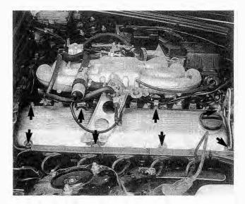
Fig. 4-4. Breather hose and cylinder head cover mounting nuts on 325e engine (arrows).
