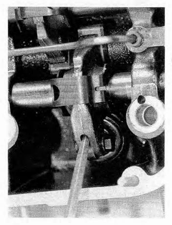
Fig. 4-30. No. 1 intake valve rocker arm being depressed with screwdriver.
