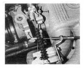
Fig. 4-52. Accelerator cable (1), automatic transmission throttle cable (2), and cruise control cable (3).
