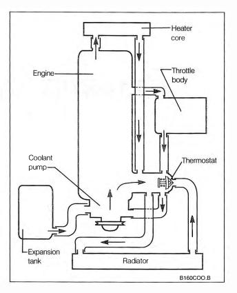
Fig. 1-2. Schematicviewof cooling system components and hose routing showing coolant flow (arrows) for 6-cylinder engine.
