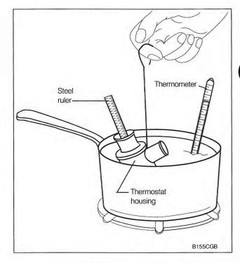
Fig. 4-10. Testing thermostat of 4-cylinder engine in hot water. Change in length is being measured using steel ruler.
