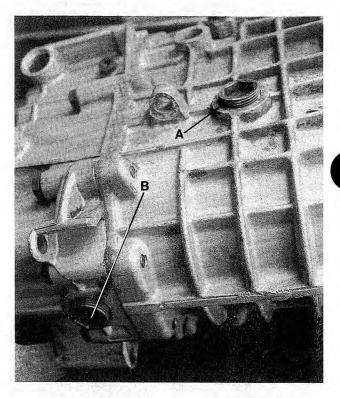
Fig. 7-1. Transmission fill plug (A) and transmission drain plug (B)
