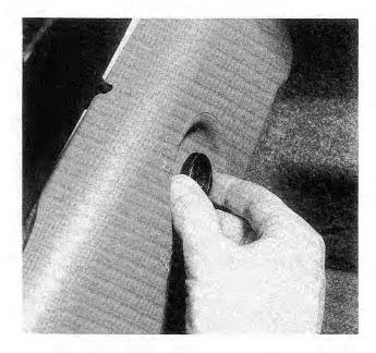
Fig. 6-6. Rear taillight bulb carrier being removed. 1988 and later models shown. On earlier models, there are two locks. Turn counterclockwise to release.
