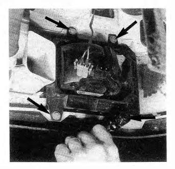
Fig. 6-10. Fog light mounting bolts (arrows).
