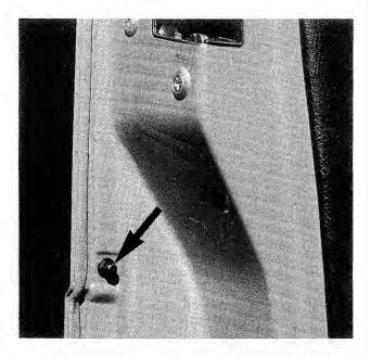
Fig. 6-13. Mounting nut (arrow) for front door body side molding. Nut for rear side panel body molding is similar.
