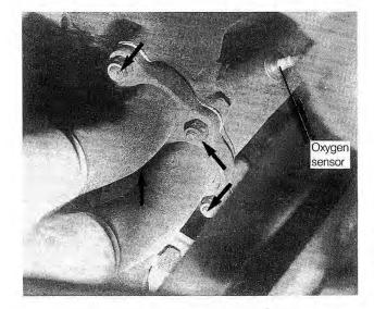
Fig. 4-43. Front pipe to exhaust manifold mounting nuts (arrows) and oxygen sensor.
