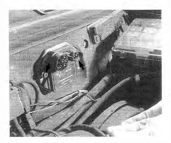
Fig. 4-5. Ignition control unit mounting screws (arrows) on Siemens/Telefunken control unit. Bosch control unit mounting points are similar.
