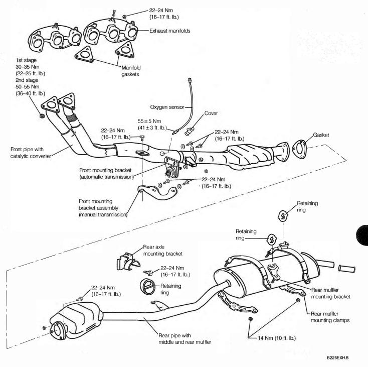
Fig. 4-2. Exploded view of 325 and 325e(es) exhaust system.
