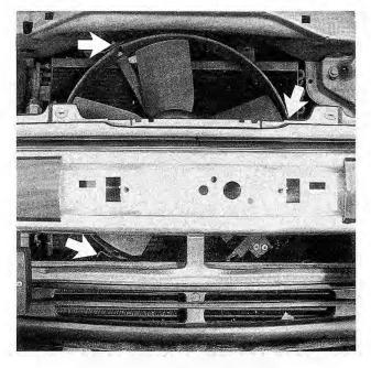
Fig. 4-24. Auxiliary cooling fan mounting nuts (arrows).
