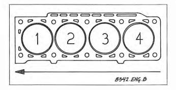
Fig. 6-3. Piston numbering sequence. Arrow points to front (radiator end) of engine.
