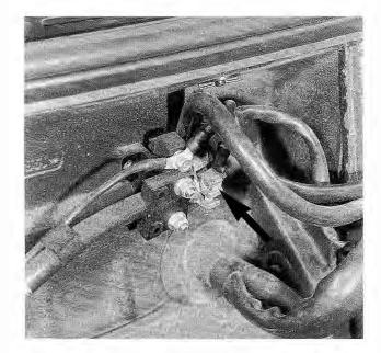
Fig. 6-2. Positive terminal jumper cable connection (arrow) for car with trunk mounted battery.
