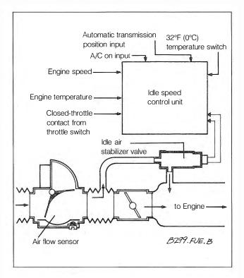
Fig. 6-14. Schematic view of idle air stabilization system installed on 1984 through 1887 325 and 325e models. System on 1988 325 and all 325i models similar, except that Motronic control unit replaces idle speed control unit, and there are additional inputs.
