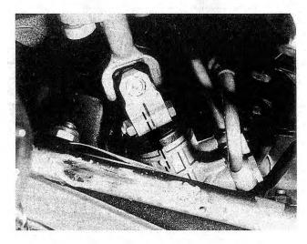
Fig. 4-4. Marks on steering gear housing align as shown when steering gear is centered and front wheels are in straight-ahead position.
