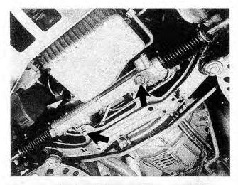
Fig. 7-16. Mounting bolts (arrows) and self-locking nuts mount steering gear to front suspension subframe. Always replace self-locking nuts.
