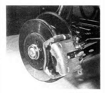
Fig. 5-7. Brake caliper being pivoted into position on pad carrier over brake pads.
