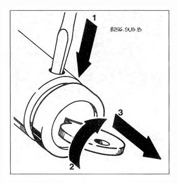
Fig. 7-10. Screwdriver inserted in small hole (arrow) will release ignition/steering lock on older (1984–1986) models. Newer models are similar. See text.
