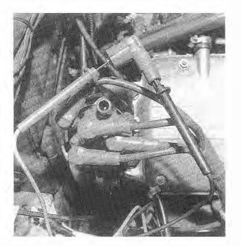
Fig. 3-6. Resistance of spark plug end of wire being measured with an ohmmeter.
