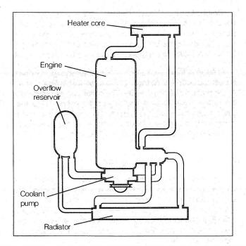
Fig. 1-4. Cooling system. Heat from engine is absorbed by coolant which is circulated by coolant pump and cooled by radiator.
