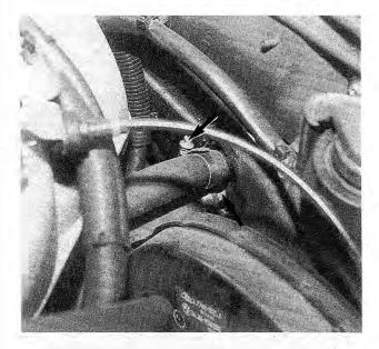
Fig. 4-55. Heater hoses for heater core (arrows).
