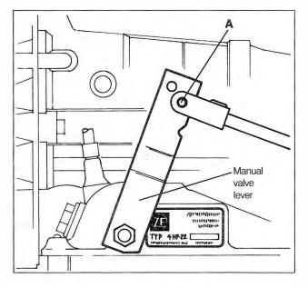
Fig. 4-6. Manual lever for 3 HP 22 transmissions. Selector rod should be installed in hole A.
