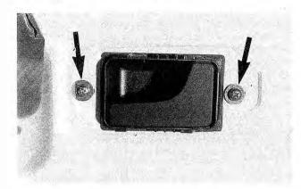
Fig. 5-22. Door operating lever and securing screws (arrows).
