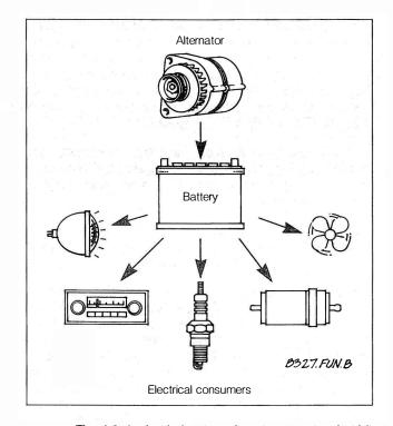
Fig. 1-9. In electrical system, alternator generates electricity to recharge battery and power other electrical consumers.
