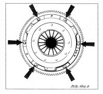
Fig. 5-9. Pressure plate bolts (arrows) to be removed for clutch removal.
