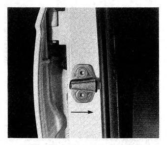
Fig. 5-5. Door striker plate. Loosen bolts and move in or out to adjust closed position of door (arrow).
