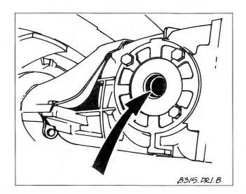
Fig. 5-7. Drive flange snap ring (arrow) to be removed from differential housing.
