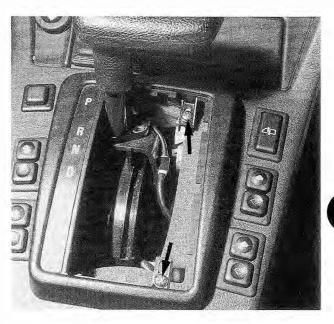
Fig. 4-4. Console trim mounting screws (arrows).
