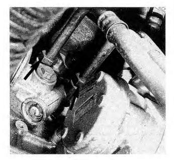
Fig. 7-9. Oil cooler fitting on oil filter housing (arrows).
