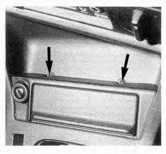
Fig. 4-8. Ashtray console retaining screws (arrows).
