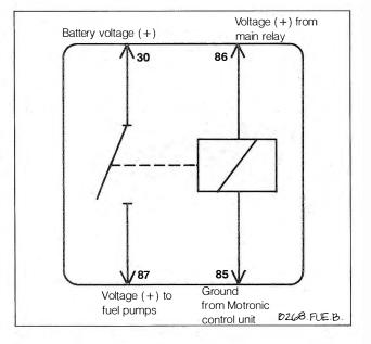
Fig. 4-11. Schematic view of fuel pump relay and circuits installed on models with 6-cylinder engine.
