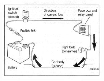
Fig. 3-3. Schematic representation of simple circuit for light bulb. Switch is shown closed, making circuit complete.
