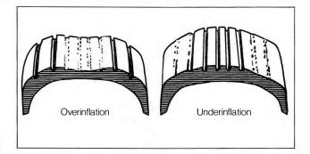
Fig. 3-3. Examples of uneven tread wear caused by overinflated and underinflated tires. Drawings courtesy of Goodyear Tire and Rubber Co.
