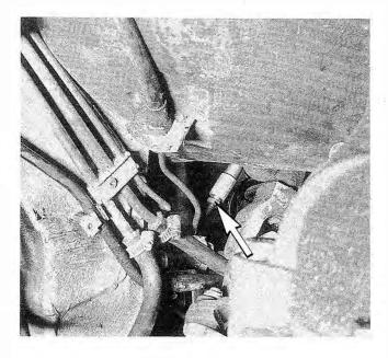
Fig. 5-4. Clutch hydraulic hose connection (arrow) to master cylinder.
