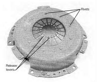
Fig. 5-11. Clutch pressure plate rivets and release lever tips to be checked.
