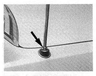
Fig. 4-15. Antenna mast clamping nut (arrow).
