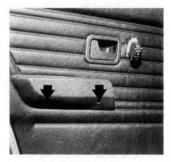
Fig. 5-11. Rear door trim panel securing screws (arrows). Armrest remains secured to panel after screws are removed.
