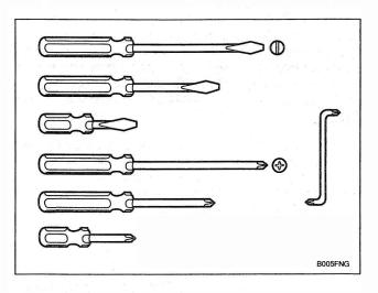
Fig. 4-1. Common flat-blade (top) and Phillips (bottom) screwdrivers. Offset screwdriver (right) is used for screws with limited access.
