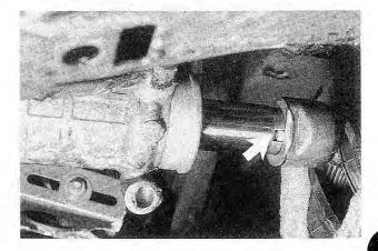
Fig. 7-13. Inner tie rod end ball joint and lockplate. Tab on lockplate (arrow) fits into notch on steering gear housing. (Shown with protective boot pulled back),
