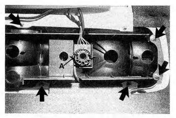
Fig. 6-7. Retaining nuts (arrows) for taillight lens. Remove harness connector (A) before removing lens. On some models, connector may be to side of lens.
