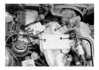
Fig. 4-45. Air flow sensor connector (1), air filter housing mounting bolts (2), brake vacuum booster hose (3), idle air bypass hose (4), and diagnostic plug (5).
