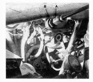
Fig. 4-23. Accelerator cable adjusting nut (A) on 4-cylinder engines. To adjust, hold guide nut (B) and turn adjusting nut.
