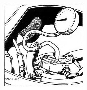
Fig. 4-5. Transfer pump fuel pressure being measured with fuel pressure gauge.
