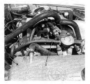
Fig. 5-8. Fuel supply line (i), fuel return line (j), and supply line bracket (k).
