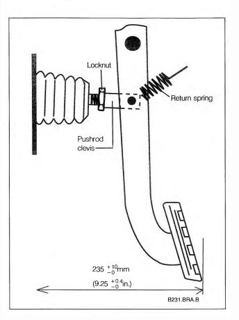
Fig. 4-8. Schematic drawing of brake pedal assembly showing brake pedal freeplay measurement.
