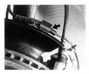
Fig. 5-2. Brake pad wear sensor connector on front left wheel (arrow).
