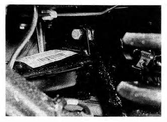
Fig. 6-15. Inner rear suspension trailing arm mount on top of rear axle carrier.
