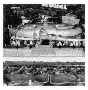
Fig. 4-29. Fuel rail mounting bolts on 6-cylinder engines (arrows).
