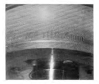
Fig. 7-9. Rear rotor minimum dimension stamped on rotor hub.
