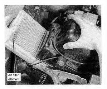
**Fig. 5-2.** Air filter being removed from air filter housing. Air filter housing will vary slightly between models.
