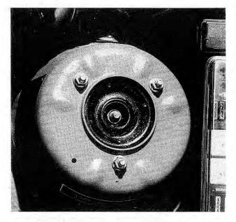
Fig. 4-7. Three mounting points of upper strut mount. Available replacement mount moves strut off-center to alter front wheel camber.
