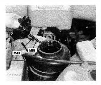
Fig. 6-7. Power steering fluid dipstick showing MIN and MAX marks.
