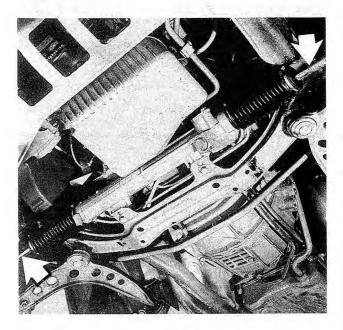
Fig. 7-1. Rack and pinion steering gear, operated by steering wheel, is connected to wheels by tie rods (arrows).
