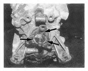
Fig. 7-44. Lockplate tabs (arrows). Bend tabs out of groove to remove lockplate and collar nut.
