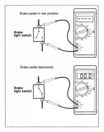
Fig. 3-3. Brake light switch being tested for continuity. With brake pedal in rest position (switch open) there is no continuity (infinite ohms). With the pedal depressed (switch closed) there is continuity (zero ohms)
