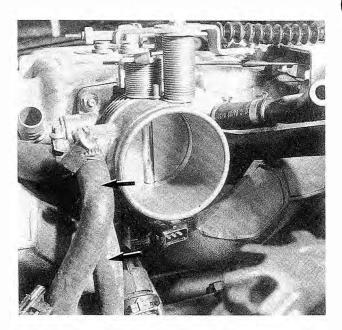
Fig. 6-8. Coolant hoses to be removed from throttle housing (arrows).
