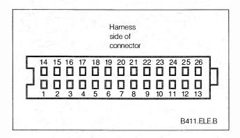
Fig. 7-1. Terminal identification for 26-point instrument cluster connectors. There are three 26-point connectors attached to the rear of the cluster. Use care not to damage connector terminals with test probes.
