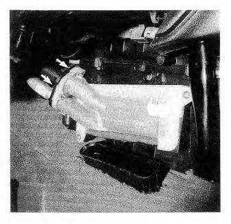
Fig. 4-23. Heater core flange bolts (arrows) between heater valve and heater core.
