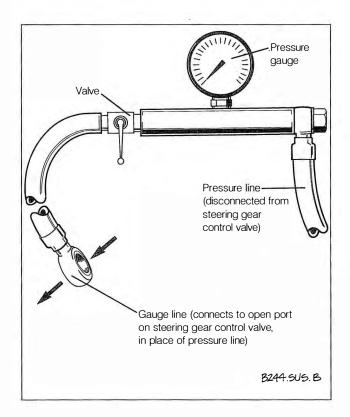
Fig. 7-17. Pressure gauge set-up for measuring power steering pump pressure. Disconnect original pressure line from steering gear and connect to gauge as shown. Connect gauge line to open pressure line connection on steering gear.
