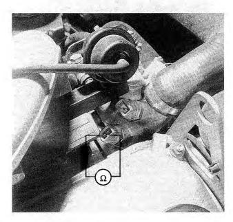
Fig. 6-13. Schematic view of ohmmeter test leads connected across coolant temperature sensor terminals.
