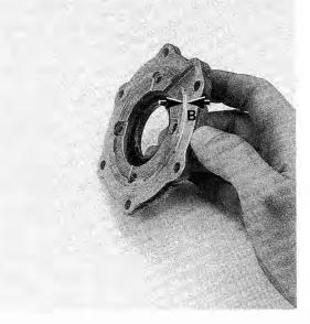
Fig. 7-27. Clutch guide sleeve protrusion height (dimension B).
