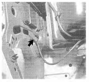
Fig. 4-18. Intake air temperature sensor mounted in air duct (arrow).
