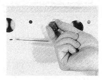
Fig. 6-25. Trunk lid stop being adjusted. Screw stops all the way in on both sides before making any adjustments to trunk lid.
