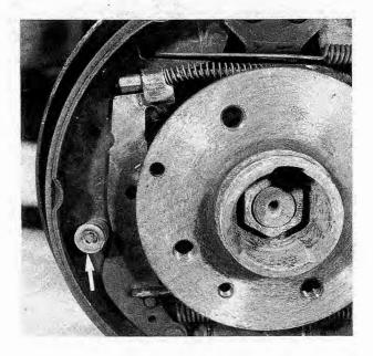
Fig. 6-4. Rear brake assembly brake shoe retaining pin and spring retainer (arrow).
