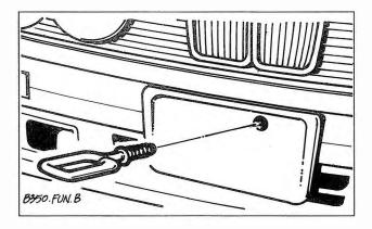
Fig. 6-4. Screw-on type front towing eye.
