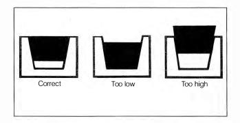
Fig. 6-3. Cross-section of correct V-belt position in pulley.
