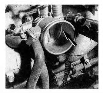
Fig. 6-4. Throttle plate clearance between housing and plate (arrow) on 325i model. 325e model is similar. Throttle plate should not contact housing.
