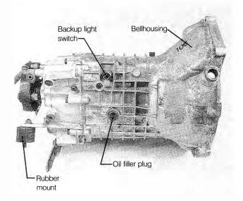
Fig. 1-1. Transmission case of five-speed Getrag 240 manual transmission.
