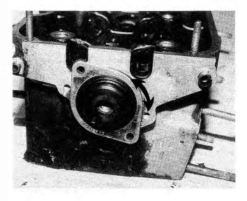
Fig. 4-33. Camshaft oil seal housing being removed from cylinder head. Rotate housing back and forth as it is removed (arrow).
