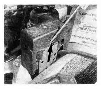
Fig. 14-2. Auxiliary relay panel protective cover being removed. Depress the catch (arrow) and lift off cover.
