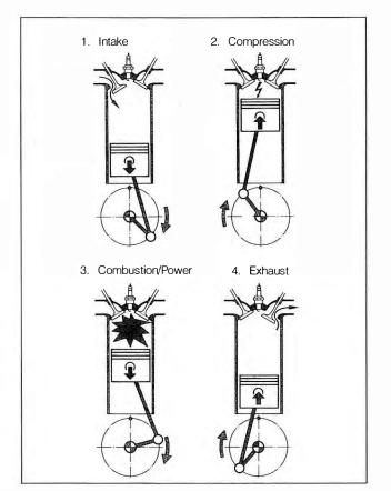
Fig. 1-2. The four-stroke cycle.
