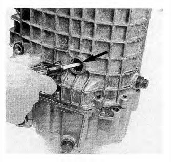
Fig. 7-23. Screwdriver being used to guide layshaft into bearing shell (arrow) as front case is installed.
