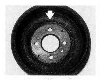
Fig. 6-10. Rear brake drum showing location of stamped drum diameter specifications (arrow). Check diameter of drum at several points.
