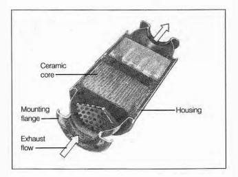
Fig. 4-7. Cutaway view of catalytic converter.
