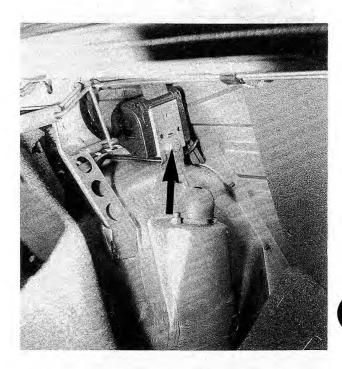
Fig. 4-38. Rear seat belt retractor mounting in trunk (arrow) for models up to 1986.
