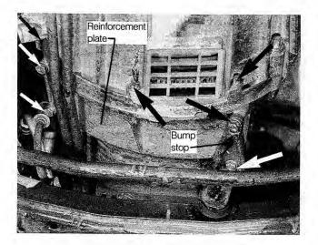
Fig. 5-2. Transmission reinforcement plate and bump stop, showing bolts to be removed (arrows).
