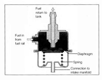
Fig. 4-19. Schematic view of fuel pressure regulator. Fuel pressure deflects diaphragm to return fuel to tank. Amount of fuel return determines pressure.
