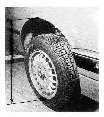
Fig. 5-9. Ride height measurement is taken from bottom of wheel arch to edge of wheel rim. (Measure with car on ground and loaded. See text.)
