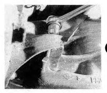
Fig. 5-3. Final drive front mounting bolt being removed. Also remove front bolt from other side.
