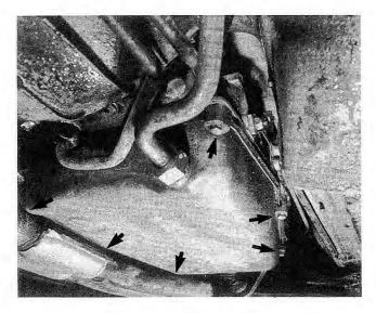
Fig. 7-10. Automatic transmission sump mounting bolts and clamping brackets (arrows).
