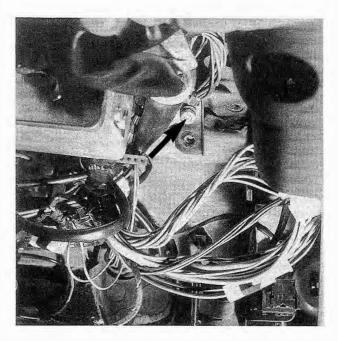
Fig. 3-9. Ground point G200 (above brake pedal) for ignition switch, on-board computer, and start relay (arrow).
