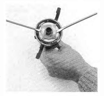
Fig. 4-10. Trigger wheel being removed from distributor shaft. Pry evenly under center of trigger wheel, from both sides using flat-blade screwdrivers.
