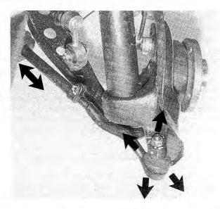
Fig. 7-12. Inspecting tie rods. There should be no noticeable play (arrows) between mating parts.
