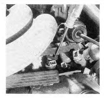
Fig. 4-30. Fuel injector mounting clip being removed.
