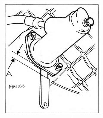
Fig. 7-5. Clutch disc being checked for wear using special tool. If gap of more than 5 mm (0.2 in.) exists (dimension A), the clutch disc is excessively worn and should be replaced.
