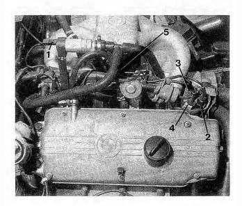
Fig. 4-44. Harness connectors that need to be disconnected. Idle air stabilizer valve connector (1), thermo-time switch (2), coolant temperature sender (3), engine temperature sensor (4), and cold-start valve (5).
