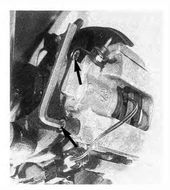
Fig. 7-3. Upper and lower caliper guide bolts (arrows) being removed.
