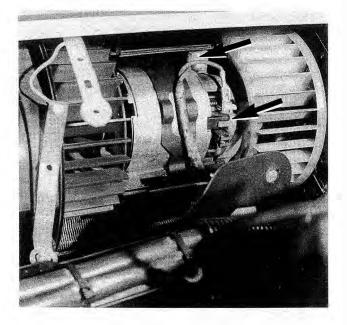
Fig. 4-32. Blower motor wires (arrows) to be removed.
