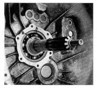
Fig. 7-25. Input shaft circlip (A) and spacer (B).
