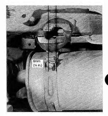
Fig. 4-4. Rear muffler retaining ring preload. Preload shown has been exaggerated for clarity.
