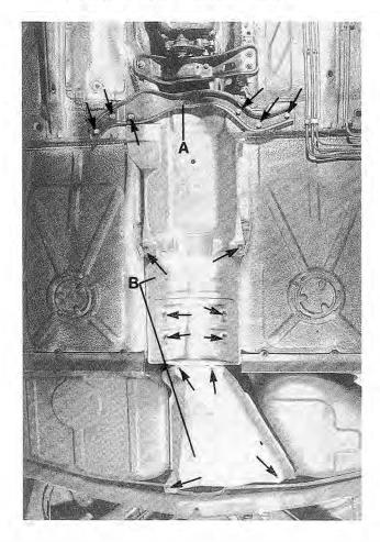
Fig. 4-2. Rear reinforcement bar (A) and heat shields (B) to be removed after removing bolts (arrows).
