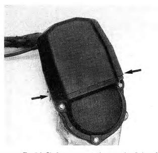
Fig. 5-9. Distributor cap protective cover installed on 6cylinder engines. Unclip cap at points indicated by arrows.
