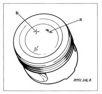
Fig. 6-4. Piston crown identification markings. Arrow should face front. Nominal piston diameter shown at **a**, and weight classification at **b**.
