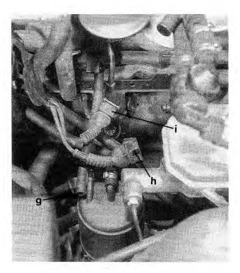
Fig. 5-21. Charcoal canister vacuum hose (g), and throttle switch harness connector (h) disconnected. Purge valve harness connector installed on models with Motronic 1.1 shown at (i).
