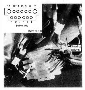
Fig. 10-13. Harness connector (C202) for headlight dimmer switch (arrow). Lower steering column trim panel removed. Inset identifies connector terminals.
