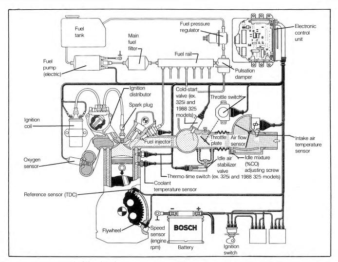
Fig. 1-2. Schematic of Motronic engine management system used on all 6-cylinder engines covered in this manual. Courtesy Robert Bosch Corp.
