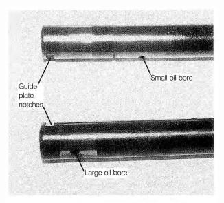
Fig. 4-41. Rocker arm shafts showing notches for front guide plate and oil bores.
