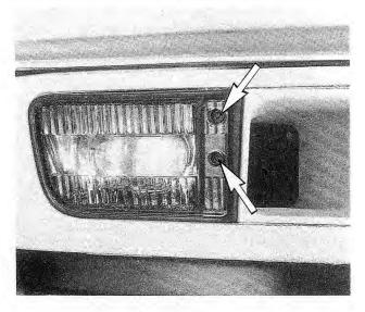
Fig. 6-11. Fog light adjusting screws (arrows).
