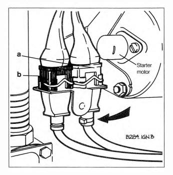
Fig. 5-5. Gray reference sensor connector (a) and black speed sensor connector (b) for 1986 and 1987 325e(es) engine. Reference sensor also marked with a ring (arrow).
