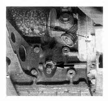
Fig. 7-1. Oil pressure switch on 6-cylinder engine (arrow).
